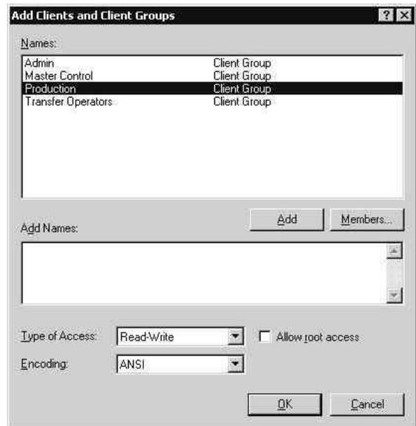
In the screen above, it is also possible to type the IP address of an individual DigiCart/E in the Add Names field and click OK. This is useful when setting up personal drives that are to be accessed by only one or a few units and you don't want to define a group for them.
