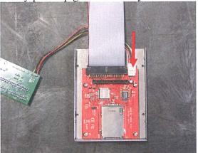
4.4.3. Verify middle connector of 40 pin ribbon cable is connected to card reader.
