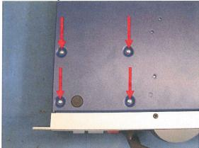
4.1.7. Remove the drive assembly from the unit.
