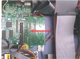
4.2.10. Connect Molex power cable to relay board.
