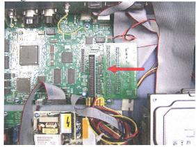
4.4.11. Plug the DC power cable into the hard drive.
