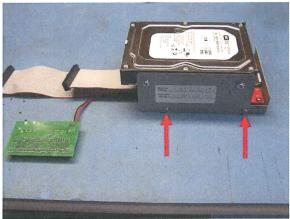
4.4.5. Connect 40 pin ribbon cable to hard drive.
