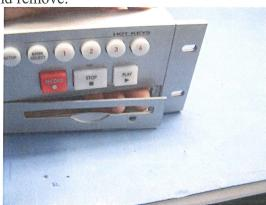
4.1.12. Using a fingernail or flat blade screwdriver as a scraper, remove any adhesive residue from the front panel.
