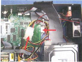
4.4.13. Plug the 40 pin ribbon cable into the DCE mainboard.
