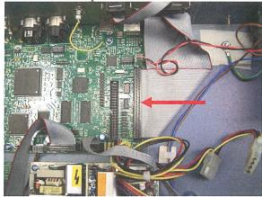
4.2.6. Fold 50 pin ribbon cable away from the DCE mainboard.
