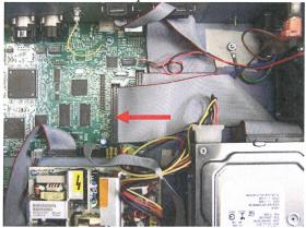
4.1.5. Disconnect the power cable from the hard drive and Zip drive.
