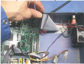
4.2.7. Set card reader/relay board assembly (without the hard drive) inside unit.
