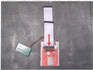
4.2.4. Insert SD card containing DCE software into card reader.
