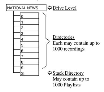
Each drive has 11 directories (numbered 0 through 9, plus "S"). Drives and Directories can be labeled for convenience. Each directory contains 1,000 Index numbers for audio files, called "Cuts". Cuts can be of any length, but are identified by this fixed Indexing scheme. Directory S is reserved for up to 1,000 Playlists (or Stack files). Playlists are not audio files, but merely listings of file IDs. Audio files cannot be stored in the Stack Directory.
