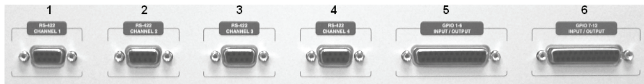
Figure 38 - Rear Panel Detail of Serial Port Connectors
