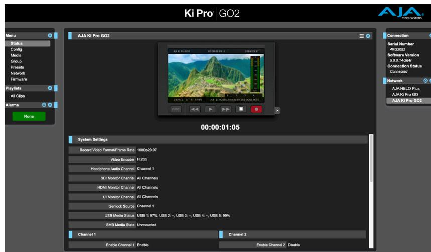
The Status screen displays the current configuration state of the Ki Pro GO2. When an SMB volume is mounted, its status is displayed along with additional SMB parameter information. When Unmounted, these parameters are hidden on this screen.
