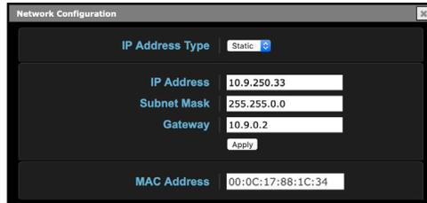
**NOTE:** LANs may be divided into zones, and devices on a LAN may have dynamically assigned (DHCP) IP addresses, or fixed (static) IP addresses. Before connecting Ki Pro GO2 to the LAN, talk to your network administrators to find out how they want it connected (DHCP or Static IP).
