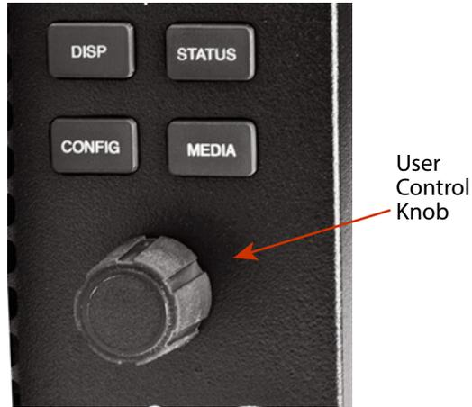
When an active configuration menu is displayed, pressing and holding the knob will restore that menu's factory default setting.
