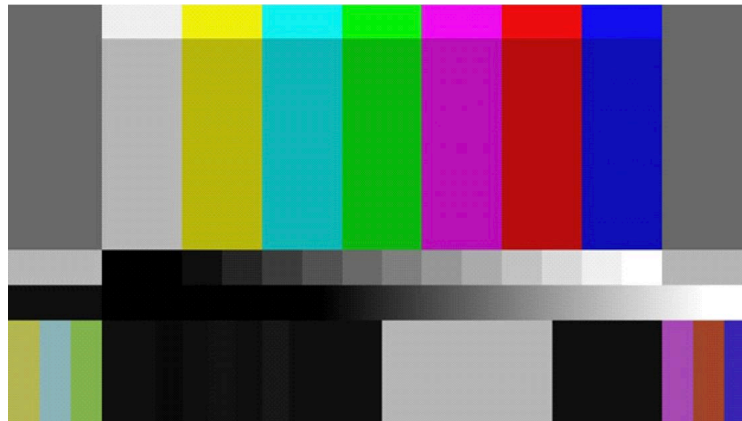
Figure 34. BT.2111 High Dynamic Range Color Bars Example
