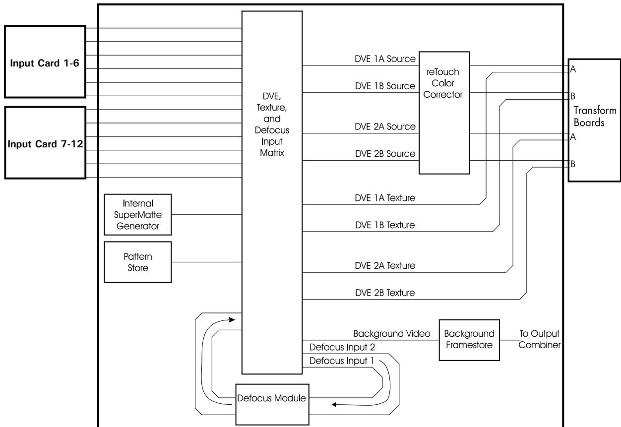
The twelve video signals, the SuperMatte generator, the Pattern Framestore, and the Defocus outputs are all available as DVE/texture matrix outputs. The nine matrix outputs feed two video/key sources (A and B) and two texture sources (A
