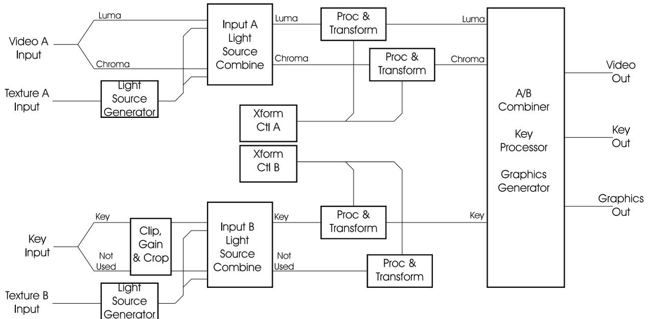
**Video-Key+Shadow Mode** The Video+Key+Shadow mode is similar to the Video+Key mode, except the “chroma” part of the B circuitry is used to process a full bandwidth shadow signal.
