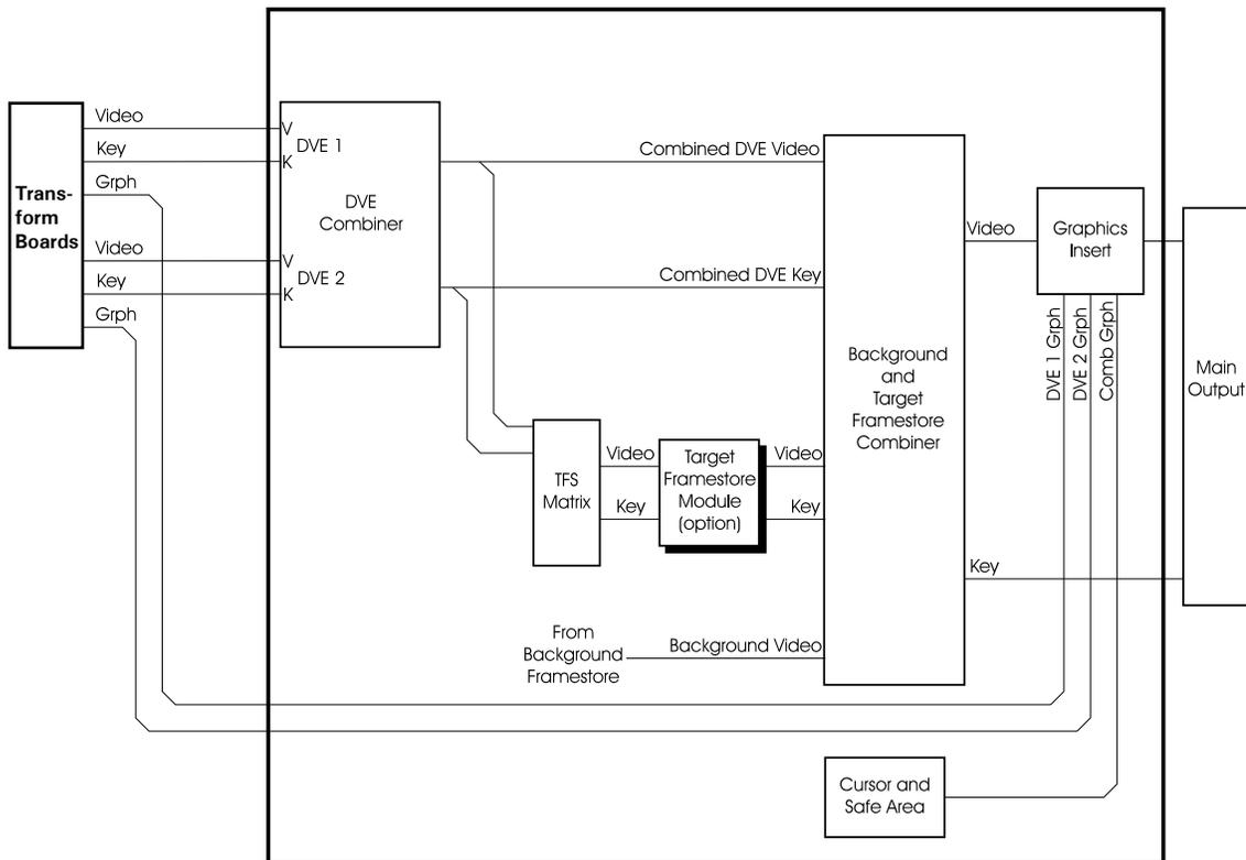
The DVE Combiner combines the two DVEs' video and key signals into a single set of video and key signals.
