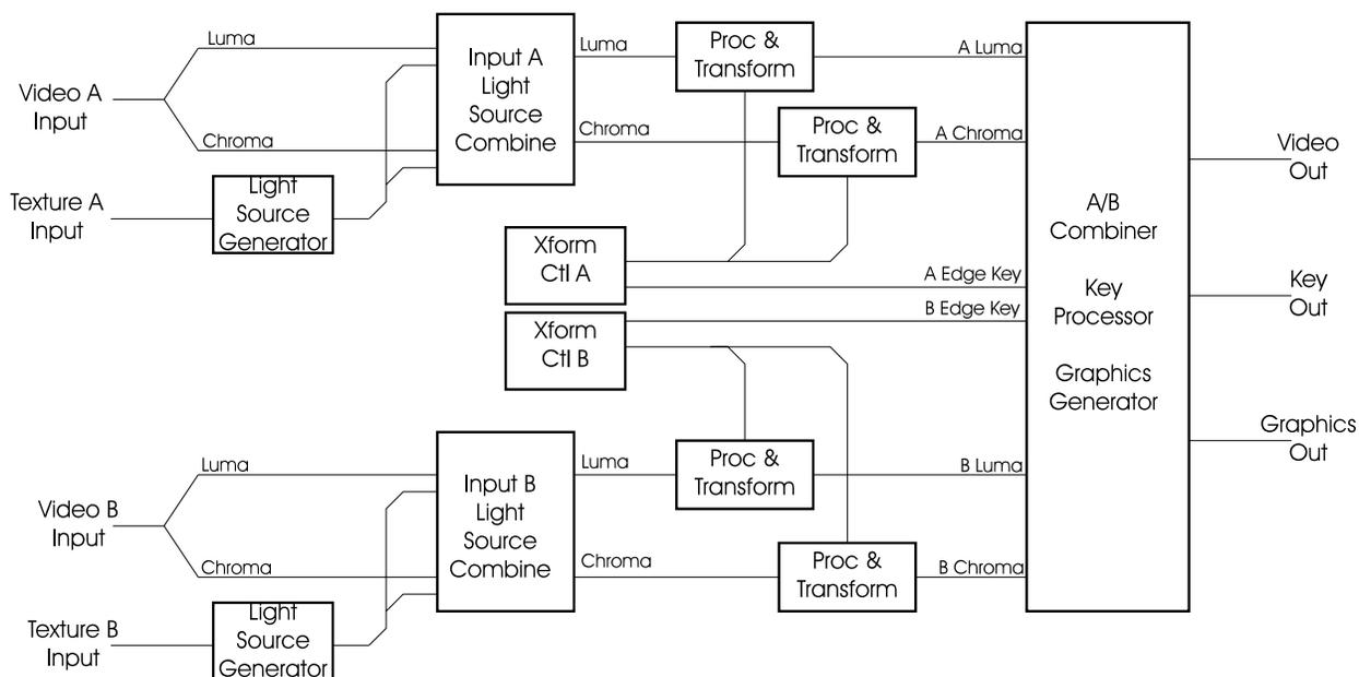
**Video+Key Mode** The Video+Key mode differs from the Video+Video mode only in that the board processes the B input as the key signal, with additional clip, gain and H phase adjustments. Note that the "chroma" part of the B circuitry is not used since key signals are monochrome.
