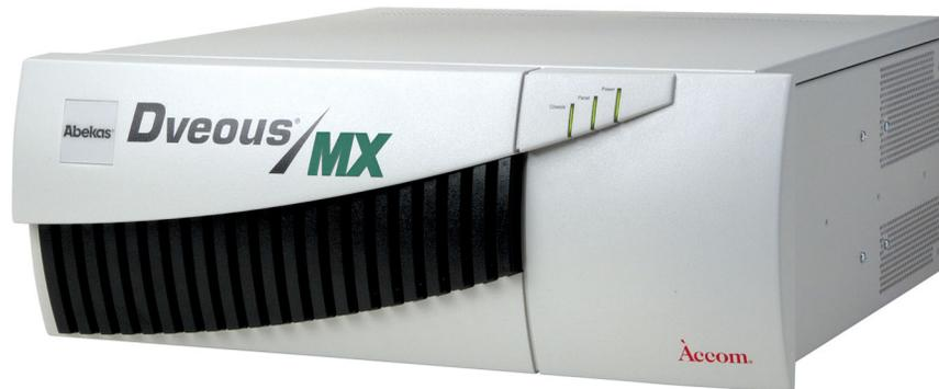
The Dveous/MX front bezel can be removed by grasping and firmly pulling forward. However, there is no need to remove this bezel unless the chassis will be rack mounted.
