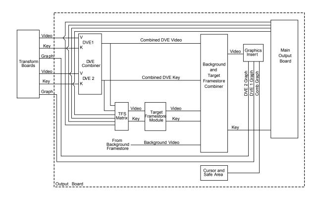
The DVE Combiner combines the two DVEs' video and key signals into a single set of video and key signals.
