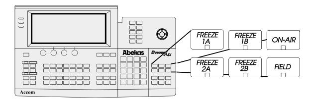
Note: On-air freezes override any timeline effect freeze: the channel input stays frozen no matter what effects you recall or run. This on-air freeze is different from the freeze setting in the Input menu, which lets you apply a freeze on a keyframe-by-keyframe basis.
