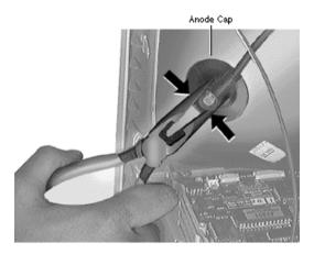
1. Using needlenose pliers, compress the anode cap to free it from the anode aperture.
