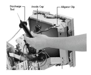
If you are working on a stand-alone monitor, attach the clip of the CRT discharge tool to the monitor chassis.
