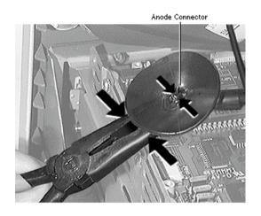
**Replacement Note:** To replace the anode cap, use needlenose pliers to press together the plastic cup outside of the anode connector so that you can insert it into the anode aperture. Tug on the high voltage cable to make sure it is firmly seated. Then press down around the edges of the rubber anode cap to ensure a firm seal.
