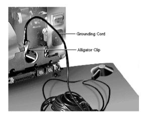
Or, if you have a grounding cord with alligator clips, attach the clip to any metal part of the device you are working on.
