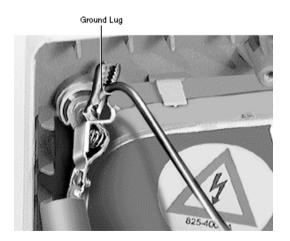
**Caution:** If you are working on a compact Macintosh that contains a CRT and incorrectly discharge the CRT to the metal chassis, you may destroy the logic board. You must discharge to the ground lug!
