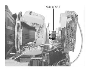
**Warning:** Do not pick up or handle a CRT by its neck, where the tube is the thinnest. To prevent an implosion, take every precaution against breaking the CRT.
