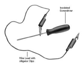
If you do not have a discharge tool, you can use an insulated screwdriver attached to a wire lead with alligator clips on both ends as shown here. You should also use this discharge method as a follow-up after using the older Apple CRT discharge tool to ensure that the CRT is discharged.
