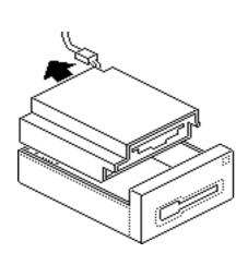
2 Lift the back of the metal drive housing—being sure to support the cable connector—and remove the drive from the bottom cover.
