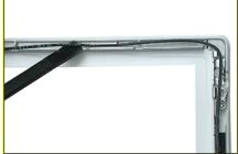
4. Free the microphone cable from the right corner of the bezel and from underneath the tape at the antenna board.
