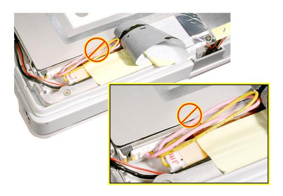
With the shield installed over the replacement LCD panel, apply a rectangular piece of foil tape to overlap the shield and cables at the left side of the clutch, as shown below.
