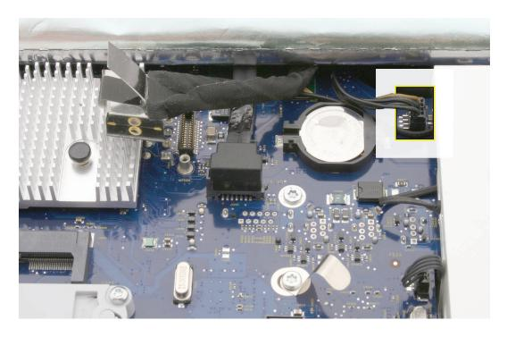
4. Using the access card or a black stick, peel the EMI tape away from each side of the panel. Remove the four panel mounting screws with a T10 screwdriver.
