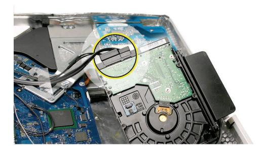
**5. Transfer the temperature sensor from the bad drive to the replacement hard drive.** Note: If you are replacing a hard drive, also remove the mounting bracket and the mounting pins shown in the following steps.
