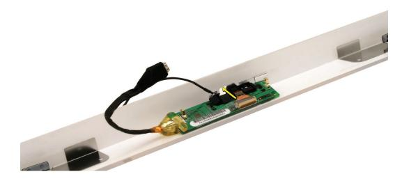
2. Install the camera board to the bezel with two T6 mounting screws.
