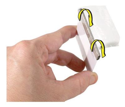
4. Bend the card at a slight angle at the top to make sure the card makes contact with each latch.
