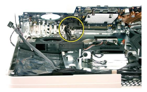
2. Check that the screw holes are aligned with the screw mounts in the chassis. **Replacement Note:** The logic board should rest on the screw mounts without any binding or bowing—if it doesn't, adjust any cables that are interfering with the logic board. Reconnect the ten logic board cables.
