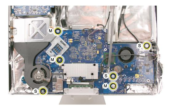
3. Rotate the unit so the top of the rear housing is facing you. With a black stick, disconnect the power supply cable on the underside of the logic board.
