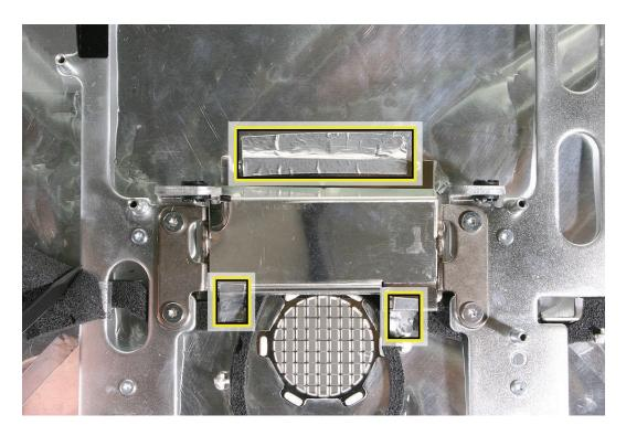
2. Remove the metal clutch cover.
