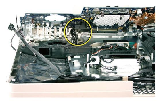
4. Pull the board toward you and gently lift the board up. **Note**: The I/O ports fit tightly into the port hole openings on the rear cover. You may have to wiggle with the board to free the ports from the rear cover.
