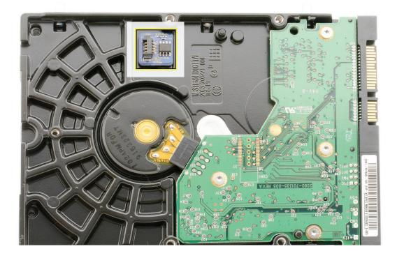
6. Using a T8 torx screwdriver, remove two screws and the mounting bracket from the drive.
