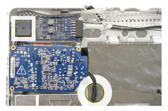
2. Using a T10 screwdriver, remove the three self-tapping screws (top right and the two on the left side) and the one machine screw on the lower right corner of the board.
