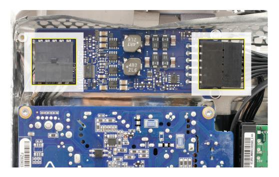
2. Using a T10 torx screwdriver, remove the two self-tapping screw from the bottom corners of the board and the machine screw in the top right corner.
