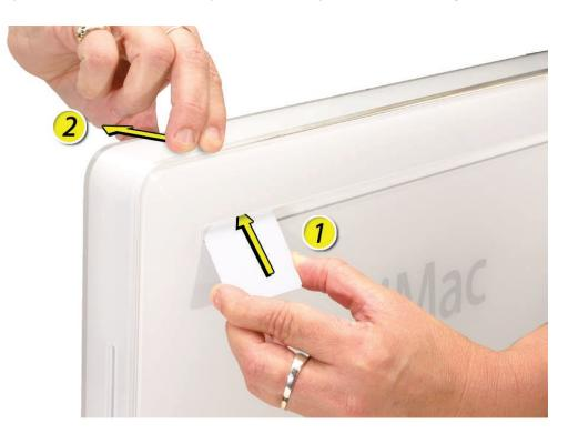
6. Repeat step 5 to release the locking latch in the right corner. Again, pull the bezel away as the card releases the latch.
