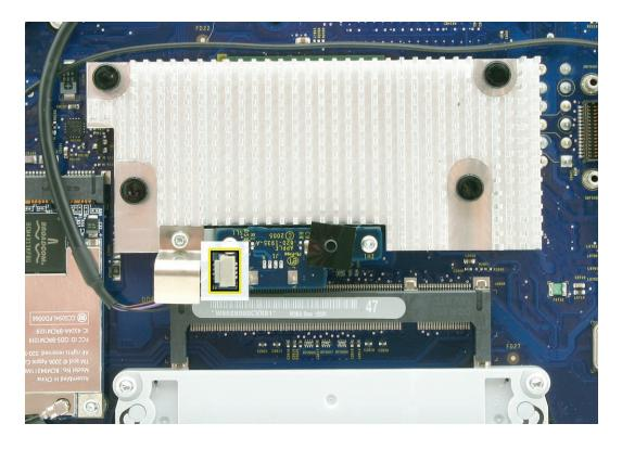
2. Using a Torx T6 screwdriver, remove the two IR screws. Lift the IR board from its mounting bracket.
