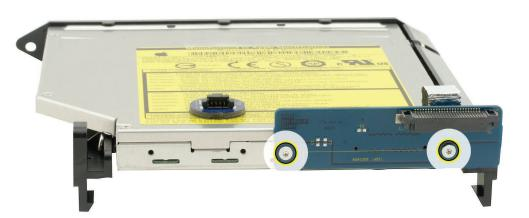
7. If replacing a bad optical drive the replacement drive comes with a new sensor already installed.
