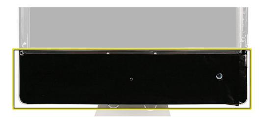
When properly repaired, all edges shown below will be wrapped by EMI tape, and the tape securely adhered to all edges. Use a black stick to flatten the EMI tape tightly and rub out air pockets and wrinkles.
