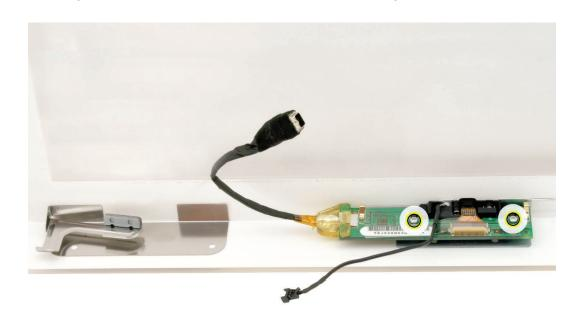
3. Using a T6 screwdriver, remove the two camera board mounting screws.
