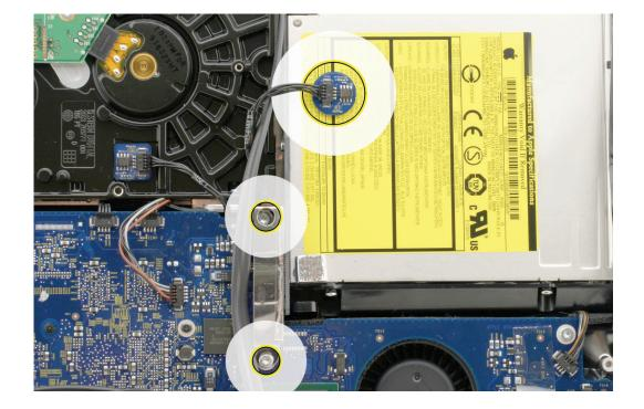
2. Locate the black tabs at each side of the plastic optical drive mounting bracket. Using a flatblade screwdriver, press down and then out on the mounting bracket to the release tab, from the chassis. Repeat process to unhook the other release tab from the chassis.
