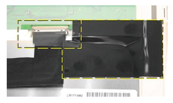
2. Pinch together the connector locking levers, and disconnect the LVDS cable connector.
