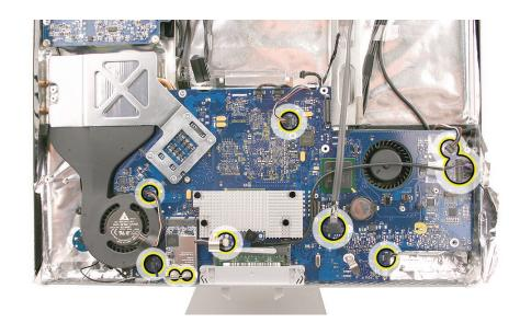
2. Using a T10 torx screwdriver, remove the screws from the logic board. The locations of the three self-tapping screws are marked by and "S" in the photo. The remaining three screws, are machine screws; they are marked with an "M". **Note**: Transfer the small metal grounding (located two screws below the battery) clip to the replacement logic board.
