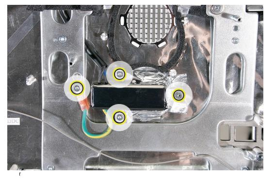
3. Peel the EMI tape off the power inlet.
