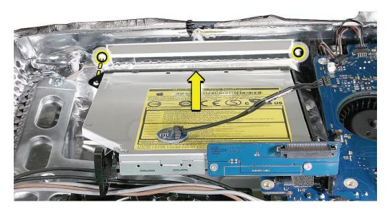
Push down on the black mounting bracket to lock the optical drive securely into place on the chassis.
