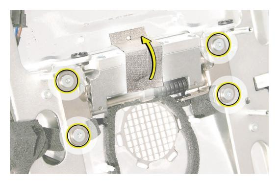
4. Stand up the unit and remove the four clutch-to-stand mounting screws. Separate the clutch from the rear housing and the stand.
