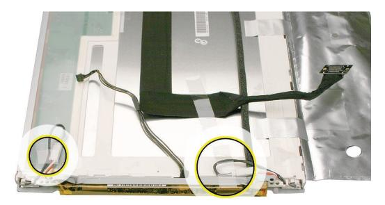
8. Peel back the clear tape and disconnect the two inverter-to-display cable connectors.
