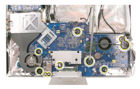
3. Secure the logic board by installing the machine screws first and then the self-tapping screws, marked with an "S".
