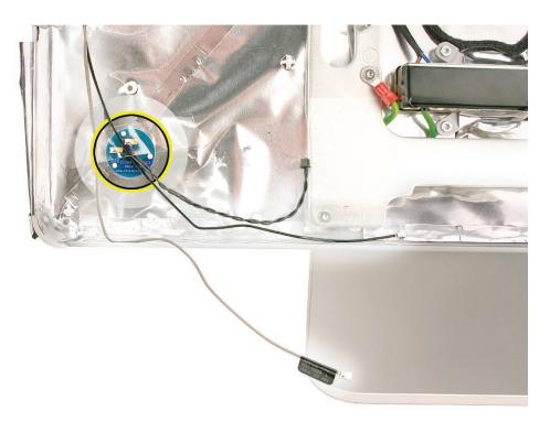
4. Pull the antenna cables through the access hole in the EMI shield at the top, near the antenna board.
