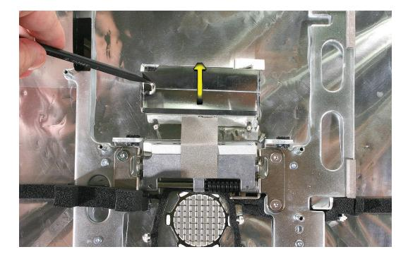
3. Using a T10 torx screwdriver, remove the four clutch mounting screws. Peel the EMI tape up to access the stand screws.
