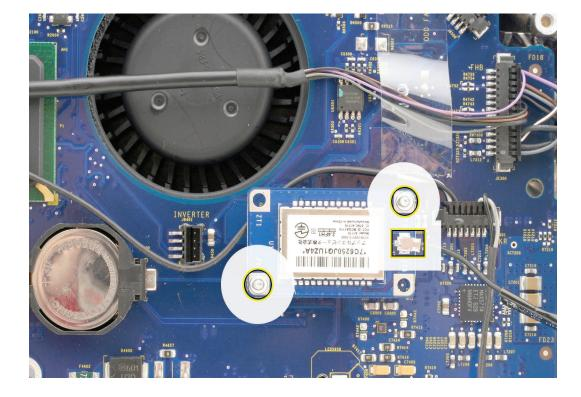
2. Lift the Bluetooth card straight up and off the logic board connector.
