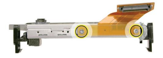
5. If replacing a bad optical drive, remove the temperature sensor from the top of the drive. Discard the sensor—the replacement drive comes with a new sensor already installed.
