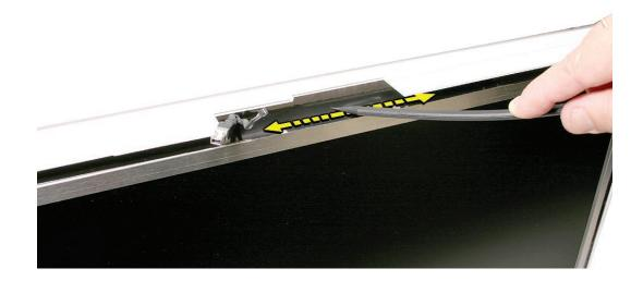
3. Tuck the cables neatly into the channel on the rear housing.
