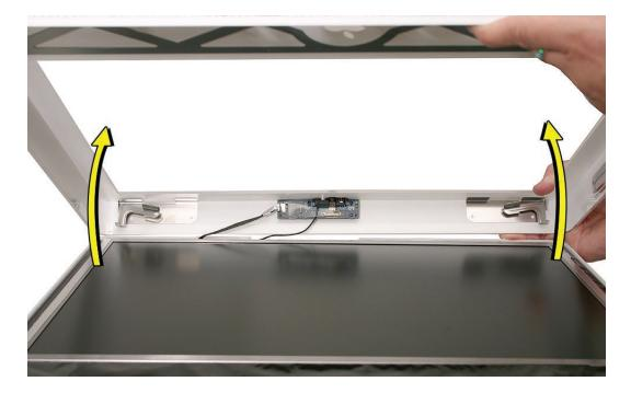
11. Swing the bezel up so you can disconnect the two camera board cables Remove the any kapton tape and disconnect the camera and microphone cables from the camera board.
