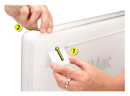
6. Repeat step 5 to release the locking latch in the right corner. Again, pull the bezel away as the card releases the latch.
