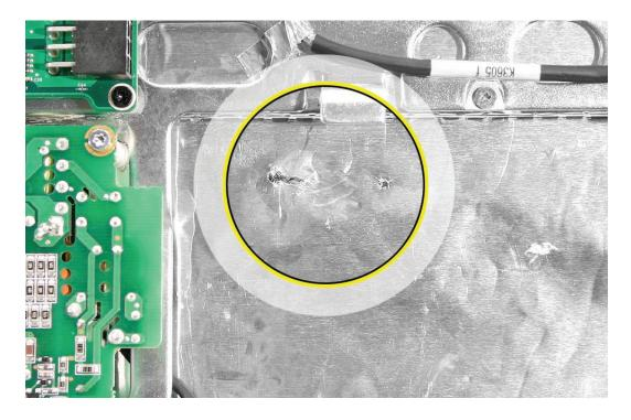
Pay particular attention to the EMI shielding inside the rear housing, shown below. The EMI shield is easily damaged when replacing the hard drive.
