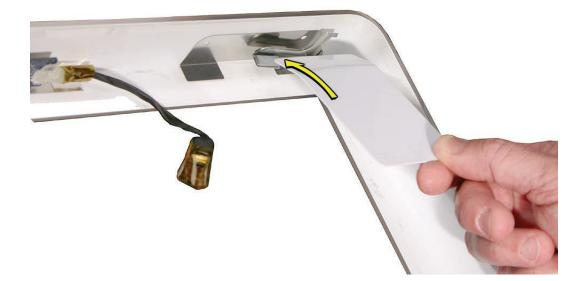
5. Start on the left side (looking from the back of the unit). As you insert the card to disengage the latch, squeeze the top of the bezel, that will help take pressure off of the latch and enable it to open easier. As the bezel releases, pull the bezel away from the rear housing. Note: If the bezel won't open, try cutting the card lengthwise into 3/4 inch or 1.5 cm strips. Insert the card again, on a 45° angle, aimed toward the outer corner, and try again.
