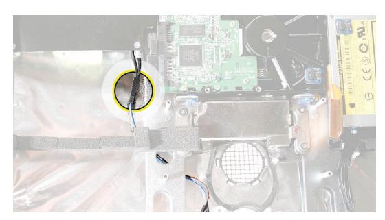
4. .Disconnect the power inlet-to-power supply cables and unlace the power inlet cable from beneath the chassis.
