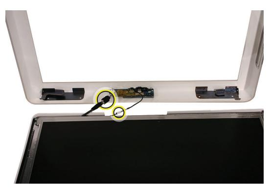
12. If replacing a damaged front bezel, remove the camera board.
