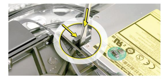
**Caution:** Never press down on or grasp the body (silver) of the optical drive when removing or installing it. Depressing the body of the optical drive could damage the mechanism. Grasp the optical drive by its mounting bracket only.
