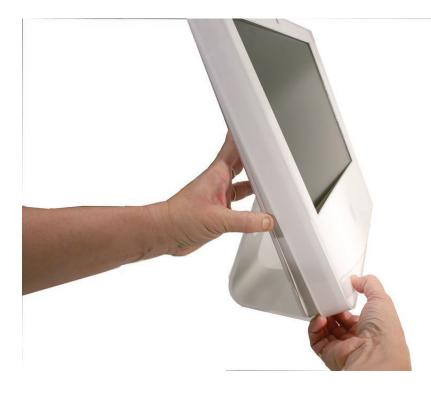
9. Once the access card has been removed, it is safe to open the bezel. Position the unit on an ESD mat, with the bottom facing toward you. **Caution**: Make sure the memory levers are closed and not protruding from the bezel when removing the bezel.
