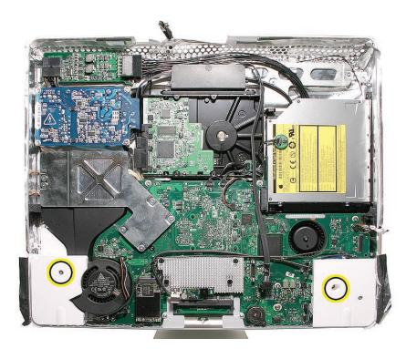
2. Lift the speakers straight up and disconnect the speaker cable under the right speaker.
