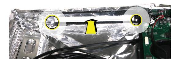
3. Push down on the mounting bracket to lock the optical drive securely into place on the chassis.
