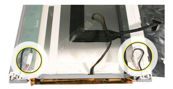
2. Using a flat-blade screwdriver as shown, pry up the inverter to remove it from inside the display panel mounting bracket.
