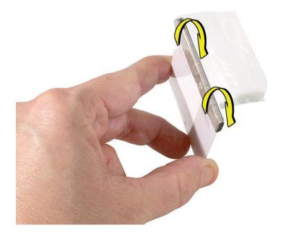
4. Bend the card at a slight angle at the top to make sure the card makes contact with each latch.
