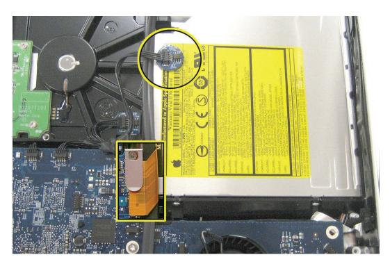
2. Locate the black tabs at each side of the plastic optical drive mounting bracket. Using a flatblade screwdriver as shown, press down on the mounting bracket at the base of the release tab, while pushing the release tab toward the center of the drive. Repeat process to unhook the other release tab from the chassis.
