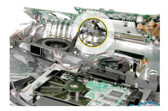
5. Disconnect the power supply cable and carefully lift the logic board out of the chassis.
