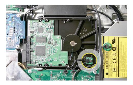
2. Note: If you are replacing the hard drive, transfer the temperature sensor to the replacement hard drive. Use the double-stick tape enclosed with the replacement hard drive to attach the sensor. Continue on to the next step.
