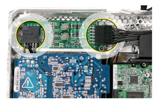
2. Using a T10 torx screwdriver, remove the self-tapping screw from the top corner of the DC-DC board and the black self-tapping screw below it. Lift the board straight up to remove it.
