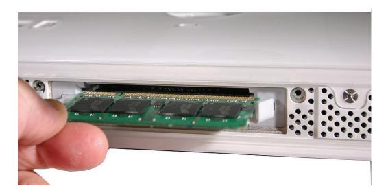
3. With your fingers, press the DIMM fully into the slot until you hear a click. After inserting the memory, fold the DIMM levers closed. There will be a slight resistance and you will hear a click when they fold into the closed position.
