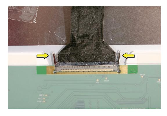
2. Pinch together the connector locking levers, and disconnect the LVDS cable connector.
