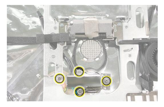
3. Peel the EMI tape off the AC filter.
