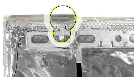
2. Remove two pieces of tape that secure the antenna cable to the rear housing (near the power on LED, in the bottom left corner). Pull the antenna cable through the access hole in the EMI shield at the top, near the antenna board.
