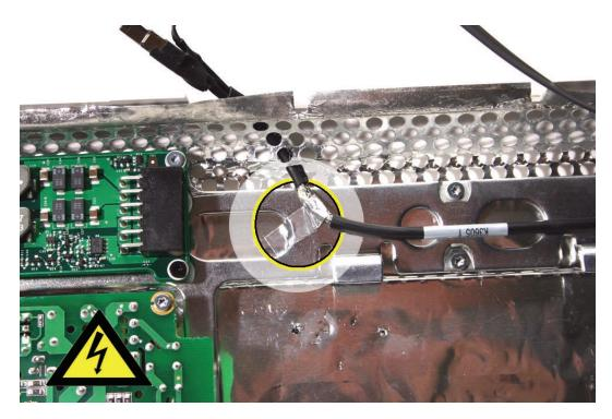
3. Route the camera cable as shown, and tape the camera cable and DC power cable to the rear housing as shown below.
