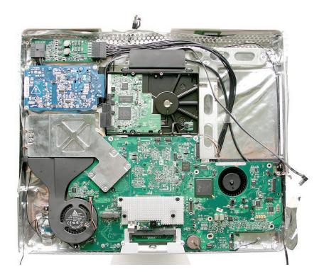
4. With the stand facing you, lift the board and locate the black power connector on the underside of the board (on the right side) Refer to the next photo for a close up.
