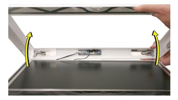
2. Disconnect the camera and microphone cables.
