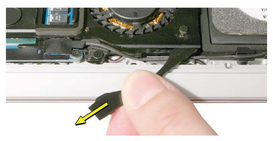
10. With the cosmetic fan cover removed, lift the mylar tab shown below to expose the microphone cable's connection to the logic board.
