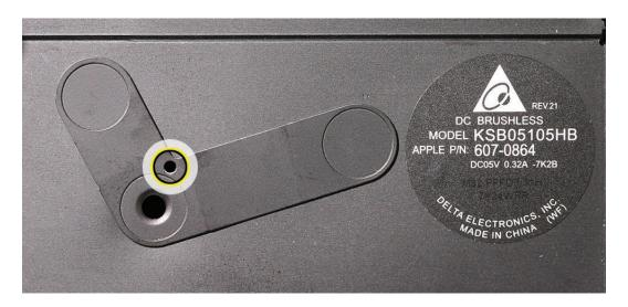
4. Install one #00 Phillips screw in the upper left corner near the fan, two #000 screws in the clips on the right upper and lower corners of the thermal module, and then fasten the center #000 screw on the boomerang clamp last. Do not overtighten the center screw.
