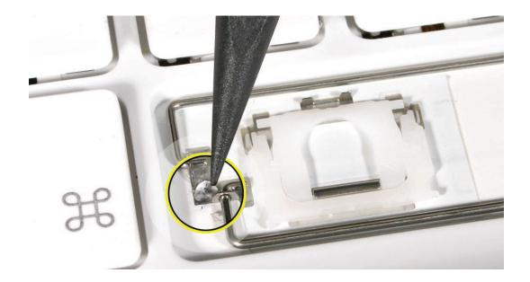
3. Test the operation of the scissor mechanism by using a black stick to carefully raise and lower the mechanism.
