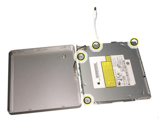
10. Immobilize the drive while removing screws or components, holding the drive enclosure by the bracket or edges only.
