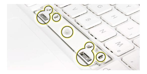
6. With the scissor mechanism open, install the slider bar under the metal hook of the top case.
