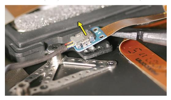
5. Carefully disconnect the audio-out cable connector (shown below).
