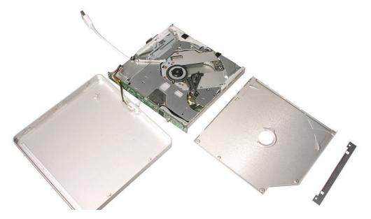
15. Orient the bottom outer case properly to the top case, as below—three tabs per side on the left and right sides of the drive, no tabs in the front (where the disc insertion slot is located), and two outer corner tabs in the back (where the USB cable is attached).
