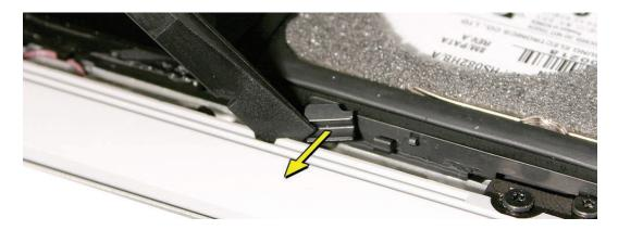
16. Remove the four Phillips screws from the hard drive bracket. Disconnect the hard drive flex cable to the logic board. (Note that unlike the photo below, the port hatch assembly does not need removal in order to remove the hard drive.)
