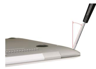
While holding the bottom case at a 30° angle, insert the clips on its front edge into the tabs on the top case before lowering into place. Make sure no cables are pinched (e.g., the AirPort/Bluetooth antenna assembly on the right side and the microphone cable in the rear).
