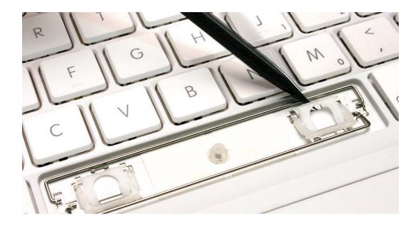
9. Check the keycap well area on the top case. If the bottom stabilizer bar is pushed up, move it down as far as it will go.
