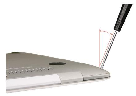
1. Remove ten Phillips #000 screws, starting from the top center and moving outward in a circular fashion in both directions.
