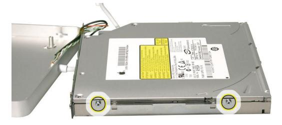
13. Lift the top of the drive enclosure, pivoting the right edge up while sliding it sideways left and downward to disengage the the left edge.
