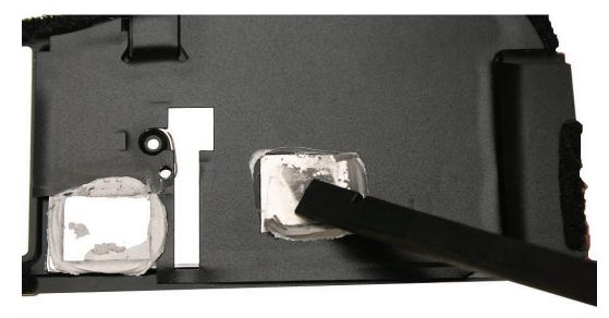
3. Use an alcohol wipe to completely clean the residual thermal paste from the two chips on the logic board and the two pads on the heatsink.
