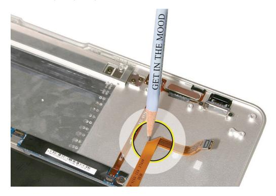
3. As in the above step, use the pencil to very lightly trace the upper bend in the cable onto the black mylar, precisely from fold to fold, being careful of the keyboard assembly beneath.
