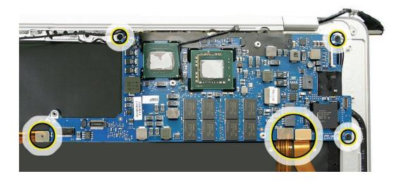
3. When removing the logic board, grasp the board in the middle lengthwise by the edges only. Do not hold the board by any narrow areas. Take all ESD precautions when handling it.
