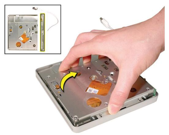
9. As if opening the page of a book, flip the drive up and over the edge and gently lay it down, keeping the edges as close together as possible to avoid straining the cable connections.
