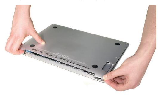
3. Pivot the rear edge upward a few inches to a 30° angle. At that same angle, pull the bottom case outward from the front edge of the top case to preserve the integrity of the front clips.
