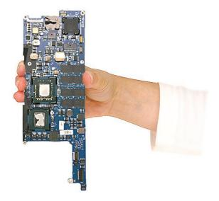
**Warning:** To avoid flexing the logic board, hold the board vertically along the wide sides. Do not hold the board by the ends or by the narrow neck at the fan cutout, or horizontally, as the board's weight can cause excessive flex.
