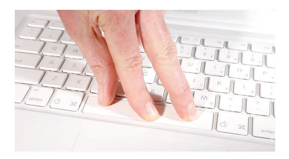
15. Check the key from all angles to make sure it is uniformly flat. Press and release one corner of the key. If the key is installed correctly, the opposite corner should respond at the same level (not tilted higher or lower).
