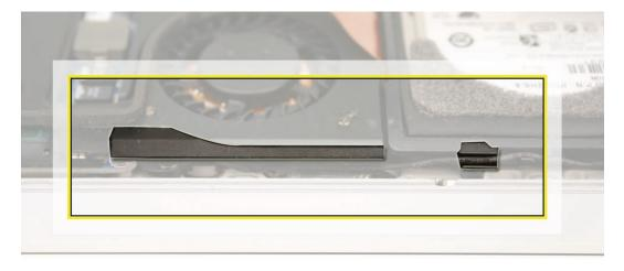
8. Begin to remove the cosmetic fan cover using a black stick to wedge it out from the left side.
