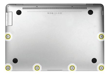
2. When reinstalling the new shoulder screws, make sure the head of the screw sits flush with the bottom case after installation.
