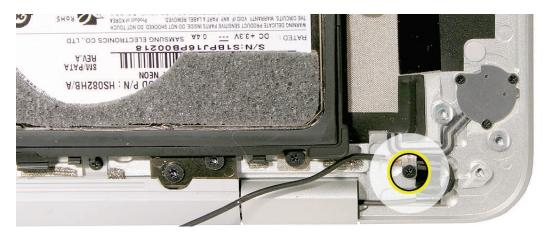
12. Note the cable routing under a clip on the fan and two sets of clips on the hard drive frame.
