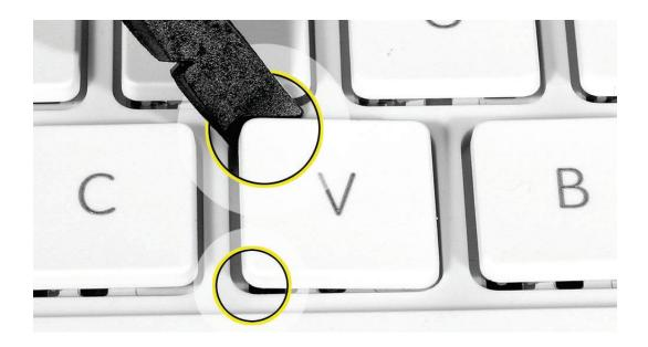
2. Because adhesive is used under the top case, closely inspect the case for any adhesive that may have built up under the keycap. Lift away any built-up adhesive using a black stick or fine-point tweezers.
