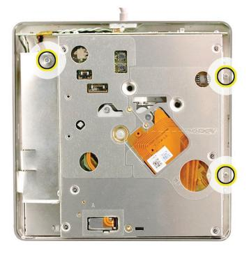
5. Note the tab on the lower left of the drive casing which fits into a recessed slit in the outer enclosure (shown in left blowout area below.) Then, on the opposite side of the drive, look for the indentation in the center of the right edge of the drive (highlighted below on right).
