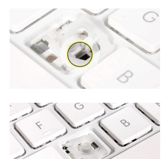
6. With the scissor mechanism open, install the slider bar under the metal hook of the top case.
