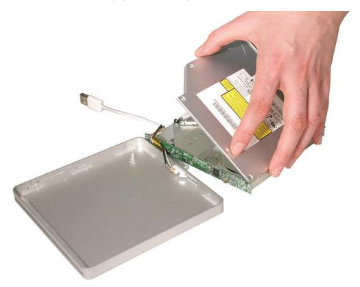
14. Remove the stuck disc, and reassemble the optical drive enclosure in the reverse order of the previous steps: 4-13, up to the point at which the outer case would be put back together.
