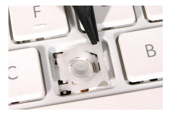
9. Moving from left to right, slide the right end of the keycap into the keycap well so that the hooks inside the right side of the keycap latch onto the pins on the right side of the scissor mechanism.
