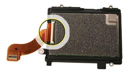
20. Carefully release the small black ZIF connector lever with a black stick.
