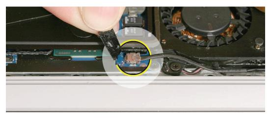
11. Disconnect the microphone cable connector from the logic board using the pointed end of the black stick to push the side tabs on the connector.
