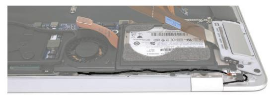
**Note:** Notice two black plastic cosmetic pieces designed to prevent screws and cabling from being visible through vent holes in the bottom case—one molded to fit the edge of the fan and a smaller piece molded to fit the hard drive frame. You will remove them in this procedure.
