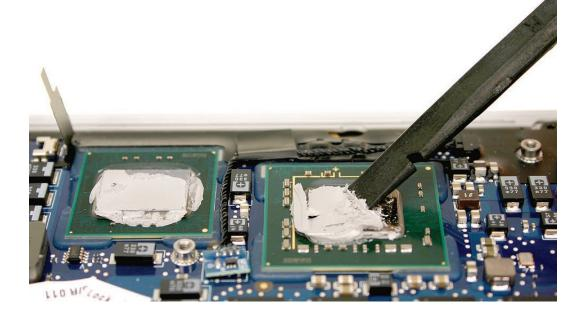
2. Use a black stick to remove thermal paste from the two mating pads on the under side of the thermal module.
