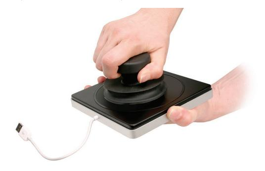
3. Once the suction cup is fully adhered, lift straight up, pulling the black bottom case directly out of the silver top case in one smooth motion.
