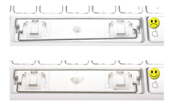
10. Determine which is the top of the Space bar keycap by checking the clips on the inner plane. The top of the keycap has the row of clips that extend closest to the sides of the keycap. These top clips most closely match the longest stabilizer bar at the top of the keycap well.
