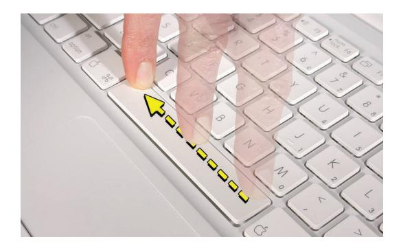
14. Press the length of the Space bar to ensure all clips are secure.
