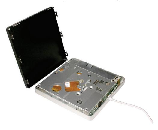
16. Set the bottom case evenly on the top case with the tabs just inside the perimeters of the top case edges. Make sure all tabs line up with the top case; and if not, adjust accordingly.
