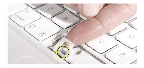
7. Allow the scissor mechanism to fold flat and hold the slider bar in place while using a black stick to insert the scissor pins—one at a time—into the top case ears.
