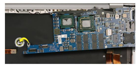
2. Install three identical Phillips screws in the order called out below.
