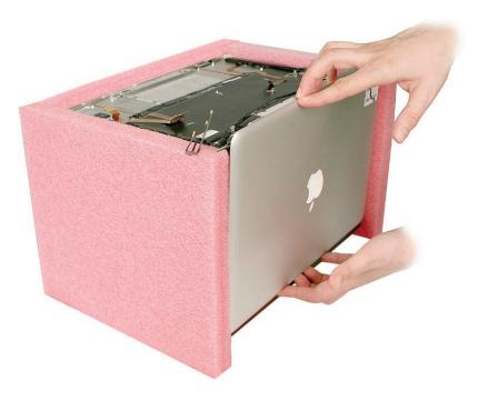
2. If necessary, slide the antenna assembly a millimeter or two to the left or right to fully align the holes.
