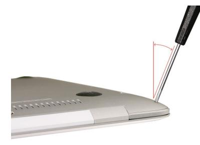
The front edge of the bottom case has five fragile metal clips that fit into five overhanging tabs on the top case. Be sure to remove and reinstall the bottom case at a 30° angle.
