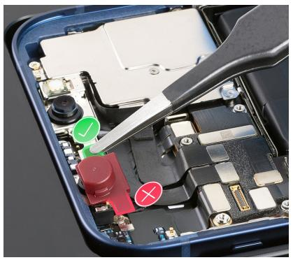
11. Inspect the TrueDepth camera. Ensure that the top edge of the TrueDepth camera is under the lip of the enclosure.
