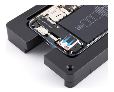
4. Use the green torque driver and JCIS bit to install four new crosshead screws (923-05052) into the speaker.
