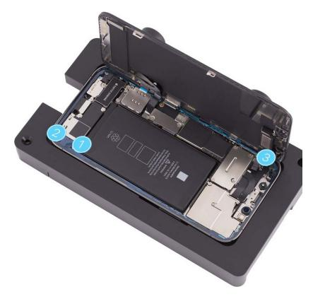
20. Inspect the display adhesive to ensure that it's in the correct position and isn't damaged or wrinkled. If the adhesive is damaged, remove it and apply replacement adhesive.
