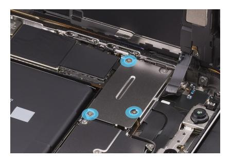
24. Hold the upper cowling in place and use a torque driver and the Micro stix bit to remove the last trilobe screw. Set aside the screw.
