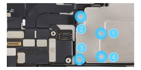
8. Use the gray torque driver and JCIS bit to install one new crosshead screw (923-05069) into the camera cowling.
