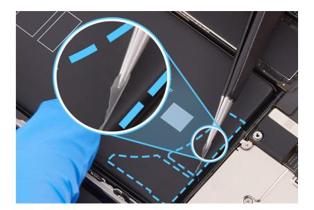
12. Keep the tweezers in the channel between the battery and the camera cowling. Continue to slowly twist the tweezers until you've removed the entire adhesive strip.
