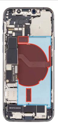
15. Insert the flat end of the black stick only into one of the insertion points as shown. Ensure that the black stick is inserted into a point where the battery strip has been fully removed. Don't insert the black stick into a point where the battery tab or strip is broken.
