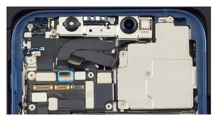
4. Use the flat end of the black stick to separate the adhesive between the TrueDepth camera flex cables and the enclosure as shown.
