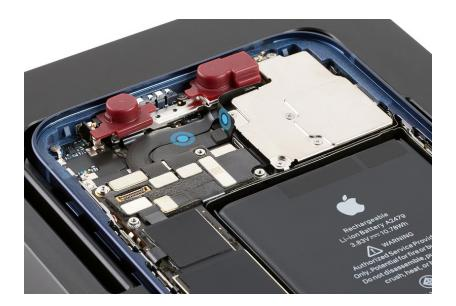
10. Use ESD-safe tweezers to remove the protective covers from the TrueDepth camera.
