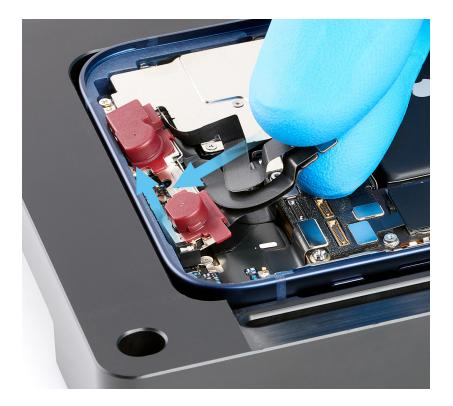
6. Then gently slide the left side of the TrueDepth camera assembly under the lip of the enclosure to engage the grounding pin.
