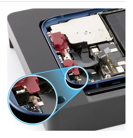
8. Press the ends of the three TrueDepth camera flex cables to the connectors.
