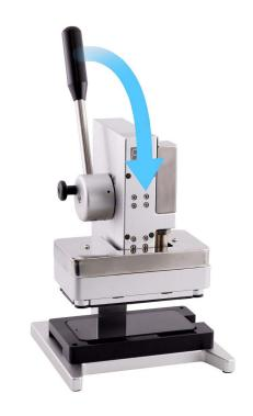
26. Wait until the display press beeps and the timer shows 0. Pull down the lever (1) and pull out the release knob (2). Then lift the lever (3).
