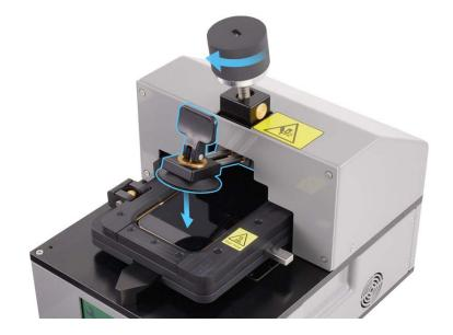
8. Grasp the handle and slide the suction cup straight out until the edge of the suction cup aligns with the bottom edge of the display.
