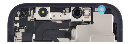
3. Use a torque driver and the Micro stix bit to remove the four trilobe screws from the camera cowling in the order shown. Set aside the screws.
