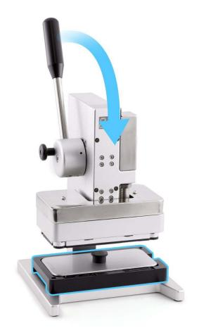
8. Wait until the display press beeps and the timer shows 0. Pull down the lever (1) and pull out the release knob (2). Then lift the lever (3).
