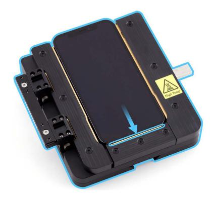
4. Flip down the clamp on the side of the pocket to lock the iPhone into place.
