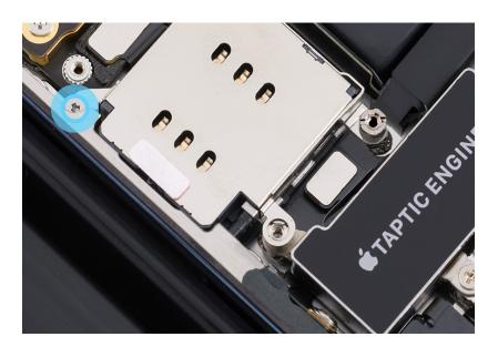
7. Use the gray torque driver and super screw bit to install one new super screw (923-04980) into the lower right corner of the SIM reader.
