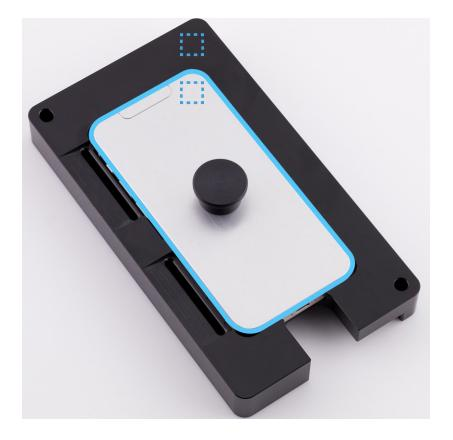
7. Position the repair tray with the iPhone in the display press. Pull down the lever until the display press locks.
