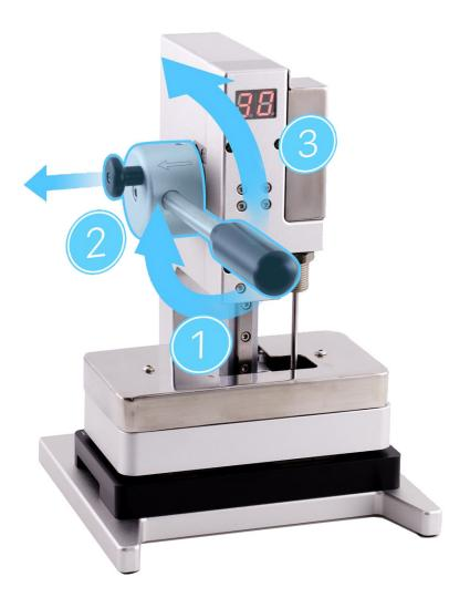
27. Remove the repair tray from the display press.
