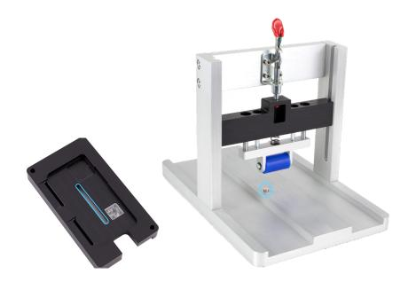
5. Flip down the red lever at the top of the battery press to lower the roller onto the battery.
