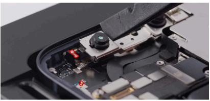
4. Align the replacement display adhesive over the enclosure with the top holes over the TrueDepth camera assembly and the bottom tab on the left.
