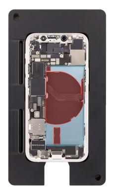
13. Insert the flat end of the black stick only into one of the insertion points as shown. Ensure that the black stick is inserted into a point where the battery strip has been fully removed. Don't insert the black stick into a point where the battery tab or strip is broken.
