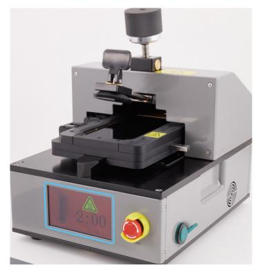
7. Turn the knob on the fixture clockwise to lower the suction cup as close to the iPhone as possible without touching the iPhone.
