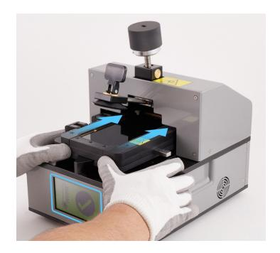
**Note:** The screen on the fixture will turn red and the timer will count down from 2 minutes while the pocket heats to the correct temperature. When the timer ends, the fixture will start to beep and the screen will turn green.
