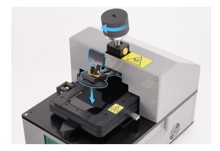
8. Grasp the handle and slide the suction cup straight out until the edge of the suction cup aligns with the bottom edge of the display.
