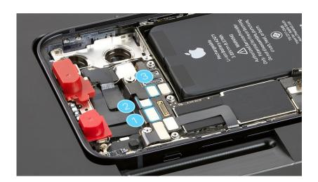
5. Use tweezers to remove the protective lens caps from the TrueDepth camera.
