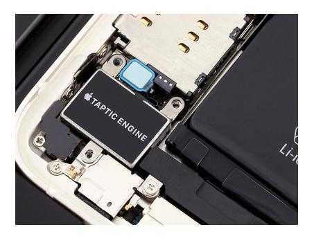
7. Use ESD-safe tweezers to remove the Taptic Engine.
