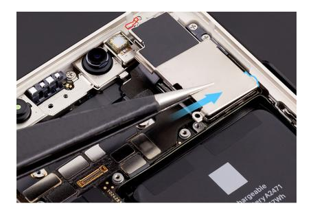
8. Use the gray torque driver and JCIS bit to install two new crosshead screws (923-04991) into the camera cowling.
