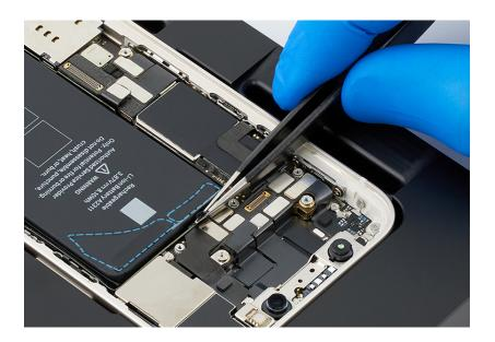
9. Hold down the iPhone. Use ESD-safe tweezers to grasp one battery adhesive tab and slowly pull it outward. Twist the tweezers to wrap the battery adhesive strip around them.
