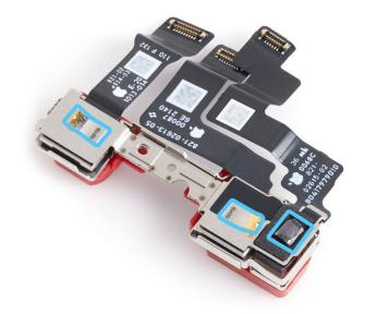
2. Slide the left edge of the TrueDepth camera underneath the lip of the enclosure first to engage the grounding pin (1). Then slide the right edge of the TrueDepth camera underneath the lip of the enclosure (2).
