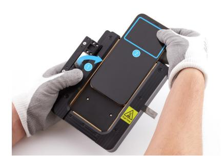
16. Place the enclosure in the repair tray with the display faceup and the Lightning connector facing the cutout. Remove the gloves.
