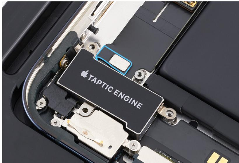
3. Use the green torque driver and JCIS bit to install one new crosshead screw (923-04981) into the Taptic Engine.
