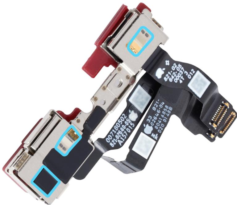
4. Hold the TrueDepth camera flex cables together and turn over the TrueDepth camera assembly.
