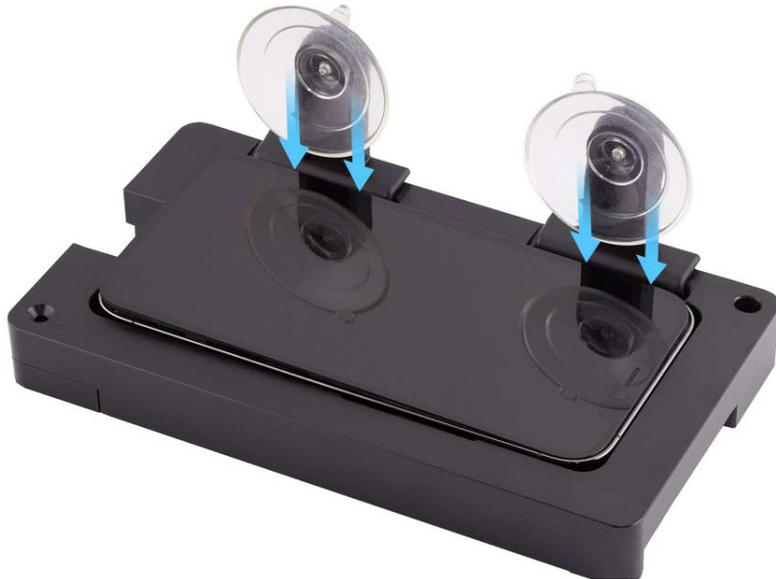
20. Tilt up the display toward the suction cups. Press the top and bottom edges of the display to secure it to the suction cups.
