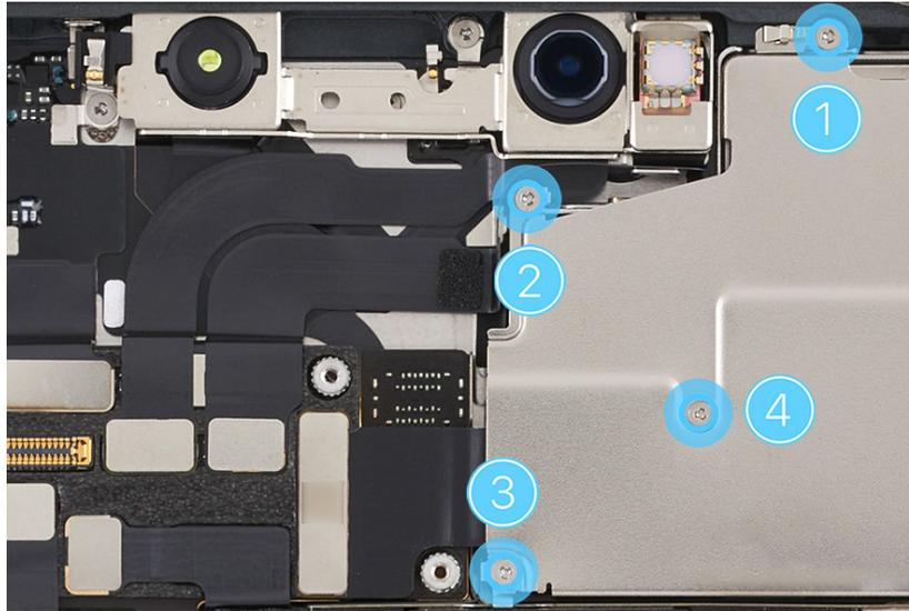
3. Use ESD-safe tweezers to tilt up the left side of the camera cowling as shown. Then slide the camera cowling out of the enclosure. Save the cowling for reassembly.
