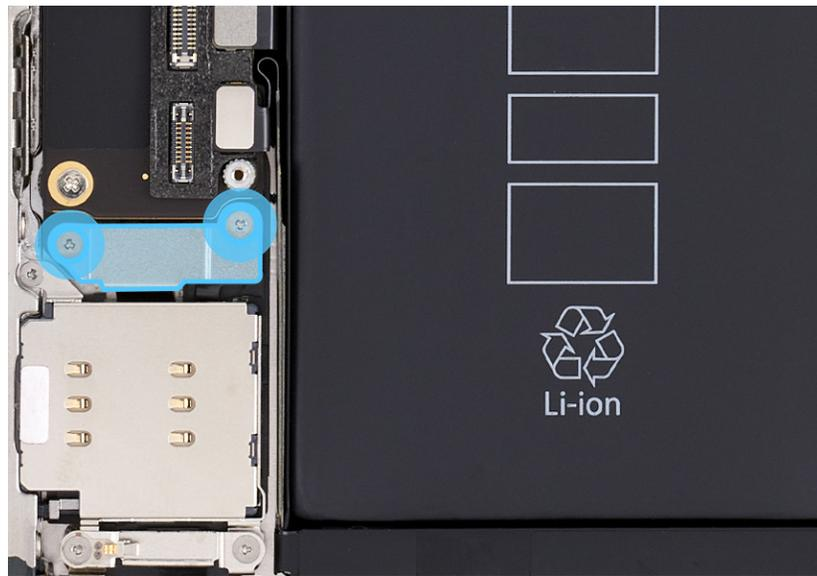
5. Use ESD-safe tweezers to remove the SIM reader connector cowling. Save the cowling for reassembly.
