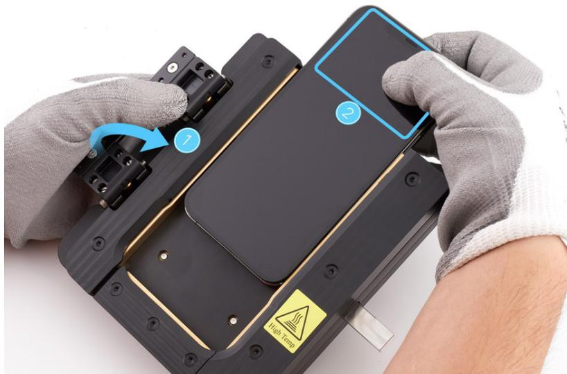
16. Place the iPhone into the repair tray with the display faceup and the Lightning connector facing the cutout. Remove the gloves.
