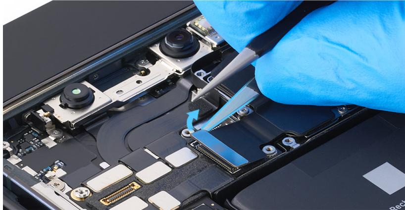
5. Use ESD-safe tweezers to gently lift the end of the bottom camera flex cable off the connector.
