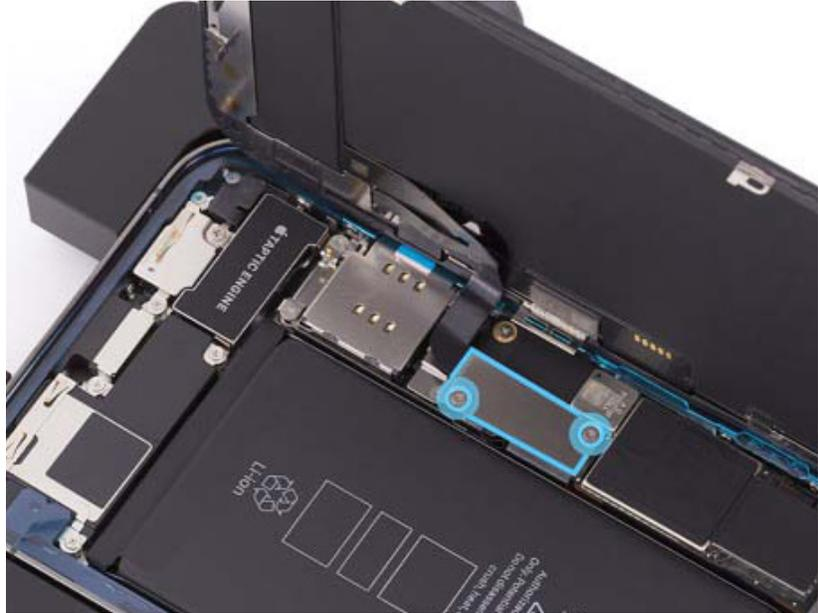
17. The upper cowlings has a tab near the second screw hole (2) that fits into a slot near the camera cowlings. Use ESD-safe tweezers to fit the tab into the slot. Then lower the cowlings over the end of the receiver flex cable.
