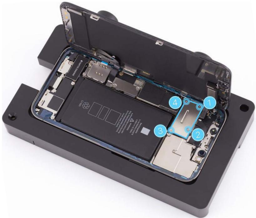
19. Peel the first strip of the middle release liner (1) counterclockwise, starting near the bottom right of the enclosure. Peel the second strip (2) clockwise, starting near the bottom right of the enclosure. Peel the third strip (3) counterclockwise, starting near the top left of the enclosure.
