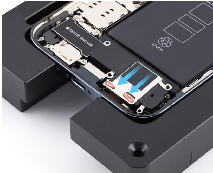
3. Use the green torque driver and JCIS bit to install four new crosshead screws (923-05052) into the speaker.
