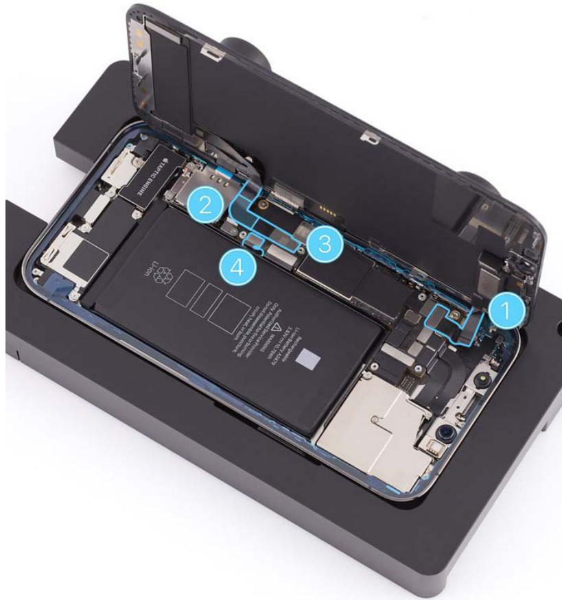
15. Use ESD-safe tweezers to position the lower cowlings over the ends of the Multi-Touch, display, and battery flex cables.
