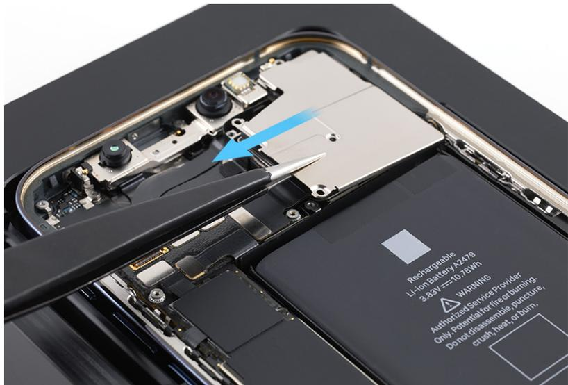
4. Use ESD-safe tweezers to gently lift the end of the top camera flex cable off the connector.
