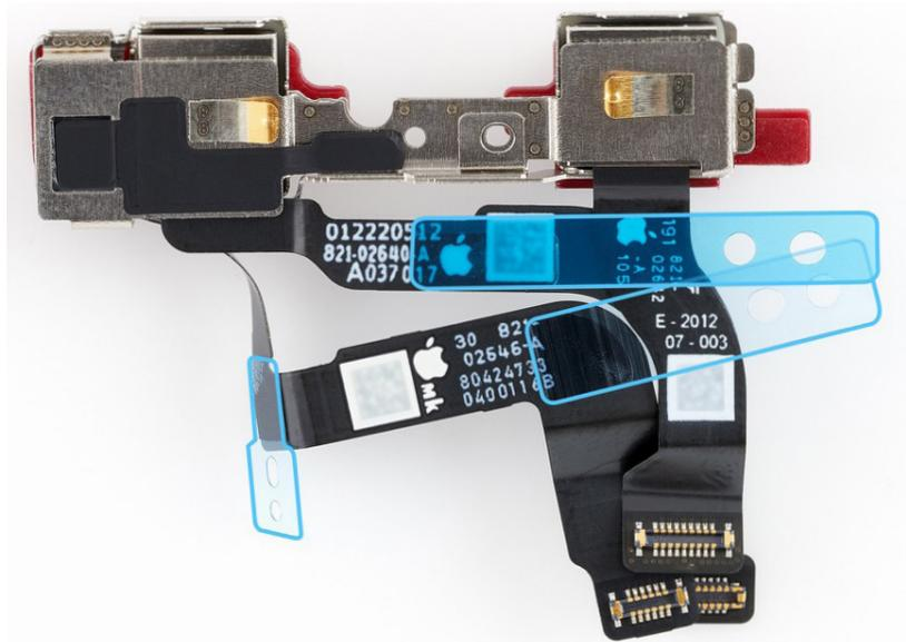
3. Inspect the back of the TrueDepth camera assembly to ensure that the grounding foam and grounding springs are intact. If either is missing or damaged, replace the TrueDepth camera assembly.
