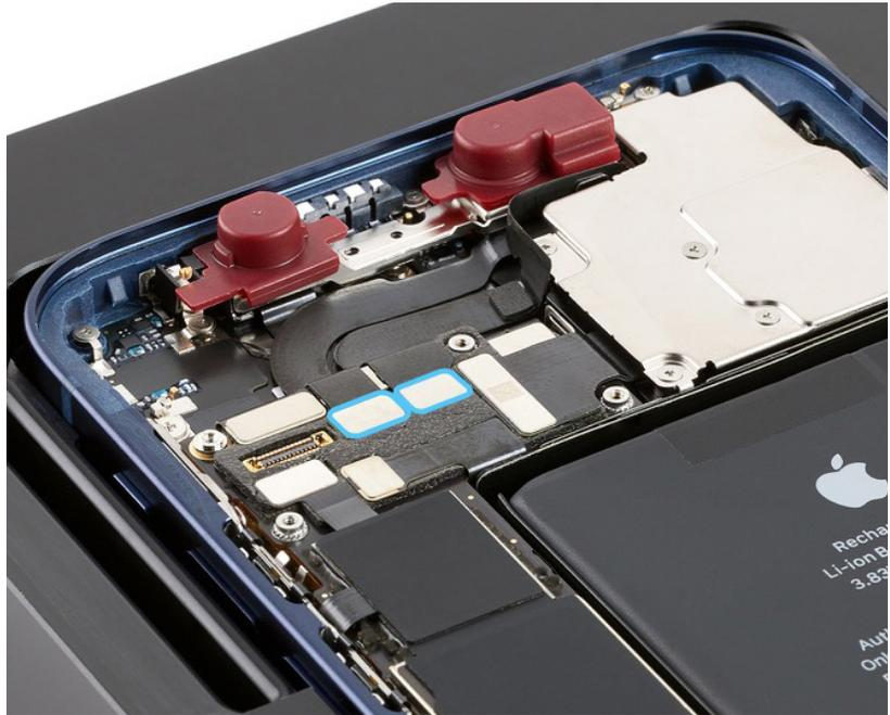
9. Lightly press the TrueDepth camera flex cables on the areas shown to adhere the flex cables into place.
