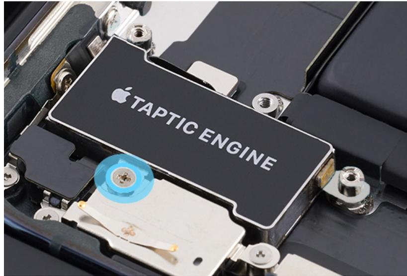
4. Use the gray torque driver and super screw bit to install two new super screws (923-04980) into the Taptic Engine.
