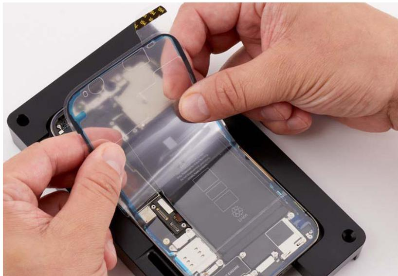
6. Place the display adhesive press plate on top of the enclosure with the icon in the top right corner as shown.
