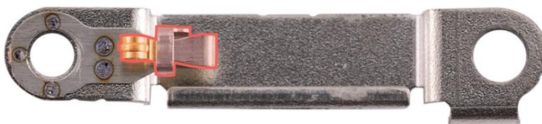
11. Use the black torque driver and Micro stix bit to install four new trilobe screws (923-04978) into the SIM reader and Taptic Engine connector cowlings.
