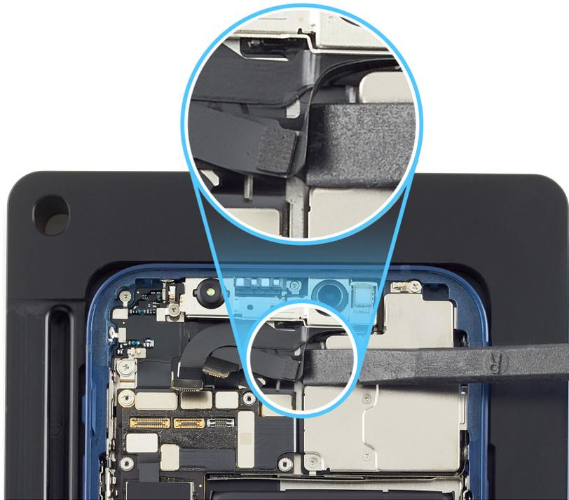
5. Gently hold the TrueDepth camera flex cables together. Then lift the TrueDepth camera assembly at a 45-degree angle to disengage the grounding pin on the left.
