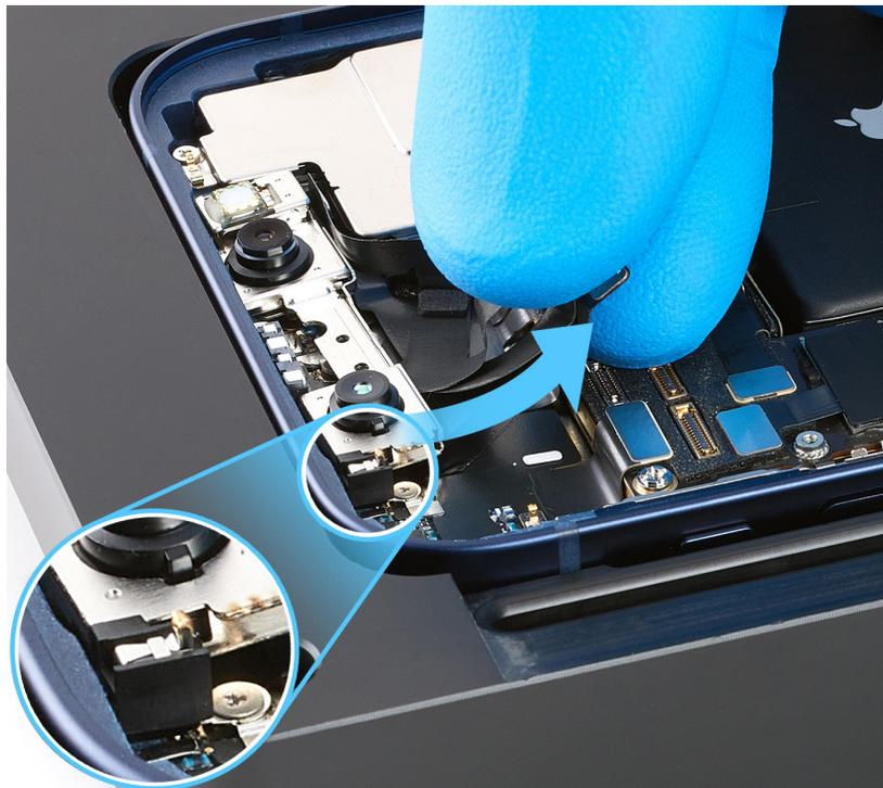
6. Slide the TrueDepth camera assembly out of the enclosure.
