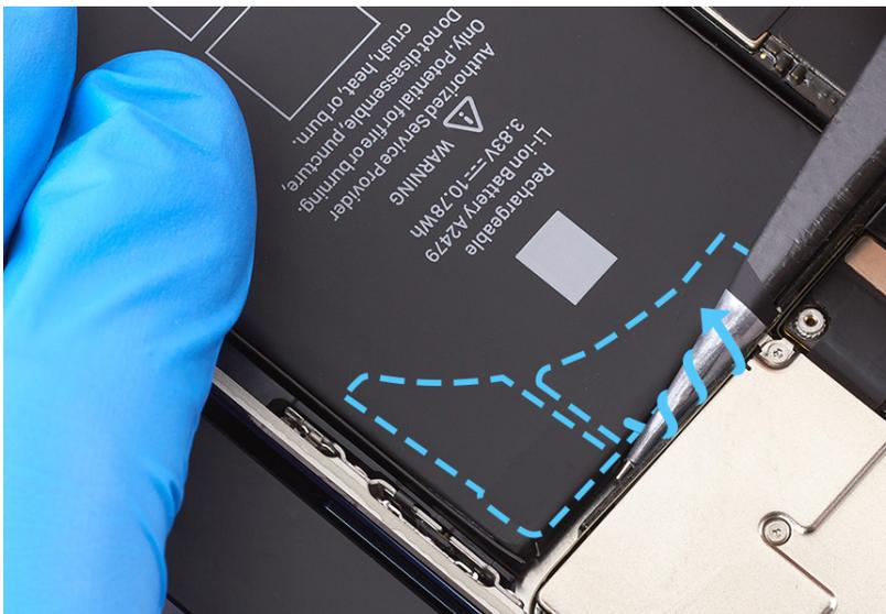
13. Repeat steps 11 and 12 to remove the remaining battery adhesive strip from the top of the battery. If you remove the entire strip, continue to step 14.
