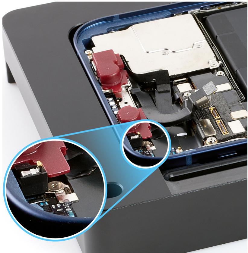
8. Press the ends of the three TrueDepth camera flex cables to the connectors.
