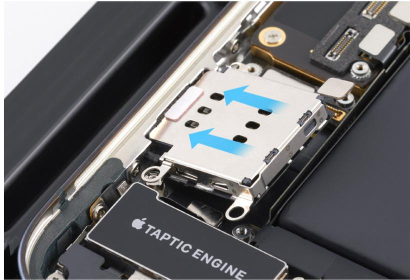
6. Use the black torque driver and Micro stix bit to install one new trilobe screw (923-04982) into the upper left corner of the SIM reader.
