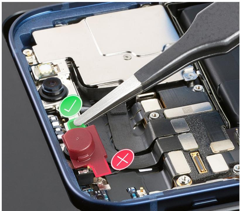
11. Inspect the TrueDepth camera. Ensure that the top edge of the TrueDepth camera is under the lip of the enclosure.
