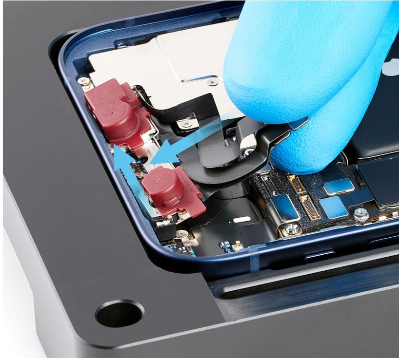
6. Gently slide the left side of the TrueDepth camera assembly under the lip of the enclosure to engage the grounding pin.
