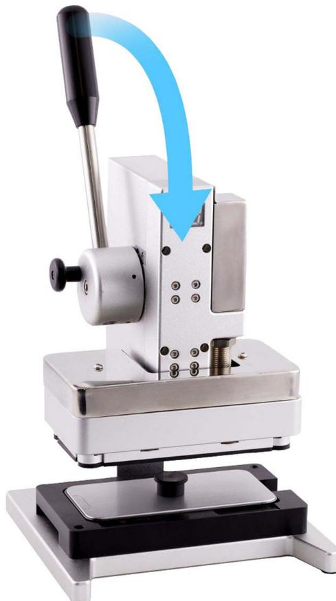
8. Wait until the display press beeps and the timer shows 0. Pull down the lever (1) and pull out the release knob (2). Then lift the lever (3).
