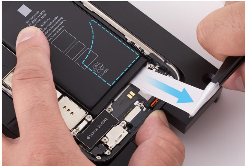
7. Use ESD-safe tweezers to grasp the bottom left battery adhesive tab. Gently peel the adhesive tab away from the battery.
