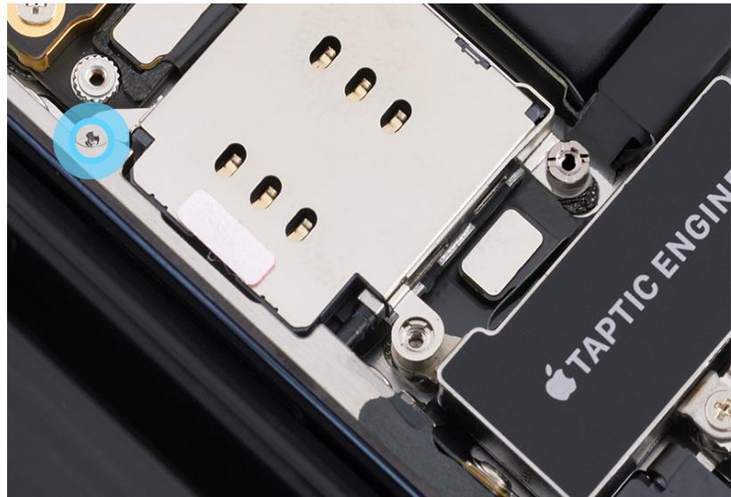
7. Use the gray torque driver and super screw bit to install one new super screw (923-04980) into the lower right corner of the SIM reader.
