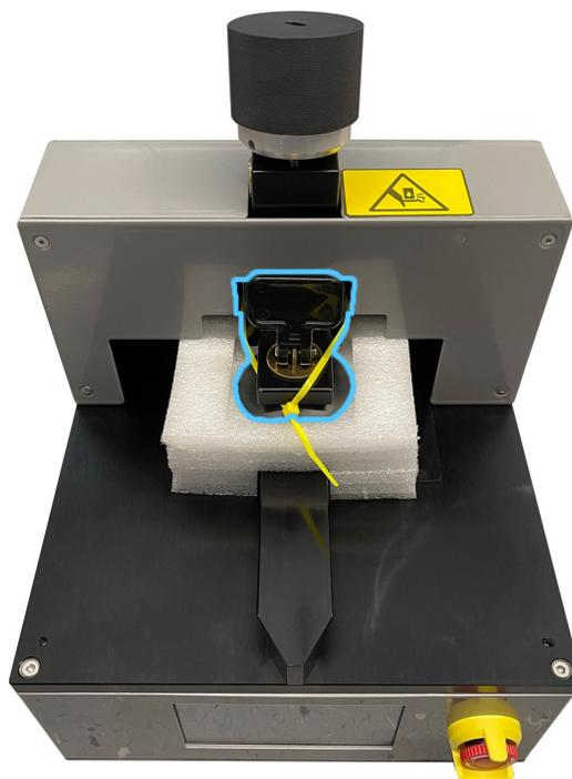
3. Turn the top knob on the fixture counterclockwise to raise the suction cup. Remove the packing foam.
