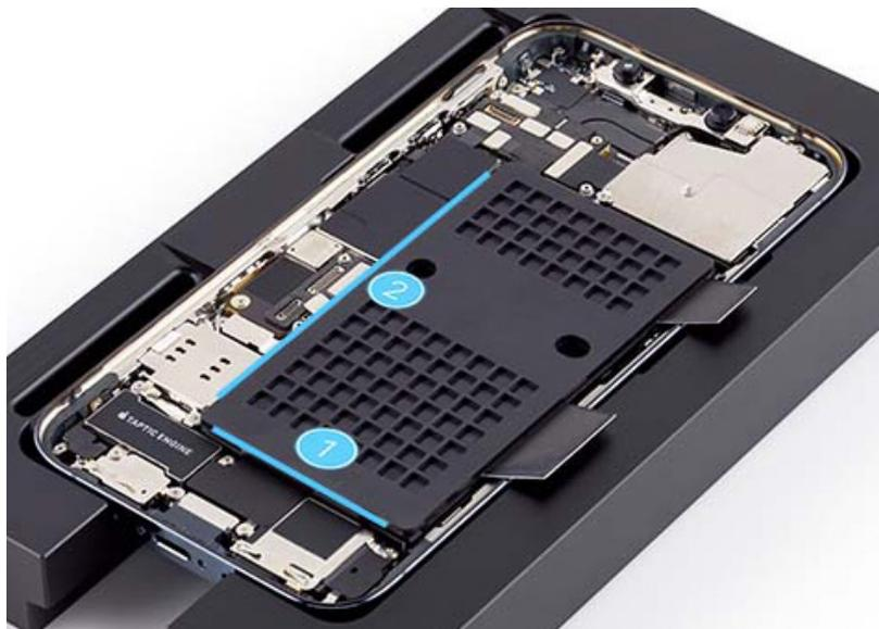
6. The center of the repair tray has two slots. Position the repair tray and enclosure onto the battery press with the left slot over the pin as shown.
