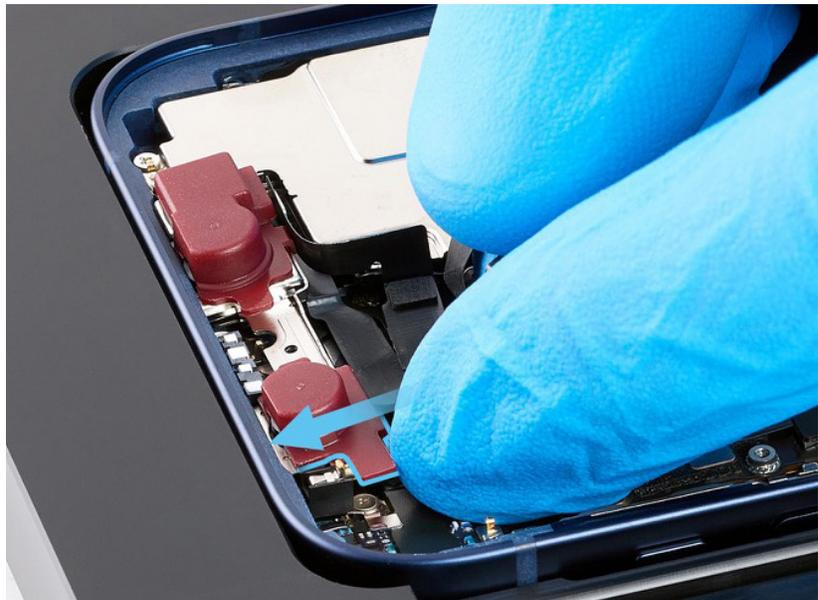
7. Inspect the TrueDepth camera assembly to ensure that the top edge of the TrueDepth camera is under the lip of the enclosure and the grounding pin is flush with the enclosure.
