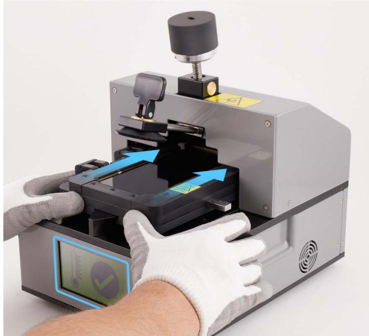
**Note:** The screen on the fixture will turn red and the timer will count down from 2 minutes while the pocket heats to the correct temperature. When the timer shows 0, the fixture will start to beep and the screen will turn green.
