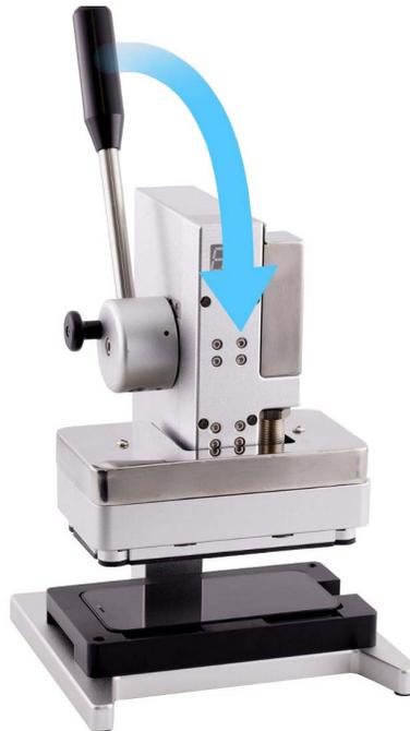
26. Wait until the display press beeps and the timer shows 0. Pull down the lever (1) and pull out the release knob (2). Then lift the lever (3).
