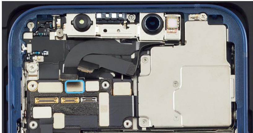
4. Use the flat end of the black stick to separate the adhesive between the TrueDepth camera flex cables and the enclosure as shown.
