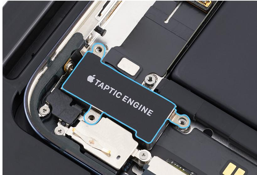
2. Press the end of the Taptic Engine flex cable to the connector.
