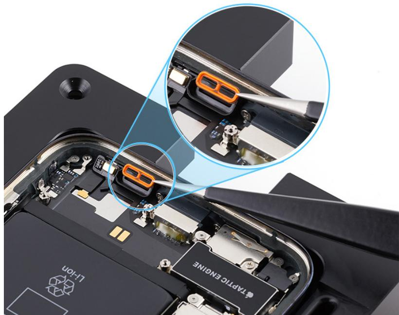
2. Rotate the repair tray. Tilt down the speaker and lower it into position.
