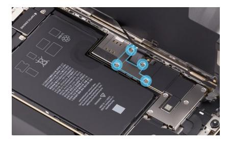
22. Use ESD-safe tweezers to remove the lower cowling. Save the cowling for reassembly.
