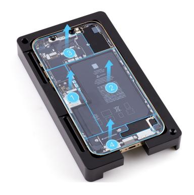
11. Insert the suction cups into the repair tray.
