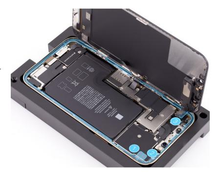
20. Inspect the display adhesive to ensure that it's in the correct position and isn't damaged or wrinkled. If the adhesive is damaged, remove it and apply replacement adhesive.
