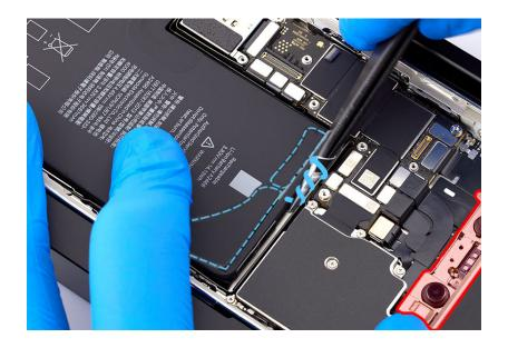
12. Repeat steps 10 and 11 to remove the remaining adhesive strip from the top of the battery. If you remove the entire strip, continue to step 13.
