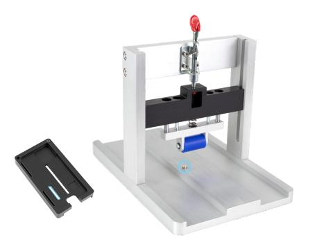
10. Flip down the red lever at the top of the battery press to lower the roller onto the battery.
