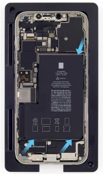
15. Slightly lift the battery with the black stick just enough to grasp underneath the battery.
