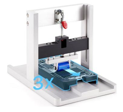
12. Flip up the red lever at the top of the battery press.
