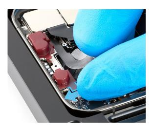
4. Inspect the TrueDepth camera assembly to ensure that the top edge of the TrueDepth camera is under the lip of the enclosure and the grounding pin is flush with the enclosure.
