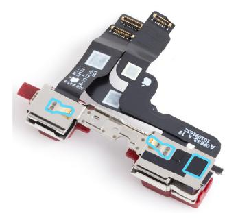
3. Tilt the top edge of the TrueDepth camera assembly under the lip of the enclosure as shown. Lower the camera into the enclosure.
