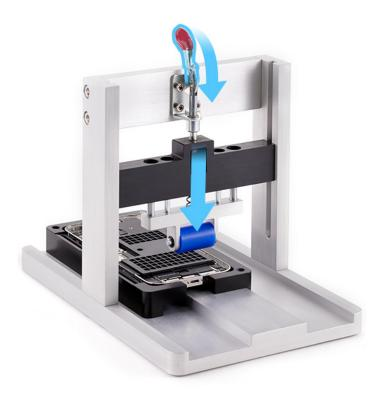
15. Slide the repair tray back and forth through the battery press three times to adhere the battery to the enclosure.
