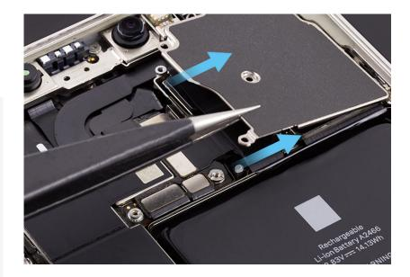
9. Hold the camera cowling in place with your finger. Use the green torque driver and Micro stix bit to install five new trilobe screws (923-05028) into the camera cowling in the order shown.
