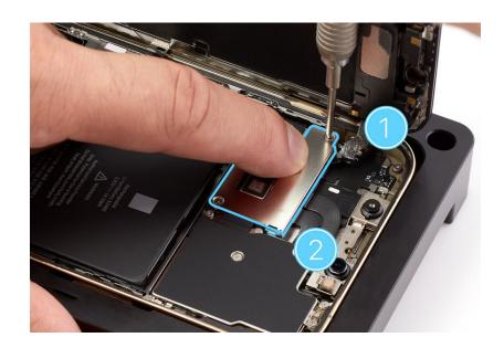
26. Use the black stick to lift the end of the battery flex cable off the connector (1).
