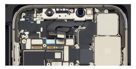
4. Gently grasp the flex cables and remove the TrueDepth camera at a 45-degree angle to disengage the grounding pin on the left side of the TrueDepth camera.
