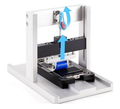
13. Position the repair tray and enclosure onto the battery press with the right slot over the pin.
