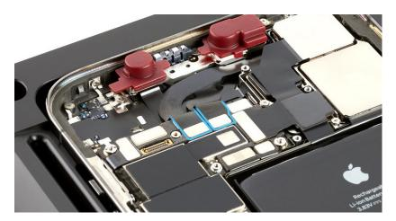
6. Use ESD-safe tweezers to remove the protective covers from the TrueDepth camera.
