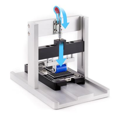
11. Slide the repair tray back and forth through the battery press three times to adhere the battery to the enclosure.
