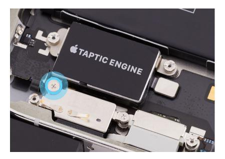
6. Use the black stick to lift the end of the Taptic Engine flex cable off the connector.
