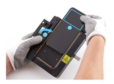
16. Place the iPhone into the repair tray with the display faceup and the Lightning connector facing the cutout. Remove the gloves.
