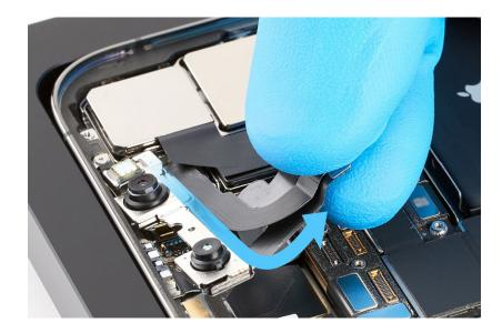
5. After the hook is disengaged, slide the TrueDepth camera out of the enclosure.
