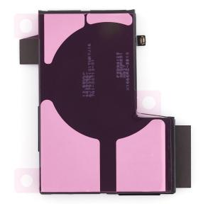
8. Hold the battery over the enclosure with the protective cover faceup. Align the bottom of the battery with the Taptic Engine (1) and the right edge with the enclosure (2). Then lower the battery into the enclosure.
