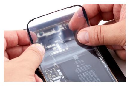
6. Place the display adhesive press plate on top of the enclosure with the icon in the top right corner as shown.
