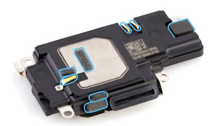
3. Rotate the repair tray. Align the port on the speaker with the hole in the enclosure. Then lower the speaker into position.
