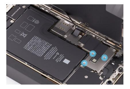
24. Hold the upper cowling in place and use a torque driver and the Micro stix bit to remove the last trilobe screw (1). Set aside the screw.
