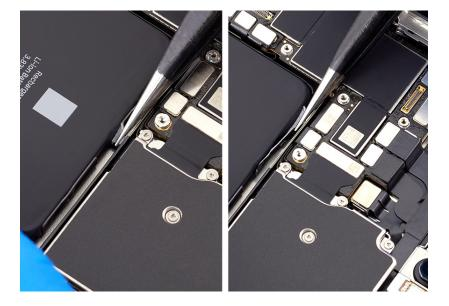
10. Hold down the iPhone. Use ESD-safe tweezers to grasp one battery adhesive tab. Twist the tweezers to wrap the adhesive strip around them.
