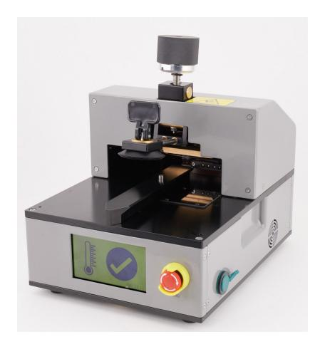
3. Gently insert the iPhone into the heated display pocket with the display faceup and the Lightning connector facing the bottom of the pocket.
