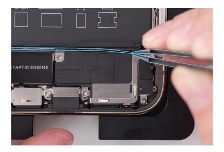
5. Use the black stick to tilt up the speaker. Then remove the speaker from the enclosure.
