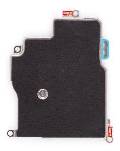
8. Hold the cowling with ESD-safe tweezers and slide the cowling tab into the slot. Then lower the cowling onto the cameras.
