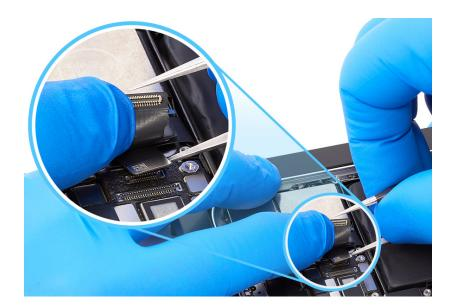
6. Gently hold the camera flex cables together and lift the cameras out of the enclosure.
