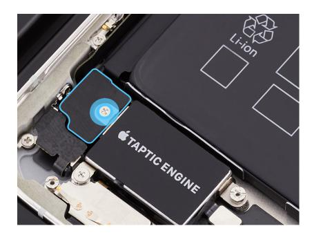
4. Use a torque driver and the super screw bit to remove the two super screws from the Taptic Engine. Set aside the screws.
