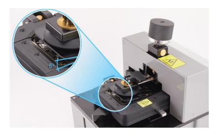
12. Flip up the handle to release the suction cup (1). Gently slide the flat end of the black stick under the edge of the suction cup to release it from the display (2).
