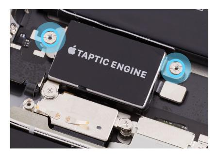
4. Use the green torque driver and JCIS bit to install one new crosshead screw (923-05038) into the Taptic Engine.
