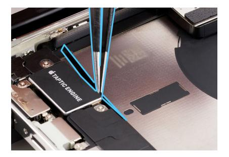
6. Use the flat end of the black stick to adhere the battery shim to the Taptic Engine and speaker.
