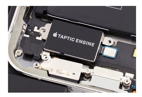
3. Use the gray torque driver and super screw bit to install two new super screws (923-05037) into the Taptic Engine.
