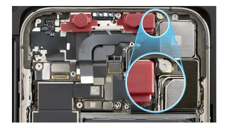
5. Press the ends of the three TrueDepth camera flex cables to the connectors.
