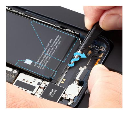
4. Keep the tweezers close and parallel to the battery and twist until you see white adhesive strip on the tweezers.
