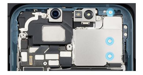
3. Use ESD-safe tweezers to tilt up the right edge of the camera cowling (1). Then pull the cowling to the right to release the tabs on the left (2). Save the cowling for reassembly.
