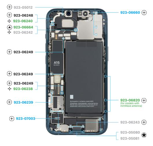
Torque driver (black, 0.35 kgf cm) Torque driver (green, 0.45 kgf cm) Torque driver (gray, 0.55 kgf cm) Torque driver (blue, 0.65 kgf cm)
