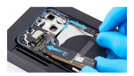
9. Press the end of the mmWave antenna flex cable to the connector.
