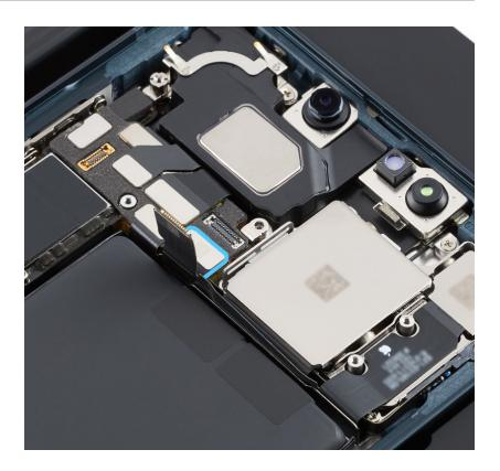
4. Press the end of the top camera flex cable to the connector.
