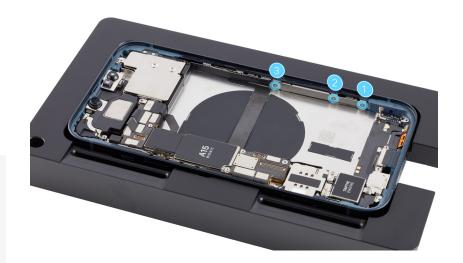
4. Separate the end of the mmWave antenna flex cable from the connector.
