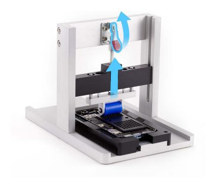
13. Remove the repair tray from the battery press.
