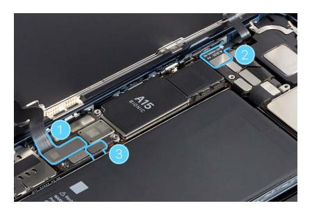
16. Use ESD-safe tweezers to position the lower cowling over the ends of the display and battery flex cables.
