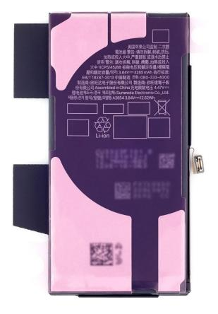
4. Hold the battery over the enclosure with the protective cover faceup. Align the bottom of the battery with the top of the speaker (1) and the left edge with the logic board (2). Then lower the battery into the enclosure.
