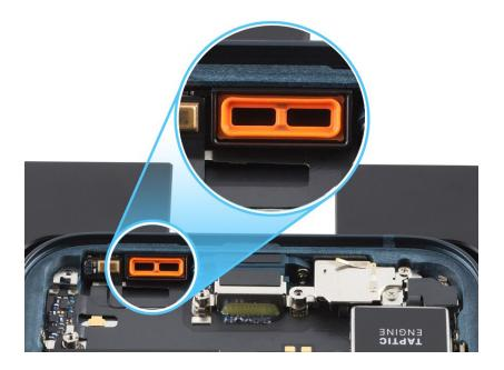
2. Tilt down the bottom edge of the bottom speaker and lower it into the enclosure.
