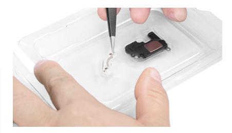
2. Use ESD-safe tweezers to remove the release liners from the underside of the grounding strap and position it on the top speaker.
