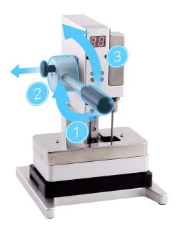
28. Remove the repair tray from the display press.
