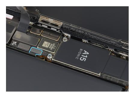
27. Use the black stick to lift the end of the display flex cable off the connector.
