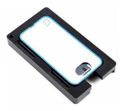
8. Position the repair tray with the iPhone in the display press. Pull down the lever until the display press locks.
