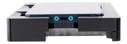
2. Flip the switch on the back of the heated display removal fixture to turn it on. The internal fan will turn on. Wait for a checkmark to appear on the screen.
