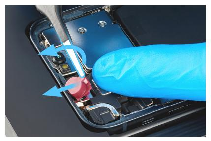
6. Inspect the TrueDepth camera assembly. Ensure that the top edge of the camera assembly is under the lip of the enclosure and centered between the sides of the enclosure.
