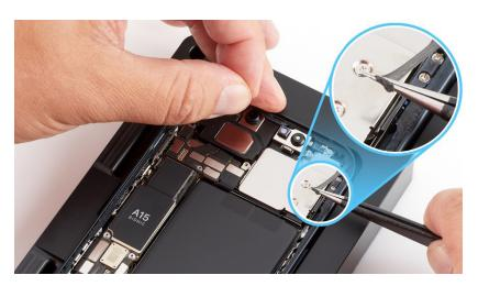
32. Use ESD-safe tweezers to remove the grounding foam from the top of the enclosure as shown.
