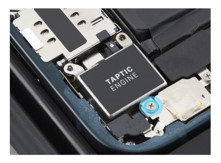
5. Lift the end of the Taptic Engine flex cable off the connector.
