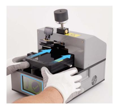
**Note:** The screen on the fixture will turn red and the timer will count down from 2 minutes while the pocket heats to the correct temperature. When the timer ends, the display will show 0, the fixture will start to beep, and the screen will be green.
