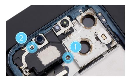
8. Position the logic board and the mmWave antenna in the enclosure as shown.
