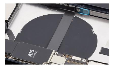
5. Lift the ends of the 13 flex cables off the connectors on the logic board.
