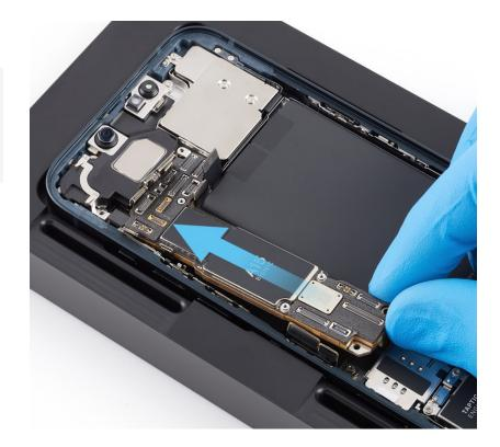
9. Press the ends of the 12 flex cables to the connectors in the order shown.
