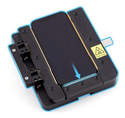
4. Flip down the clamp on the side of the pocket to lock the iPhone into place.
