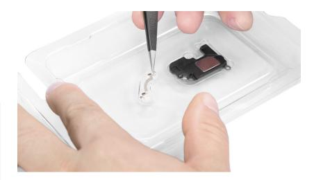
2. Use ESD-safe tweezers to remove the release liners from the underside of the grounding strap. Then use the tweezers to position the grounding strap on top of the speaker.
