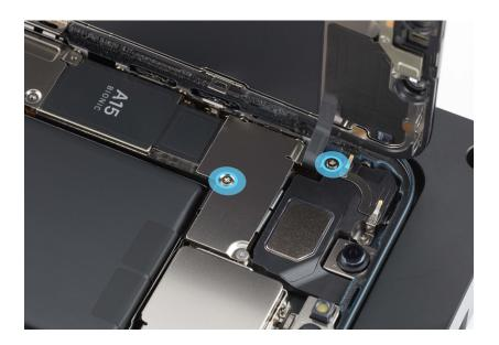
24. Hold the upper cowling in place. Use a torque driver and the Micro stix bit to remove the trilobe screw from the upper cowling. Set aside the screw.
