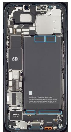
3. Hold down the iPhone. Use ESD-safe tweezers to continue peeling the bottom right battery adhesive tab from the battery.
