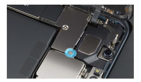
25. Use ESD-safe tweezers to tilt up the upper cowling (1). Then slide the cowling out from under the ambient light sensor flex cable (2). Save the cowling for reassembly.
