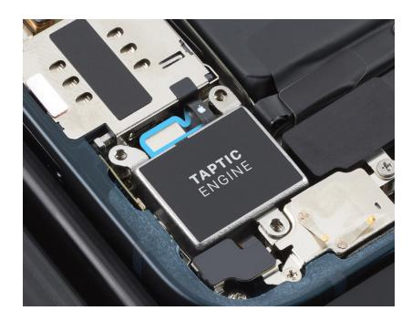
6. Use ESD-safe tweezers to remove the Taptic Engine.
