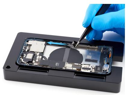
3. Use a torque driver and the JCIS bit to remove the three crosshead screws from the mmWave antenna connector cowling. Remove the cowling and save it for reassembly. Set aside the screws.
