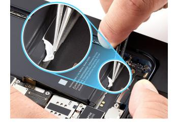
Note: The battery has four adhesive tabs.
