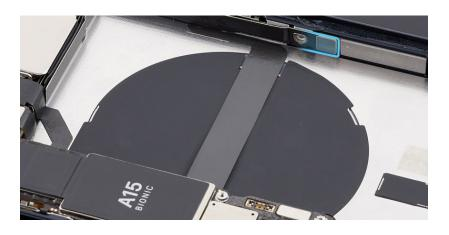
10. Press the ends of the 11 flex cables to the connectors in the order shown.
