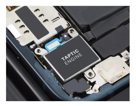
3. Use the blue torque driver and JCIS bit to install one new crosshead screw (923-07003) into the Taptic Engine.
