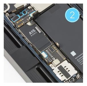
3. Use a torque driver and the JCIS bit to remove the crosshead screw from the lower end of the logic board. Set aside the screw.
