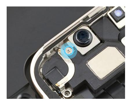
6. Position the logic board and the mmWave antenna in the enclosure as shown.
