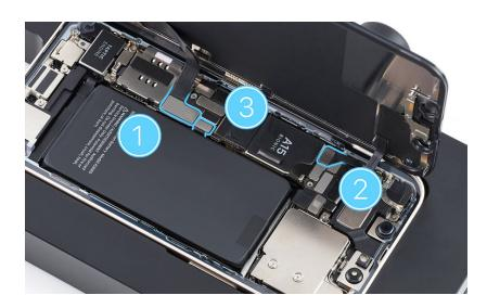
Use ESD-safe tweezers to position the lower cowling over the ends of the display and battery flex cables.
