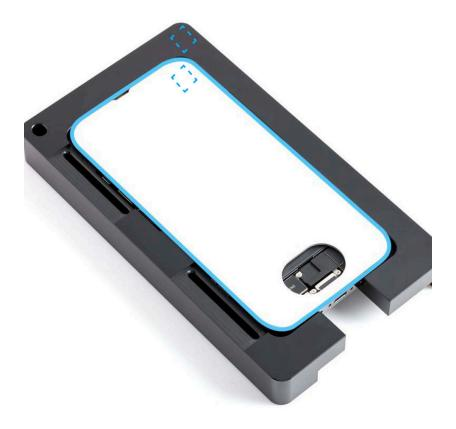
8. Position the repair tray with the iPhone in the display press. Pull down the lever until the display press locks.
