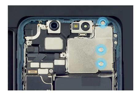
3. Use ESD-safe tweezers to tilt up the right edge of the camera cowling (1). Then pull the cowling to the right to release the tabs on the left (2). Save the cowling for reassembly.
