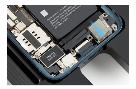
3. Use the gray torque driver and JCIS bit to install four new crosshead screws (923-06670) (1) (923-06671) (2) into the bottom speaker. Press the bottom speaker down as you install the screws.
