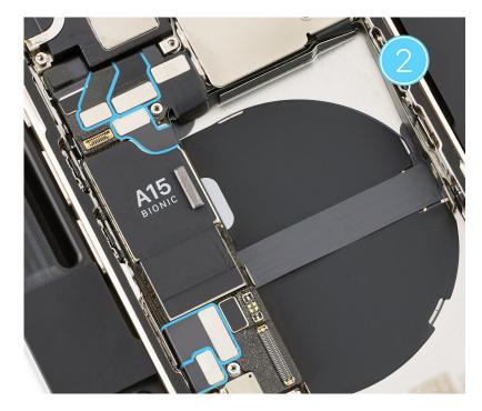
9. Use the blue torque driver and super screw bit to install one new super screw (923-06673) into the logic board.
