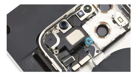
5. Use the gray torque driver and JCIS bit to install one new crosshead screw (923-06676) into the top speaker.
