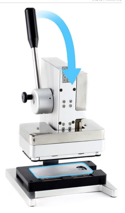
9. Wait until the timer on the display press beeps and the timer shows 0. Pull down the lever (1) and pull out the release knob (2). Then lift the lever (3).
