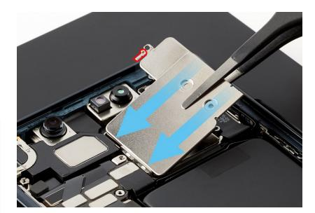
7. Use the blue torque driver and JCIS bit to install three new crosshead screws (923-06660) into the camera cowling in the order shown.
