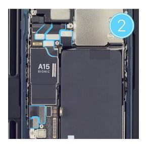
8. Use the blue torque driver and super screw bit to install one new super screw (923-06673) into the logic board.
