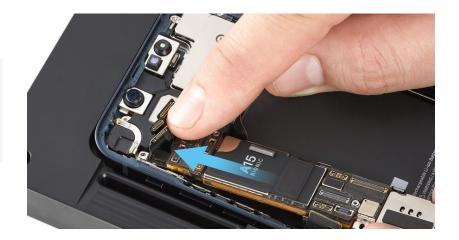
7. Press the ends of the 11 flex cables to the connectors on the logic board in the order shown.
