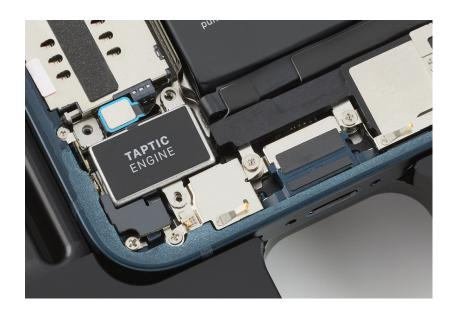
7. Use ESD-safe tweezers to remove the Taptic Engine.
