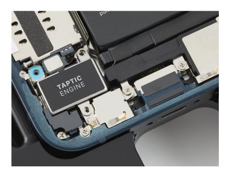
4. Use the gray torque driver and JCIS bit to install one new crosshead screw (923-06667) into the Taptic Engine.
