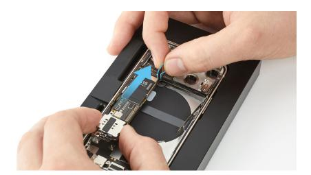
7. Follow <u>camera</u> reassembly steps 1 through 7 to reinstall the camera in the enclosure. Then continue to step 8 on the next page.
