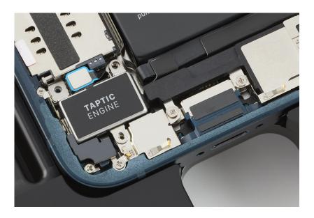
3. Use the blue torque driver and super screw bit to install one new super screw (923-06669) into the Taptic Engine.
