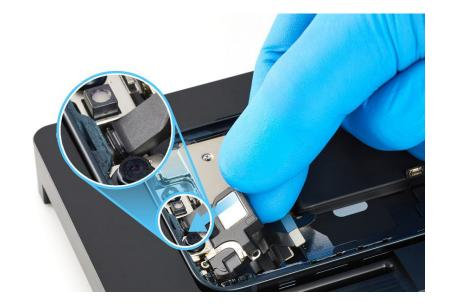
4. Use the blue torque driver and super screw bit to install one new super screw (923-06675) into the top speaker.
