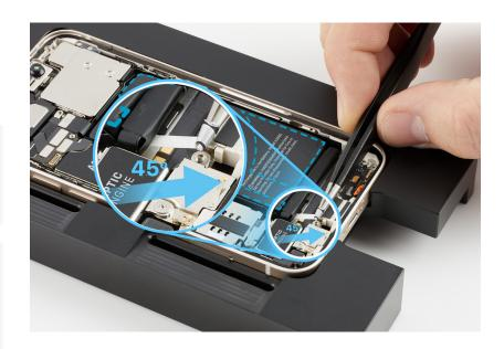
6. Use ESD-safe tweezers to grasp the bottom right battery adhesive tab and gently peel it away from the battery.
