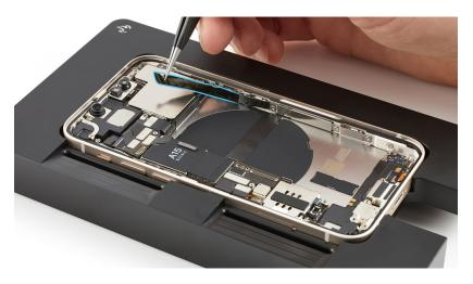
3. Use a torque driver and the JCIS bit to remove the three crosshead screws from the mmWave antenna connector cowling in the order shown. Set aside the screws. Remove the cowling and save it for reassembly.
