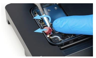
6. Inspect the TrueDepth camera assembly. Ensure that the top edge of the camera assembly is under the lip of the enclosure.
