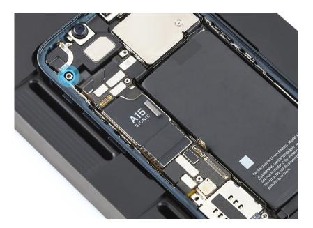
9. Use the gray torque driver and JCIS bit to install one new crosshead screw (923-06676) in the logic board.
