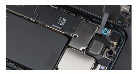
25. Use ESD-safe tweezers to tilt up the upper cowling (1). Then slide the cowling out from under the ambient light sensor flex cable (2). Save the cowling for reassembly.
