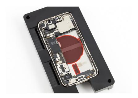
14. Insert the flat end of the black stick only into one of the insertion points as shown. Ensure that the black stick is inserted into a point where the battery adhesive strip has been fully removed. Don't insert the black stick into a point where the battery tab or adhesive strip is broken.
