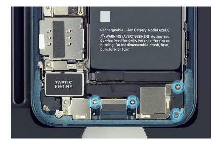
3. Remove the bottom speaker from the enclosure.
