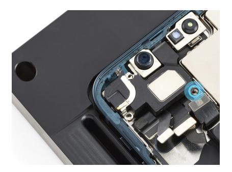
5. Use the gray torque driver and JCIS bit to install one new crosshead screw (923-06676) into the top speaker.
