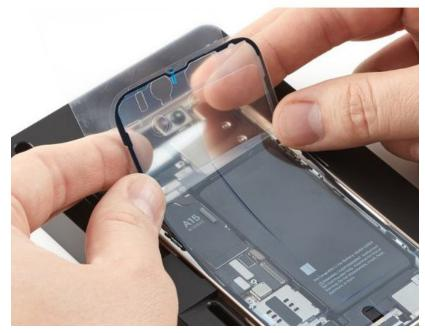
6. Use the flat end of the black stick to lightly press the grounding foam to adhere it as shown.
