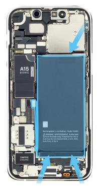
15. Slightly lift the battery with the black stick just enough to grasp underneath the battery.
