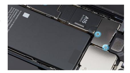
24. Use a torque driver and the JCIS bit to remove the crosshead screw from the upper cowling. Set aside the screw.
