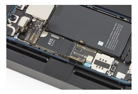
4. Use a torque driver and the super screw bit to remove the super screw from the upper end of the logic board. Set aside the screw.
