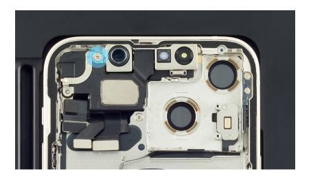
17. Use a torque driver and the super screw bit to remove one super screw from the top speaker. Set aside the screw.
