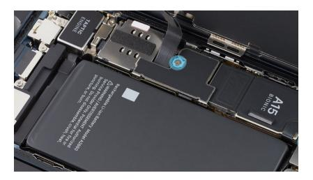
22. Use ESD-safe tweezers to tilt up the lower cowling to release two cowling tabs from the slots on the logic board. Remove the lower cowling and save it for reassembly.
