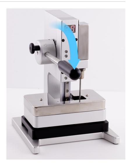
28. Wait until the timer on the display press beeps and the timer shows 0. Pull down the lever (1) and pull out the release knob (2). Then lift the lever (3).
