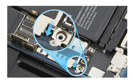
15. Gently lift the mmWave antenna and the logic board up and out of the enclosure.
