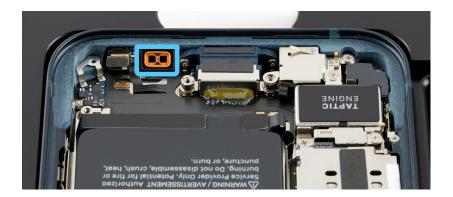
2. Rotate the repair tray. Align the port on the bottom speaker with the hole in the enclosure. Then lower the bottom speaker into position.
