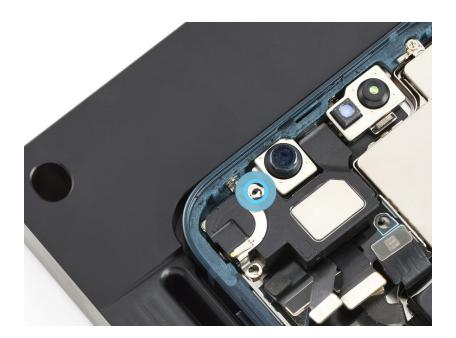
6. Tilt the logic board and lower it into position.
