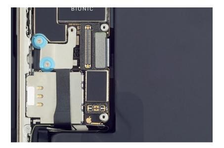
6. Use ESD-safe tweezers to remove the logic board cowling. Save the cowling for reassembly.
