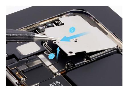
5. Use a torque driver and the Micro stix bit to remove the two trilobe screws from the logic board cowling. Set aside the screws.
