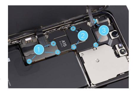
25. Use ESD-safe tweezers to tilt up the upper cowling. Then slide the cowling out from under the ambient light sensor flex cable. Save the cowling for reassembly.
