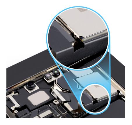
3. Press the ends of the two camera flex cables to the connectors.
