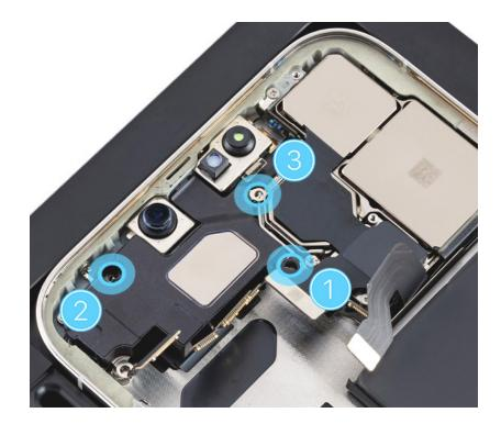
6. Use ESD-safe tweezers to position the grounding strap on the top speaker.
