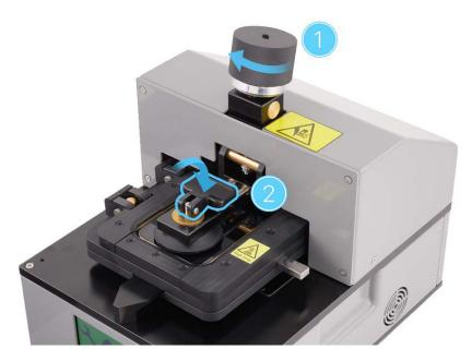
Slowly turn the knob on the fixture counterclockwise until the display begins to separate from the enclosure.
