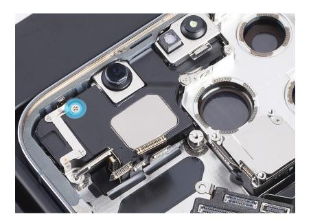
20. Use ESD-safe tweezers to remove the grounding strap from the top speaker.
