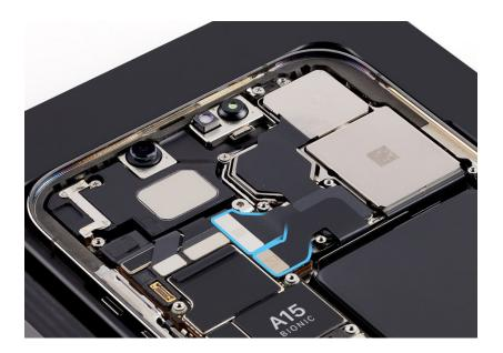
6. Gently hold the camera flex cables together and lift the cameras out of the enclosure.
