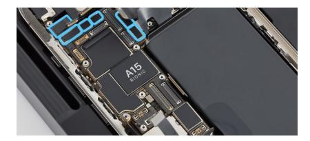
8. Use a torque driver and the super screw bit to remove the two super screws from the logic board. Set aside the screws.
