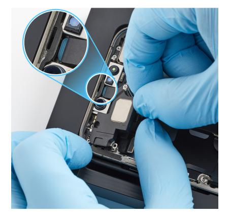
3. Inspect the TrueDepth camera. Ensure that the top edge of the TrueDepth camera is under the lip of the enclosure.
