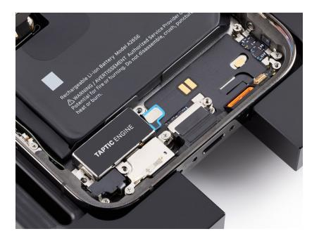
5. Remove the Taptic Engine from the enclosure.
