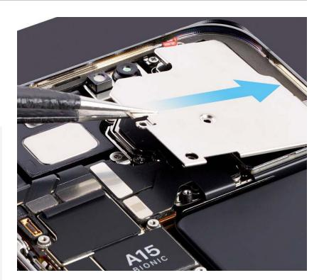
14. Hold down the camera cowling. Then use the black torque driver and Micro stix bit to install one new trilobe screw (923-06266) into the middle of the cowling.
