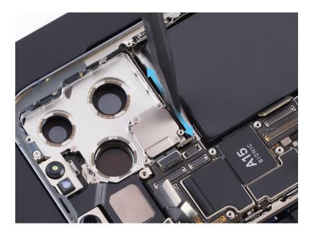
17. Place the battery protective cover on top of the battery.
