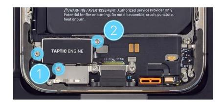
4. Lift the end of the Taptic Engine flex cable off the connector.
