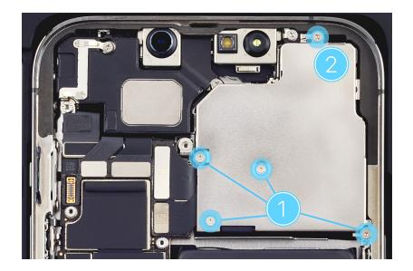
4. Use ESD-safe tweezers to tilt up the left side of the camera cowling (1). Then slide the cowling tabs out of the slots on the right side of the enclosure (2). Save the cowling for reassembly.
