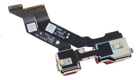
3. Tilt the top edge of the TrueDepth camera assembly under the lip of the enclosure as shown. Then lower the camera into the enclosure. Use your finger or the black stick to adjust the alignment.
