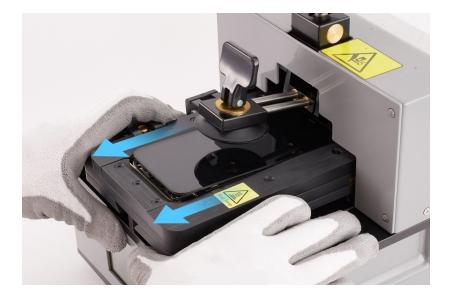
15. Flip up the clamp on the side of the pocket to release the iPhone (1). Hold the area outlined in blue and gently remove the iPhone from the pocket (2).
