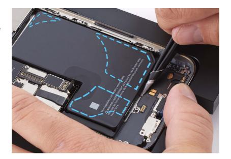
4. Keep the tweezers close and parallel to the battery and twist until you see white adhesive strip on the tweezers.
