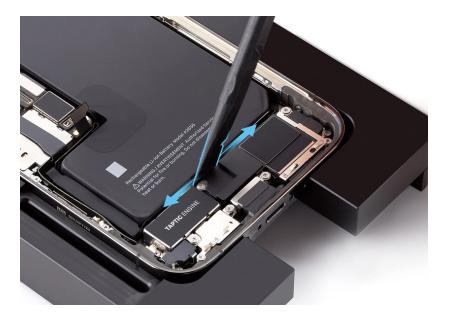
3. Use a torque driver and the JCIS bit to remove the four crosshead screws from the bottom speaker. Set aside the screws.
