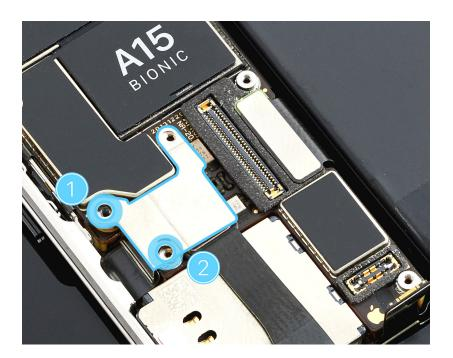
13. The camera cowling has tabs that fit into slots on the right side of the enclosure. Hold the cowling with ESD-safe tweezers and slide the cowling tabs into the slots. Then lower the cowling onto the cameras.
