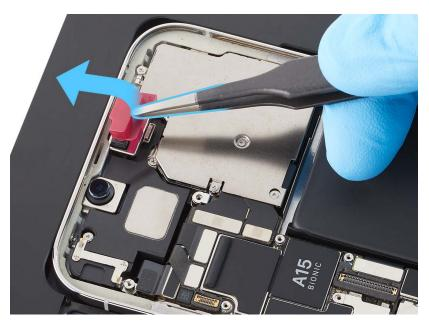
6. Inspect the TrueDepth camera assembly. Ensure that the top edge of the camera assembly is under the lip of the enclosure and centered between the sides of the enclosure.
