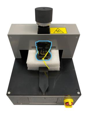
3. Turn the top knob on the fixture counterclockwise to raise the suction cup. Remove the packing foam.
