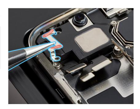
7. Use the green torque driver and JCIS bit to install one new crosshead screw (923-06273) into the grounding strap.
