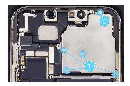
4. Use ESD-safe tweezers to tilt up the camera cowling from the left side (1). Then slide the cowling tabs out of the slots on the right side of the enclosure (2). Save the cowling for reassembly.
