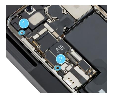
12. Position the logic board cowling. Then use the black torque driver and Micro stix bit to install two new trilobe screws (923-06284) (1) (923-06286) (2) into the logic board cowling.
