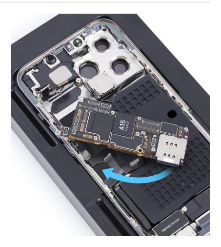
9. Remove the battery protective cover.
