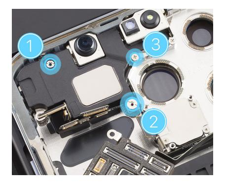
6. Use ESD-safe tweezers to position the grounding strap on the top speaker.
