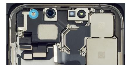
8. Position the logic board in the enclosure.
