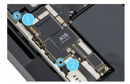
14. Position the logic board cowling. Then use the black torque driver and Micro stix bit to install two new trilobe screws (923-06284) (1) (923-06286) (2) into the logic board cowling.
