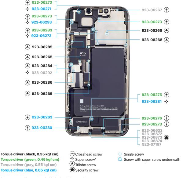
\*A super screw has a threaded hole that holds another screw.
