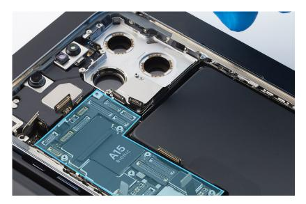
9. Press the ends of the 11 flex cables to the connectors in the order shown.
