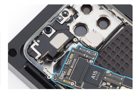
19. Use a torque driver and the JCIS bit to remove the crosshead screw from the grounding strap on the top speaker. Set aside the screw.
