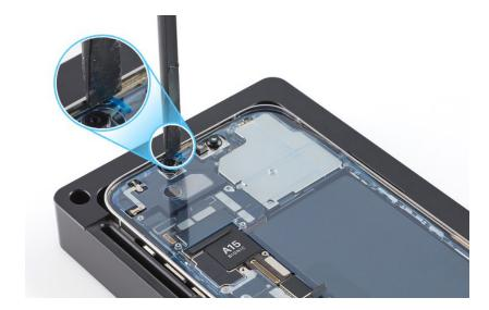
7. Place the display adhesive press plate on top of the enclosure with the icon in the top right corner as shown.
