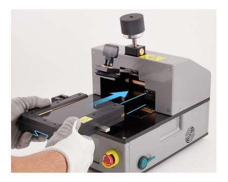
6. Slide the pocket into the fixture until the pocket clicks into place.
