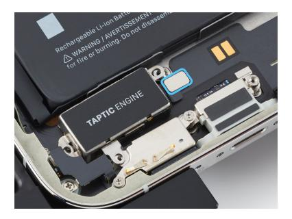
5. Use ESD-safe tweezers to remove the Taptic Engine with the battery shim attached from the enclosure.
