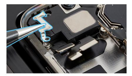
7. Use the green torque driver and the JCIS bit to install one new crosshead screw (923-06269) into the grounding strap.
