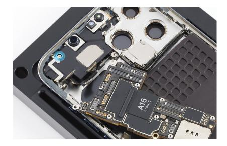
8. Carefully rotate the logic board back over the enclosure and remove the battery protective cover. Lower the logic board into the enclosure.
