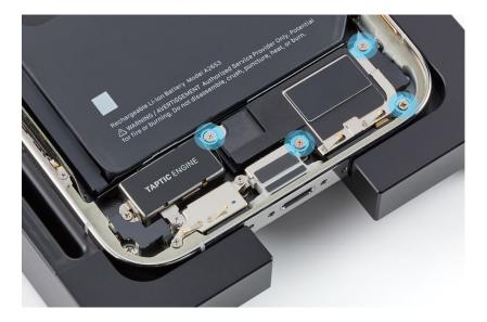
3. Use ESD-safe tweezers to grasp the lower left screw hole and peel the bottom speaker away from the battery shim. Then remove the bottom speaker from the enclosure.
