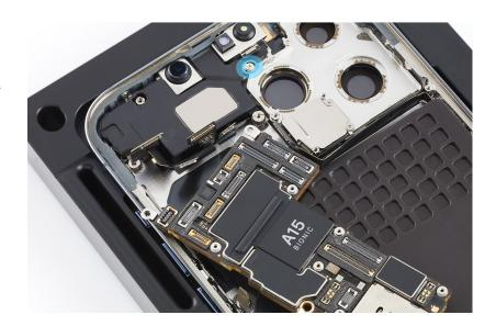
6. Use ESD-safe tweezers to position the grounding strap on the top speaker.
