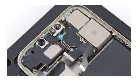
6. Use ESD-safe tweezers to position the grounding strap on the top speaker.
