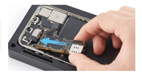
9. Press the ends the 12 flex cables to the connectors on the logic board in the order shown.
