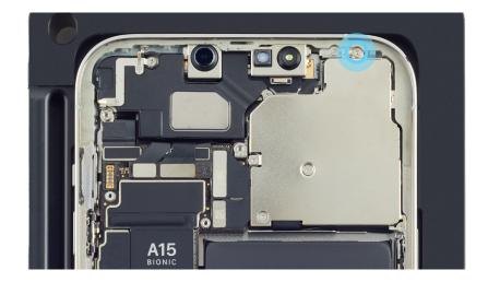
4. Use ESD-safe tweezers to tilt up the camera cowling from the left side (1). Then slide the cowling tabs out of the slots on the right side of the enclosure (2). Save the cowling for reassembly.
