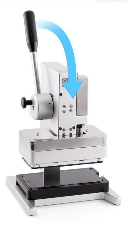
28. Wait until the display press beeps and the timer shows 0. Pull down the lever (1) and pull out the release knob (2). Then lift the lever (3).
