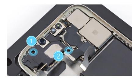
5. Use the green torque driver and JCIS bit to install one new crosshead screw (923-06269) into the top speaker.
