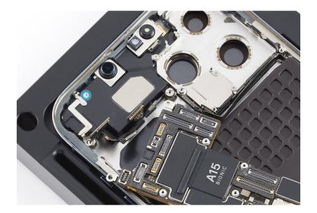
20. Use ESD-safe tweezers to remove the grounding strap.
