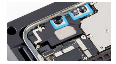
4. Align the replacement display adhesive over the enclosure with the grounding foam on top and the bottom tab on the right.
