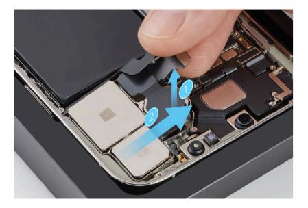
11. Use the black stick to break the adhesive between the mmWave antenna flex cable and the camera well.
