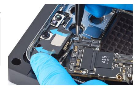
4. Use the blue torque driver and super screw bit to install two new super screws (923-06271) (1) (923-06653) (2) into the top speaker.
