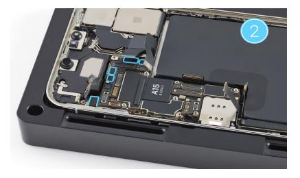
8. Use a torque driver and super screw bit to remove the two super screws from the logic board. Set aside the screws.
