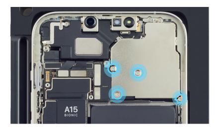
3. Use a torque driver and the JCIS bit to remove the crosshead screw from the camera cowling. Set aside the screw.
