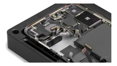
4. Use the blue torque driver and super screw bit to install two new super screws (923-06271) (1) (923-06653) (2) into the top speaker.
