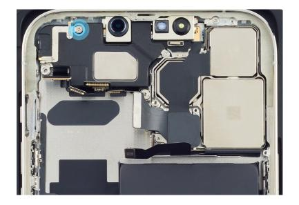
16. Use ESD-safe tweezers to remove the grounding strap from the top speaker.
