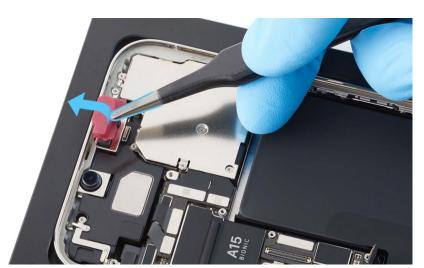
6. Inspect the TrueDepth camera assembly. Ensure that the top edge of the camera assembly is under the lip of the enclosure and centered between the sides of the enclosure.
