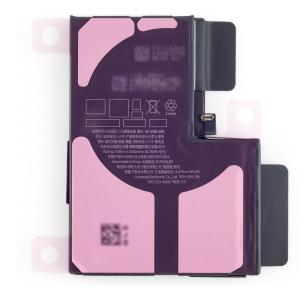
5. Hold the battery over the enclosure with the protective cover faceup. Align the bottom of the battery with the Taptic Engine (1) and the left edge with the logic board (2). Then lower the battery into the enclosure.
