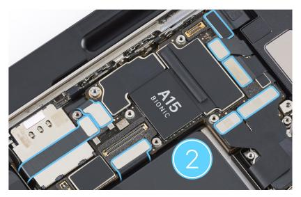
10. Use the gray torque driver and super screw bit to install two new super screws (923-06292) (1), (923-06293) (2) into the logic board.
