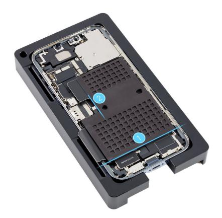
6. The center of the repair tray has two slots. Position the repair tray and enclosure onto the battery press with the left slot over the pin as shown.
