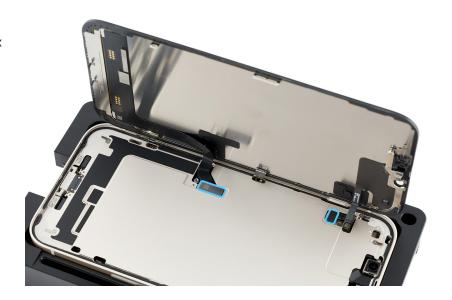
29. Hold the display by the edges. Pull the tabs on the suction cups to release them from the display. Then set the display facedown on a clean, flat surface.
