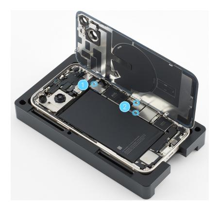
23. Use ESD-safe tweezers to remove the lower cowling. Save the cowling for reassembly.
