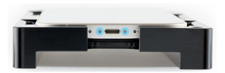
7. Flip the switch on the back of the heated display removal fixture to turn it on. The internal fan will turn on. Wait for a checkmark to appear on the screen.
