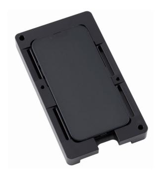
23. Position the repair tray with the iPhone display faceup in the display press. Pull down the lever until the display press locks.
