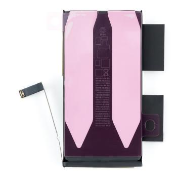
3. Hold the battery over the enclosure with the protective cover faceup. Align the top of the battery with the camera sidewall (1) and the right edge with the logic board (2). Then lower the battery into the enclosure.
