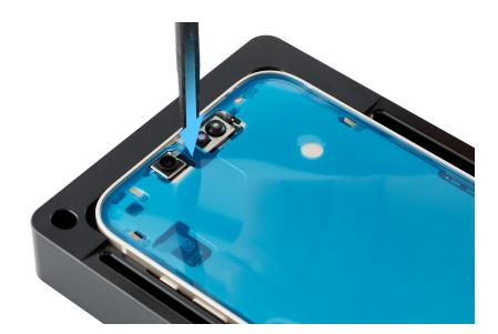
7. Place the display adhesive press plate on top of the enclosure with the icon in the top right corner as shown.
