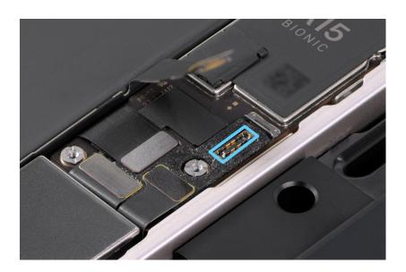
4. Press the end of the back glass flex cable to the connector.
