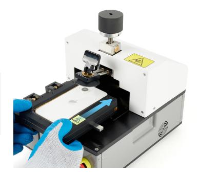
7. Slide the pocket into the fixture until the pocket clicks into place.
