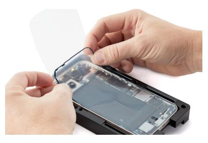
5. Inspect the back glass adhesive to ensure that it's positioned on the shelf of the enclosure. If the adhesive isn't correctly positioned on the enclosure, repeat removal steps 28 and 29. Then repeat reassembly steps 1 through 5.
