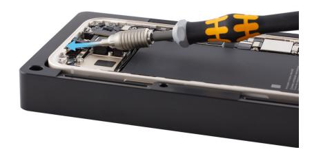
3. Use a torque driver and the JCIS bit to remove the seven crosshead screws from the top speaker. Set aside the screws.
