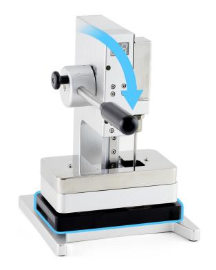
23. Wait until the display press beeps and the timer shows 0. Pull down the lever (1) and pull out the release knob (2). Then lift the lever (3).
