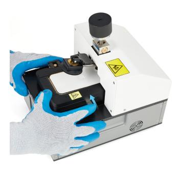
15. Hold both sides of the pocket and slide it straight out of the fixture.
