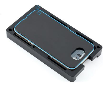
7. Position the repair tray with the iPhone in the display press. Pull down the lever until the display press locks.
