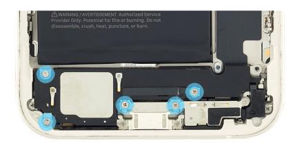
3. Use a torque driver and the Micro stix bit to remove the trilobe screw from the bottom speaker. Set aside the screw.
