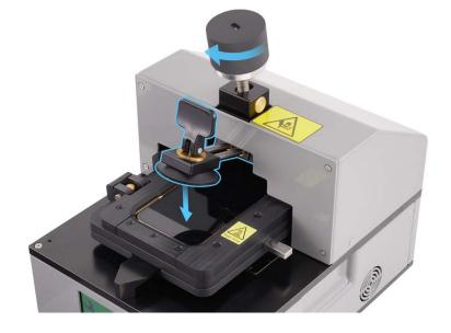
13. Grasp the handle and slide the suction cup straight out until the edge of the suction cup aligns with the bottom edge of the display.
