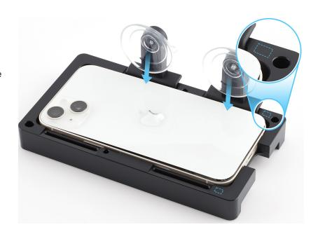
21. Tilt up the back glass toward the suction cups. Press the top and bottom edges of the back glass to secure it to the suction cups.
