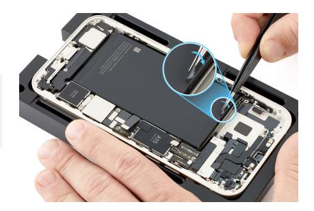
**Note:** The battery has two adhesive tabs.
