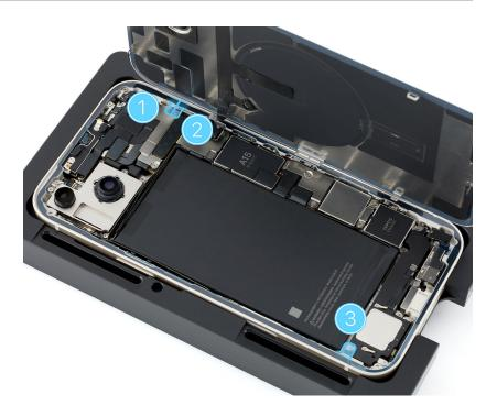
17. Inspect the back glass adhesive to ensure that it's in the correct position and not damaged or wrinkled. If the adhesive is damaged, remove it and apply replacement adhesive.
