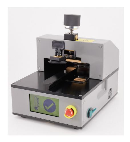
8. Take the iPhone out of the repair tray. Then gently insert the iPhone into the heated display pocket with the display faceup and the Lightning connector facing the bottom of the pocket.
