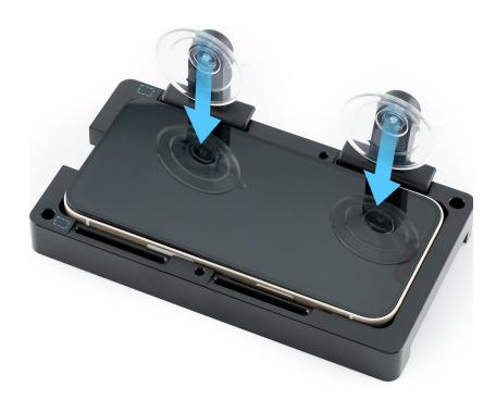
25. Tilt up the display toward the suction cups. Press the top and bottom edges of the display to secure it to the suction cups.
