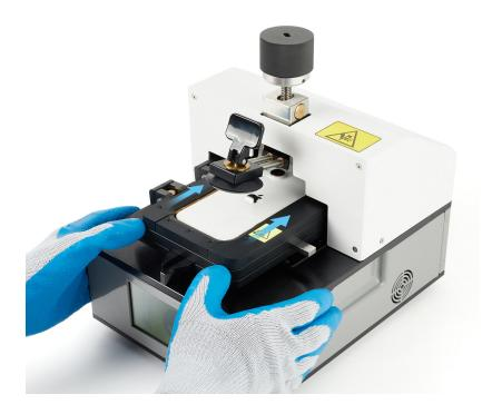
**Note:** The screen on the fixture will turn red and the timer will count down from 2 minutes while the pocket heats to the correct temperature. When the timer shows 0, the fixture will start to beep and the screen will turn green.
