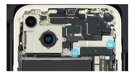
4. Remove the TrueDepth camera connector cowling and save it for reassembly.
