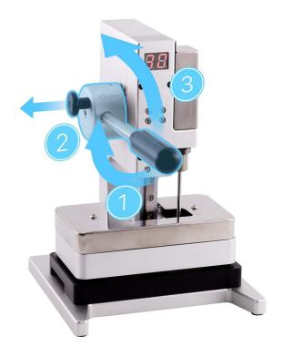
24. Remove the repair tray from the display press.
