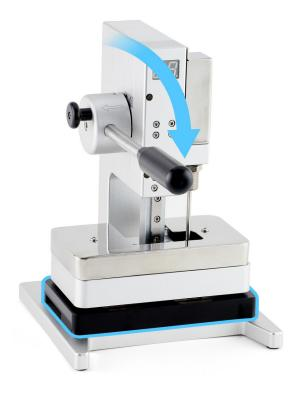
24. Wait until the display press beeps and the timer shows 0. Pull down the lever (1) and pull out the release knob (2). Then lift the lever (3).
