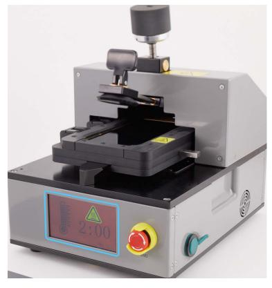
12. Turn the knob on the fixture clockwise to lower the suction cup as close to the iPhone as possible without touching the iPhone.
