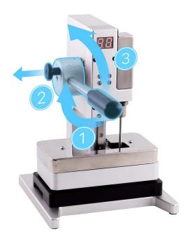
25. Remove the repair tray from the display press.
