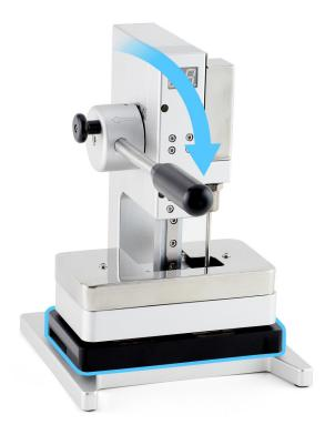
9. Wait until the display press beeps and the timer shows 0. Pull down the lever (1) and pull out the release knob (2). Then lift the lever (3).
