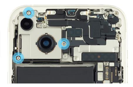
4. Lift the ends of the two camera flex cables from the connectors (1).
