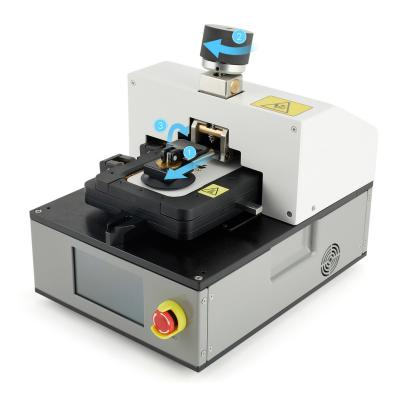
11. Slowly turn the knob on the fixture counterclockwise until the back glass begins to separate from the enclosure.
