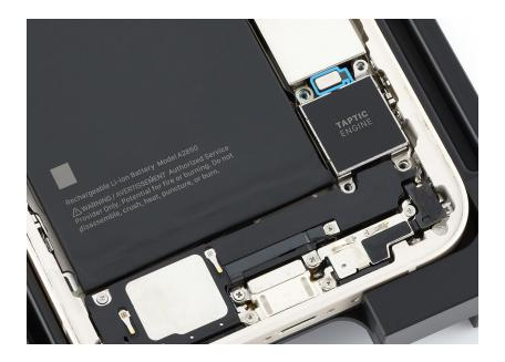
7. Remove the Taptic Engine from the enclosure.
