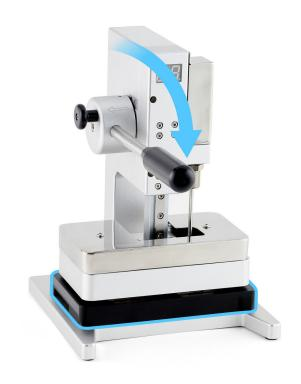
8. Wait until the display press beeps and the timer shows 0. Pull down the lever (1) and pull out the release knob (2). Then lift the lever (3).
