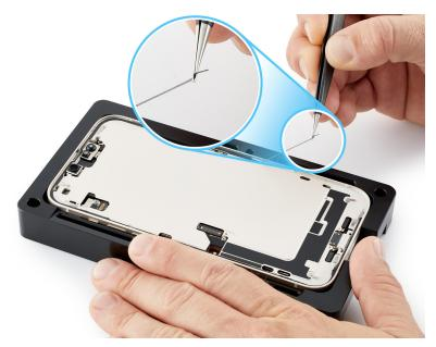
32. Use ESD-safe tweezers to remove the grounding foam from the top of the enclosure as shown.
