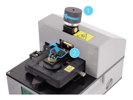
15. Slowly turn the knob on the fixture counterclockwise until the display begins to separate from the enclosure.
