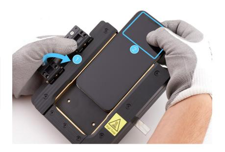
21. Place the iPhone into the repair tray with the display faceup and the Lightning connector facing the cutout. Remove the gloves.
