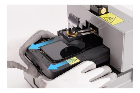
20. Flip up the clamp on the side of the pocket to release the iPhone (1). Hold the area outlined in blue and gently remove the iPhone from the pocket (2).
