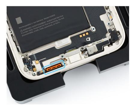
2. Position the bottom speaker in the enclosure. Slide the bottom right screw hole of the bottom speaker under the vent cowling screw hole as shown.
