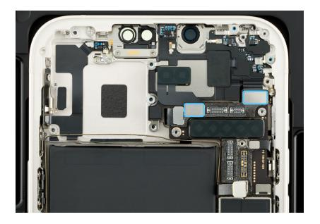
3. Use the gray torque driver and JCIS bit to install one new crosshead screw (923-08504) into the sidewall of the enclosure. Keep the torque driver as perpendicular as possible to avoid stripping the screw.
