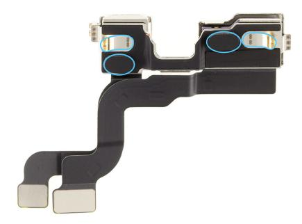
3. Use ESD-safe tweezers to remove the protective cover from the TrueDepth camera.
