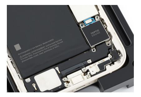
3. Use the teal torque driver and super screw bit to install one new super screw (923-08507) into the Taptic Engine.
