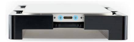
3. Flip the switch on the back of the heated display removal fixture to turn it on. The internal fan will turn on. Wait for a checkmark to appear on the screen.
