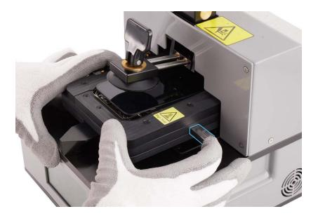
19. Hold both sides of the pocket and slide it straight out of the fixture.
