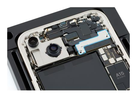
5. Lift the ends of the two TrueDepth camera flex cables off the connectors.
