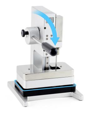
30. Wait until the display press beeps and the timer shows 0. Pull down the lever (1) and pull out the release knob (2). Then lift the lever (3).
