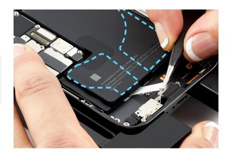
5. Pull the tweezers toward the Lightning connector at the bottom of the iPhone and continue to twist the adhesive until you've removed the entire strip.
