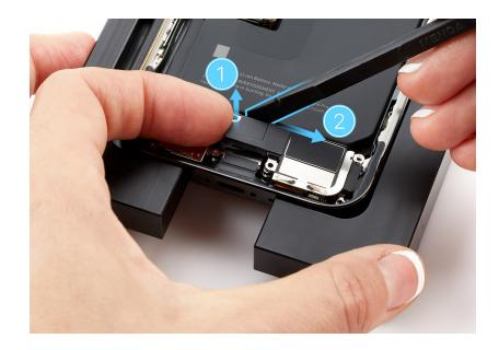
4. Remove the bottom speaker from the enclosure.
