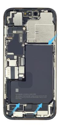
14. Slightly lift the battery with the black stick just enough to grasp underneath the battery.
