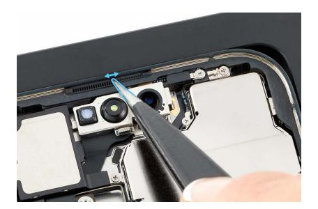
9. Align the replacement display adhesive over the enclosure. Ensure that the top holes of the adhesive align over the TrueDepth camera assembly.
