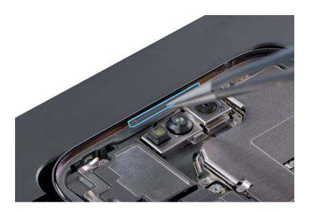
8. Position the tip of the ESD-safe tweezers in the middle of the top speaker grille. Slightly move the tweezers from side to side to ensure that the speaker grille is firmly adhered to the enclosure and doesn't move.
