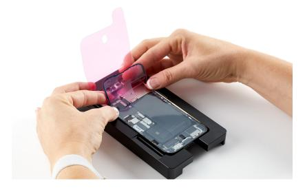
11. Inspect the adhesive to ensure that it's positioned on the lip of the enclosure. If the adhesive isn't correctly positioned, repeat removal steps 29 and 30. Then repeat reassembly steps 1 through 10.
