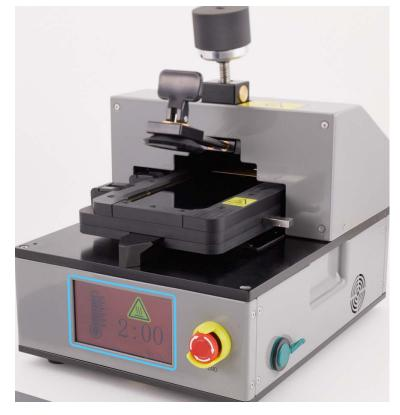
8. Turn the knob on the fixture clockwise to lower the suction cup as close to the iPhone as possible without touching the iPhone.
