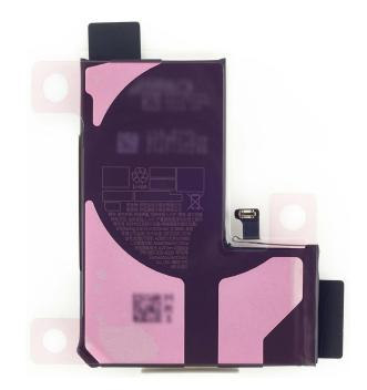
5. Hold the battery over the enclosure with the protective cover faceup. Align the bottom of the battery with the bottom speaker (1) and the right edge with the enclosure (2). Then lower the battery into the enclosure.
