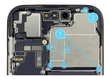
5. Use ESD-safe tweezers to tilt up the camera cowling from the left side (1). Then slide the cowling tab out of the slot on the right side of the enclosure (2). Save the cowling for reassembly.
