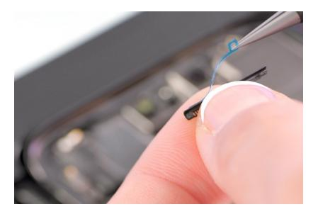
7. Position the replacement top speaker grille in the cutout on the lip of the enclosure. Ensure that the adhesive side of the speaker grille faces the side of the enclosure.
