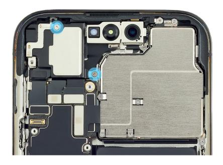
4. Use the black stick to tilt up the top speaker as shown. Then lift the top speaker out of the enclosure.
