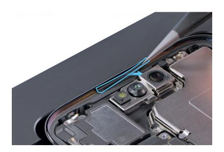
6. Use ESD-safe tweezers to peel the adhesive liner off the back of the replacement top speaker grille.
