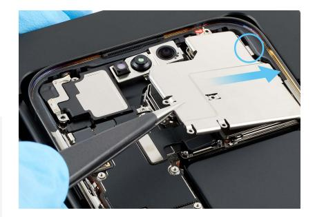
7. Use the black torque driver and Micro stix bit to install four new trilobe screws (923-08160) (1) into the camera cowling.
