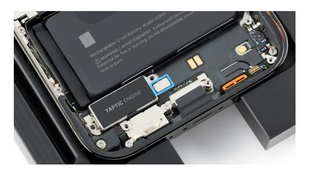
4. Use the blue torque driver and super screw bit to install one new super screw (923-08151) into the Taptic Engine.
