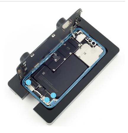
24. Inspect the display adhesive to ensure that it's in the correct position and isn't damaged or wrinkled. If the adhesive is damaged, remove it and apply replacement adhesive.
