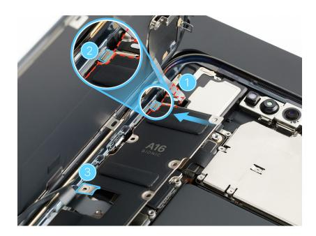
22. Use the green torque driver and Micro stix bit to install the following eight new trilobe screws into the logic board:
