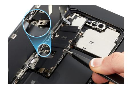
24. Use ESD-safe tweezers to slide the logic board cowling out from under the ambient light sensor flex cable (1). Then lift the cowling out of the enclosure (2). Save the cowling for reassembly.
