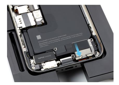
3. Use the gray torque driver and JCIS bit to install four new crosshead screws (923-08147) (1) (923-08377) (2) into the bottom speaker.
