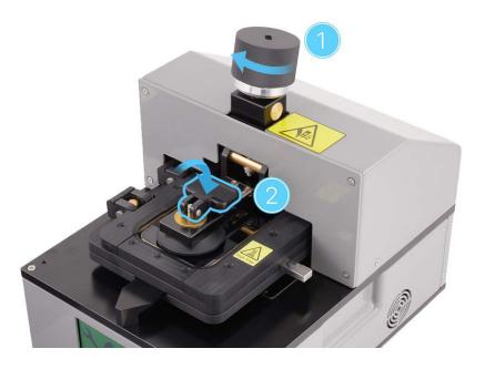
11. Slowly turn the knob on the fixture counterclockwise until the display begins to separate from the enclosure.
