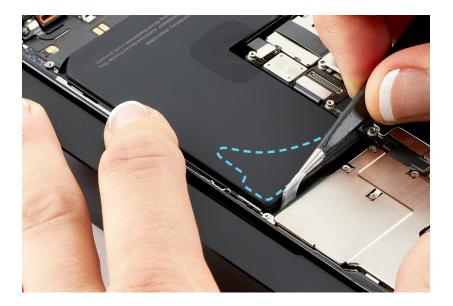
12. If all three battery adhesive strips were fully removed, continue to step 14. If at least one strip was fully removed, continue to step 13.
