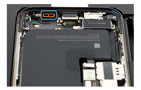
2. Rotate the repair tray. Align the port on the bottom speaker with the rubber gasket. Then position the bottom speaker in the enclosure.
