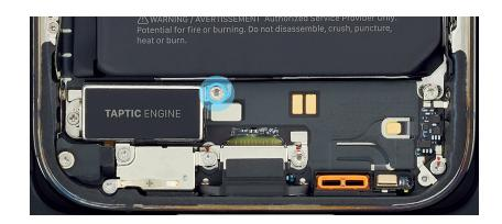
3. Use a torque driver and the JCIS bit to remove the two crosshead screws from the Taptic Engine. Set aside the screws.
