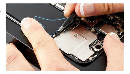
11. Keep the tweezers close to the channel between the battery and the camera cowling. Continue to slowly twist the tweezers until you've removed the entire adhesive strip.
