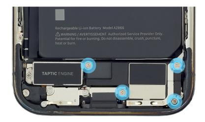
3. Slightly tilt up the bottom speaker as shown (1). Run the flat end of the black stick between the battery shim and the Taptic Engine and bottom speaker to loosen the adhesive on the battery shim (2).
