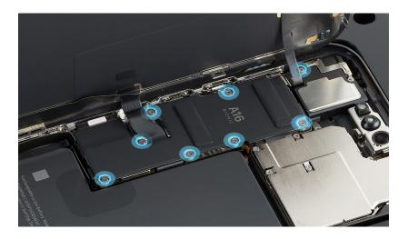
23. Use ESD-safe tweezers to slightly lift the logic board cowling. Ensure that the bottom tab on the logic board cowling clears the display flex cable as you lift it.
