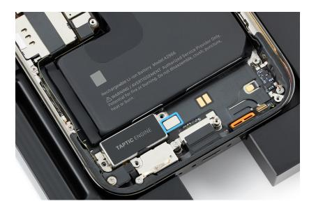
5. Remove the Taptic Engine and battery shim from the enclosure.
