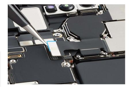
7. Position the ESD-safe tweezers under the bottom left corner of the bottom camera flex cable as shown. Then gently lift the end of the bottom camera flex cable off the connector.
