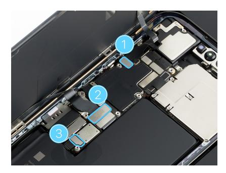
21. Use ESD-safe tweezers to slide the top tab of the logic board cowling behind the ambient light sensor flex cable (1). Then slide the edge of the cowling under the tab on the side of the enclosure (2) and slide the bottom tab behind the display flex cable (3). Lower the cowling over the ends of the flex cables.
