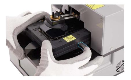
15. Hold both sides of the pocket and slide it straight out of the fixture.
