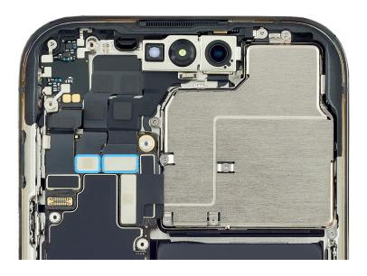
4. Gently hold the TrueDepth camera flex cables together and lift the TrueDepth camera out of the enclosure.
