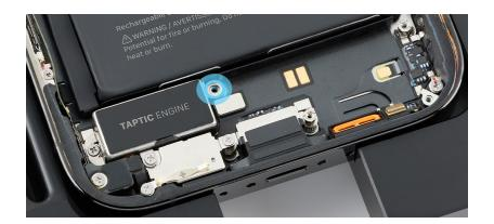
5. Use the teal torque driver and JCIS bit to install two new crosshead screws (923-08149) (1) (923-08374) (2) into the Taptic Engine.
