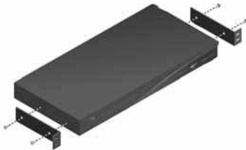
Figure 2.3: AMX Switch Rack Mounting Diagram
