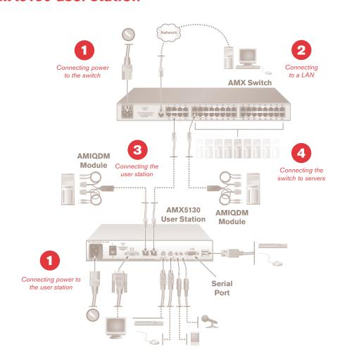
AMIQDM (dual port/multimedia) module. Plug the AMIQDM module connectors into the appropriately labeled ports on your server for each computer to be connected to your AMX switch.
