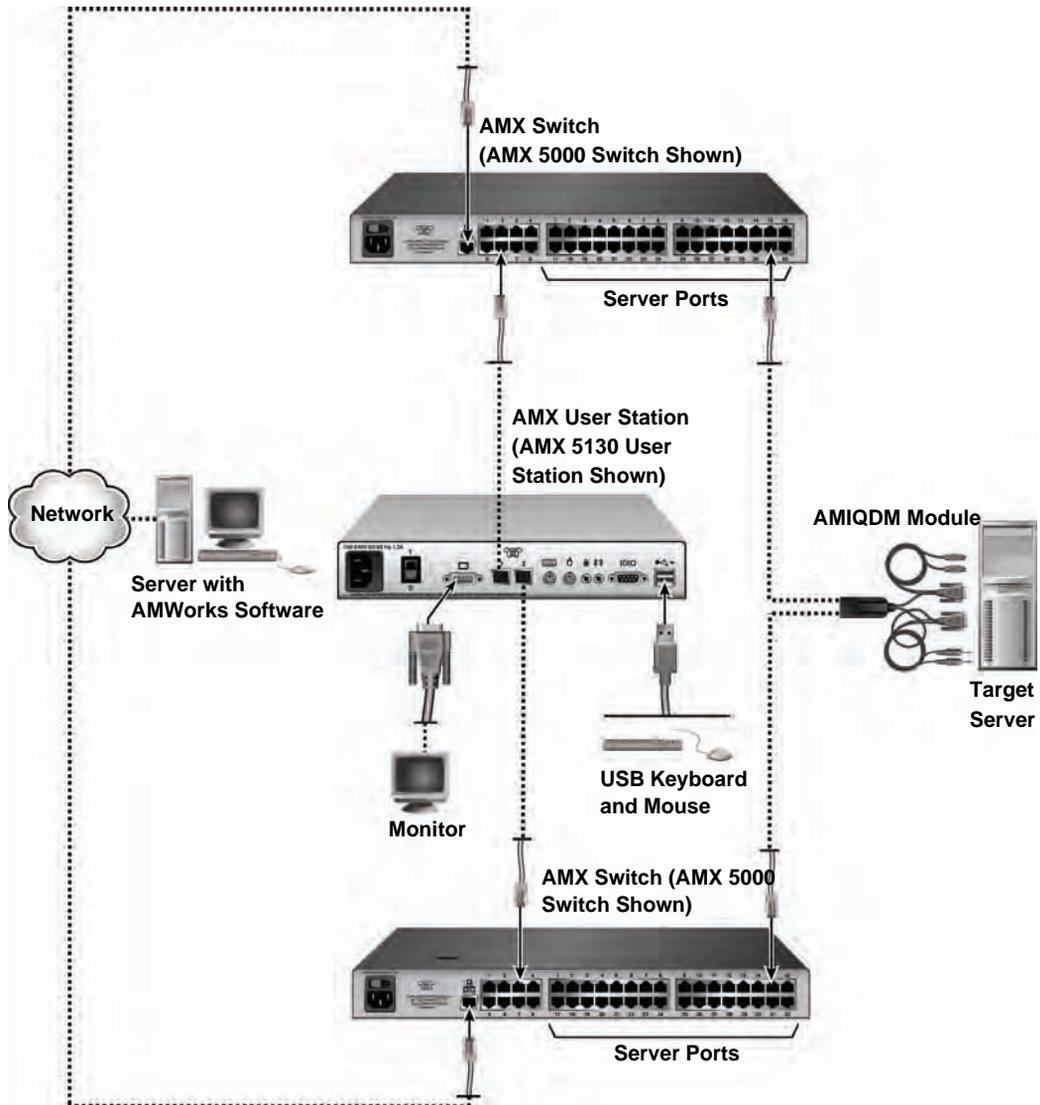
Figure 2.4: AMX Switching System Configuration with Redundancy
