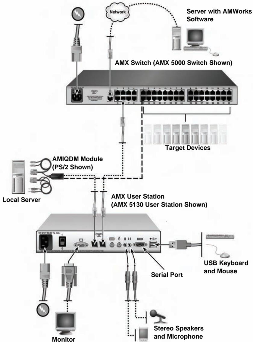
Figure 2.3: AMX Switching System Configuration with AMIQDM Modules
