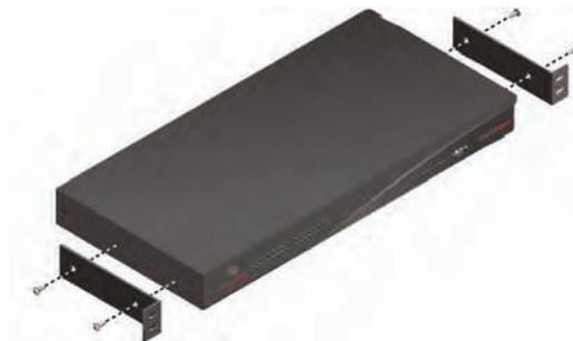
Figure 2.5: AMX Switch Rack Mounting Diagram
