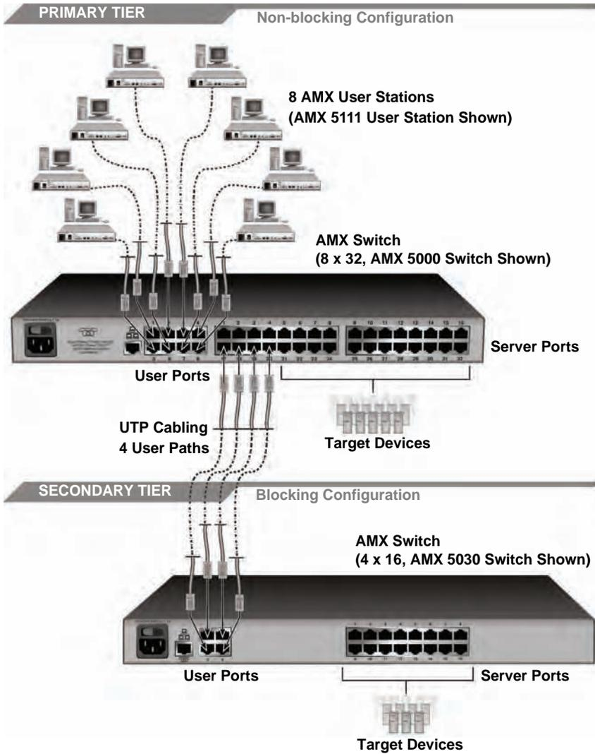
Figure 2.11: Cascaded AMX Switching System, Blocking Configuration
