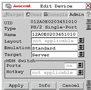
**Figure 3.27: Edit Device Screen (Normal Configuration)**
