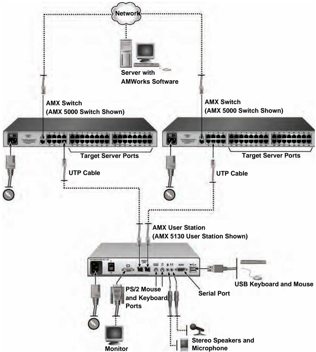
Figure 2.9: Connecting a User Station for Switch Redundancy
