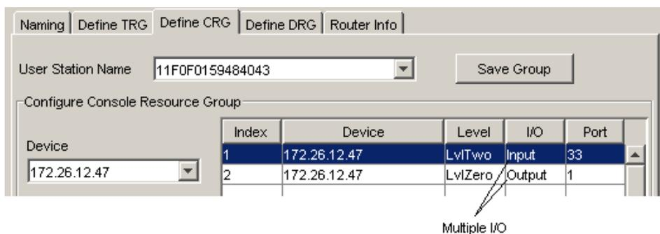
Figure 4.7: Defining CRGs - Multiple I/O
