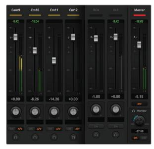
Try sliding the gain faders up and down on your hardware control surface and verify that the audio mixer faders show a corresponding movement in the software on your computer screen
