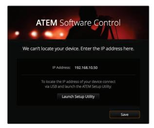
The setup dialog box will help you if you need to manually add your switcher's IP address when launching ATEM Software Control.
