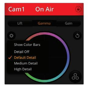
The camera settings button lets you turn color bars on or off and adjust the in-camera sharpening of connected Blackmagic Studio cameras. Step 4. On the Blackmagic Studio Camera, press 'menu'. Navigate to studio settings>camera number and set it to match your switcher input. For example, if studio camera 1 is connected to 'cam 1' on your ATEM switcher, your camera number must also be set to 1. This ensures tally is sent to the correct camera.
