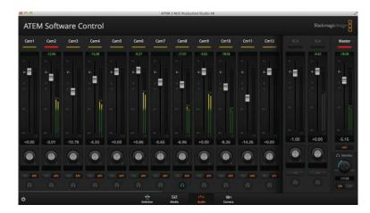
ATEM switchers include a built-in audio mixer that lets you use the embedded HDMI and SDI audio from your cameras, media servers and other inputs without the need for an external audio mixer. This is perfect when using an ATEM switcher on location or in small spaces within modern OB vehicles as you don't have to find room for an external audio mixer. The audio is mixed in the Audio tab of ATEM Software Control and output via the SDI and HDMI program outputs.
