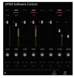
The audio mixer displays tally lights for any audio sources that are currently on air or when AFV is selected, as well as audio level, audio balance and buttons for selecting which audio should be used.
