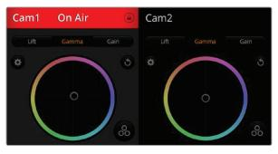
Each camera controller displays the channel status so you know which camera is on air. Use the color wheels to adjust each YRGB channel's lift, gamma and gain settings.
