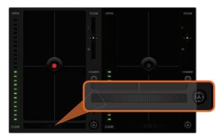
Click on the auto focus button or drag the manual focus adjustment left or right to focus a compatible lens.
