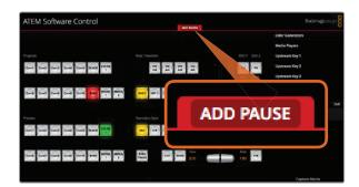
ATEM Software Control displays a red border to indicate when you are recording a macro. The 'add pause' button located at the top of the red border lets you enter durations for pauses between switcher actions.
