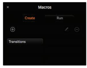
The image above shows how a macro button appears in the macros window after it has been recorded. To run a macro, click on the 'run' button to enter the run page. Now you can load and/or run the macro by clicking on the macro button.
