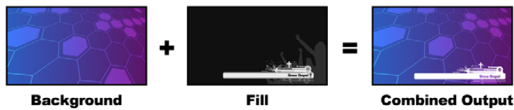
Combining a background and fill/key in a luma key
