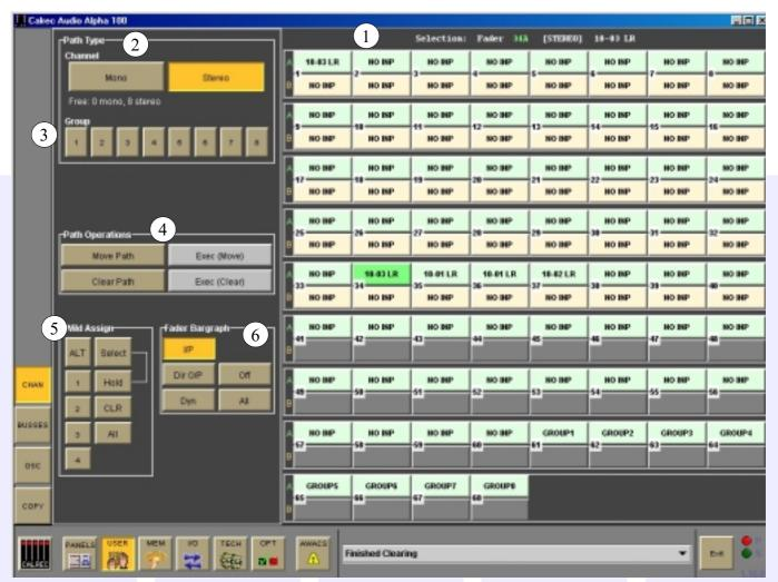
This screen provides alternative controls for channel functions already available on the control surface. It provides a back-up set of controls, which can be used should the control surface develop a fault.
