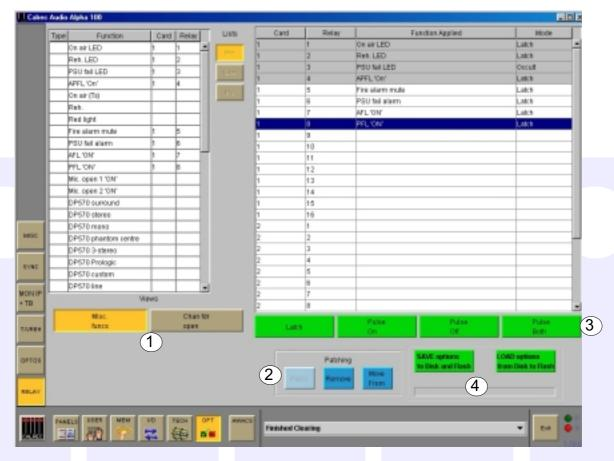
The Relay-isolated Output connections for various Console Functions can be assigned here in the same way that Opto-isolated Inputs are assigned.
