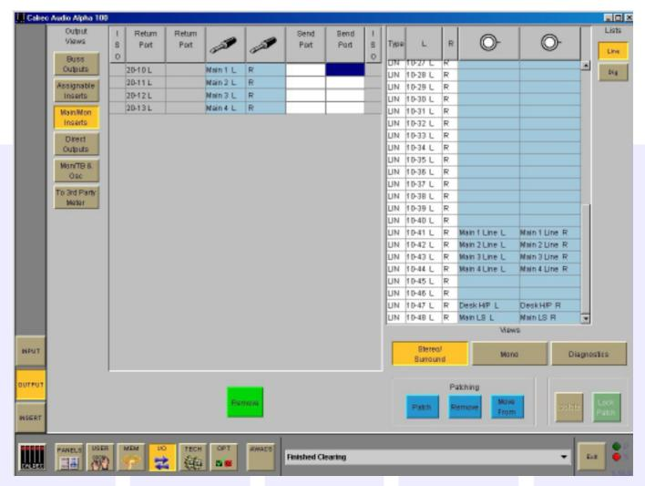
The Main and Monitor Insert Sends are set up on the Output Ports screen, by selecting "Main/Mon Inserts" from the list of Output Views. The Output Ports for Main and Monitor Insert Sends can be patched, moved and removed here in the same way as buss outputs are patched.
