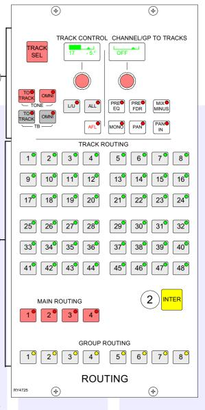
The Mix Minus, Pre-EQ and Pre-Fader buttons act as a cancelling set. When none are selected the signal is sent to the track routing selector Post-Fader. Mix Minus feeds the Mix Minus signal of the channel or group, as set up on the Direct Output section of the Input/Output panel, to the Track Routing selector.
