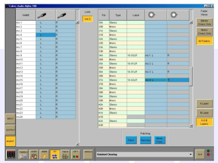
Once the Assignable Insert Sends and Returns have been set up on the Input and Output screens, they can be patched here to channels and groups, in the same way that channel inputs are patched. The Fader View buttons select which paths are on display. The Assignable Inserts can also be patched to channels and groups by using the I/O Matrix panel on the console. Once connected, the Insert is switched into the channel path using the buttons on the Input/Output module (shown).
