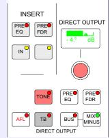
halves of the pair can be used for separate mono signals. The inserts can be viewed as pairs (best for patching to stereo paths) or individual (best for patching to mono paths).
