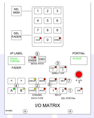
It is possible to determine which lists of input ports appear for selection on the I/O Matrix Panel using the Options-Miscellaneous screen. By only making the relevant lists available for selection reduces the number of times the pot needs to be pushed, to go through all the available lists.
