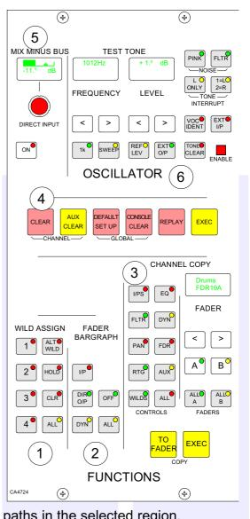
It is possible to assign the same control to Wilds 1, 2, 3 or 4 for all fader paths by selecting ALL before pushing the required Assign Panel rotary control.
