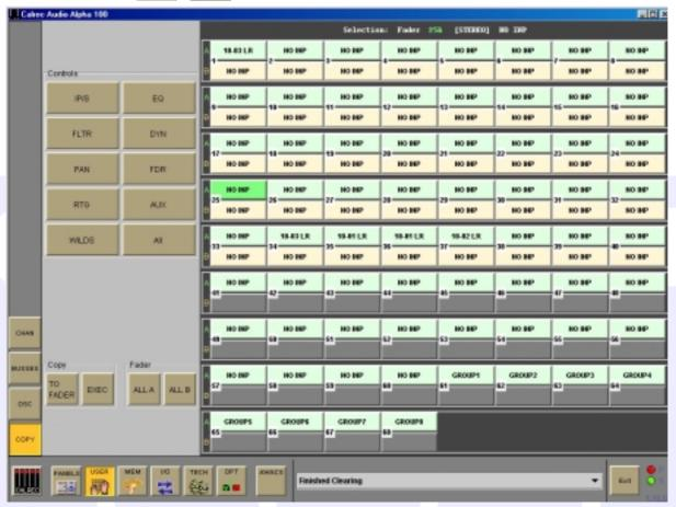
In addition to the controls on the Functions panel, nine sections of a channel or ALL together can be copied to another channel or channels using this screen. If a stereo channel's settings are copied to mono channels, only the relevant settings will be copied. If groups or mains are included in the selected destinations, they will simply be ignored.
