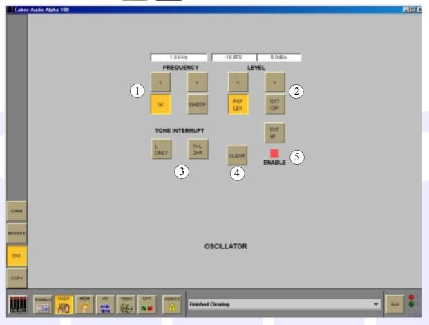
This screen provides alternative controls for the oscillator controls already available on the control surface. It provides a back-up set of controls, which can be used when using the panel is not convenient, or should the control surface develop a fault.
