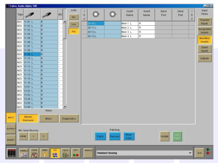
The Main and Monitor Insert Returns are set up on the Input Ports screen, by selecting "Main/Mon Inserts" from the list of Input Views. The Input Sources for Main Insert Returns can be patched here in the same way that channel inputs are patched.
