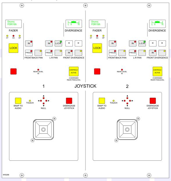
The joystick panel is available as an option, and can be either a single joystick, or twin joysticks as shown above. The joysticks allow accurate stereo and surround panning of the channel, group or main path.
