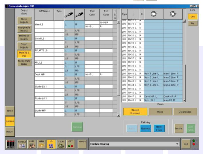
The output ports for the Monitoring, Talkback and Oscillator Outputs can be patched on the Output Ports screen, by selecting "Mon/TB & Osc" from the list of Output Views.
