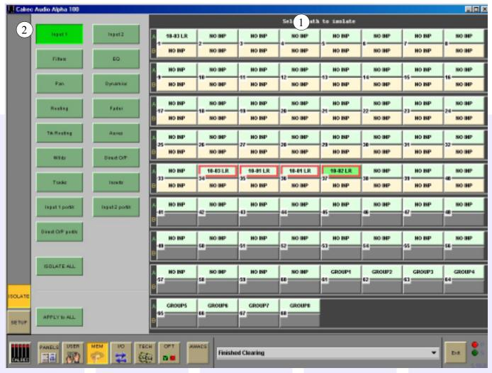
The Isolate screen allows some console settings to be isolated from memory recall. This means their current settings will not be over-written by what is in the memory when it is loaded.
