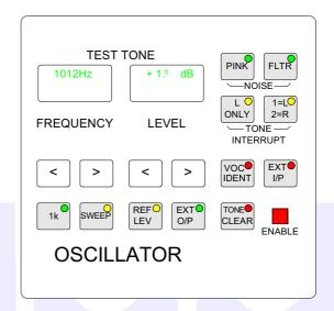
The oscillator can be set to generate pink noise instead of a tone, by selecting the PINK noise button. The FLTR button filters out frequencies below 400Hz and above 1500Hz from the pink noise generated.
