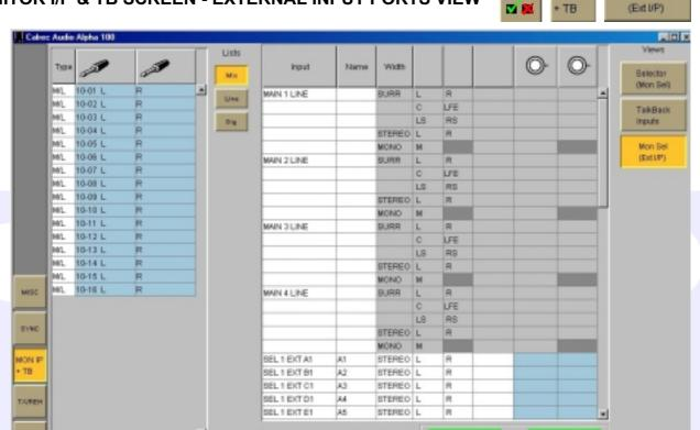
The Input Sources for External Monitor Inputs can be patched here in the same way that channel inputs are patched. The NAME of the external input will correspond to the text on the button as shown on the Monitor Selector View.
