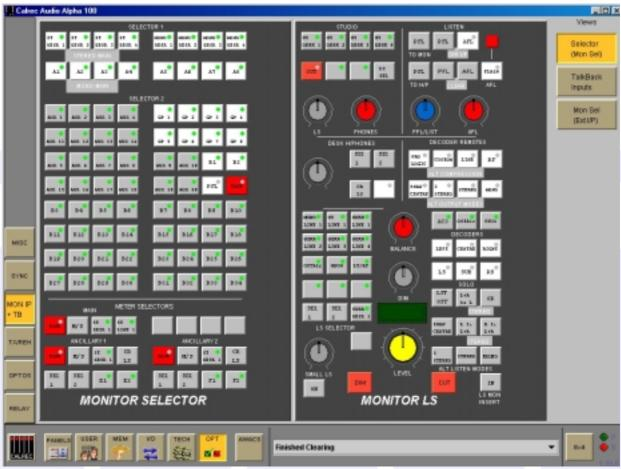
This screen gives a confirmation of how the Monitor Selector panel buttons have been set up.
