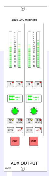
These modules control the Auxiliary outputs.
