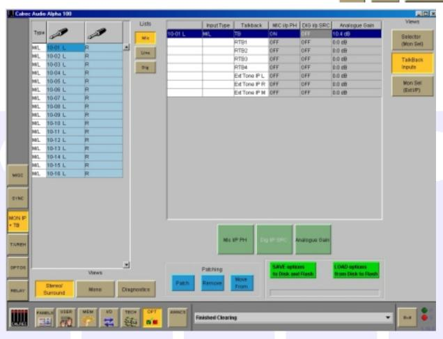
The Input Sources for Talkback and Reverse Talkback can be patched here in the same way that channel inputs are patched. Talkback input ports can be any kind of port.
