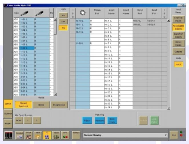
The Assignable Insert Returns are set up on the Input Ports screen, by selecting "Assignable Inserts" from the list of Input Views. The Input Sources for Assignable Insert Returns can be patched, moved and removed here in the same way that buss outputs are patched.
