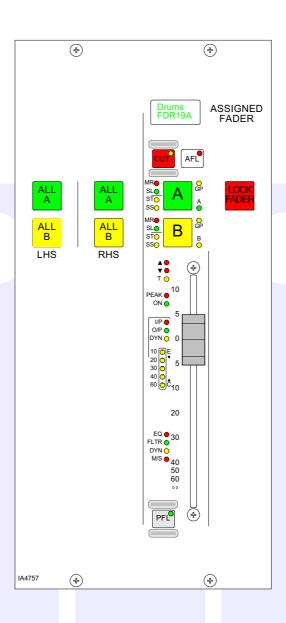
The Assignable Fader is positioned towards the centre of the console, in the optimum listening position, and works in parallel with the last "Channel" Fader selected. Alternatively, the LOCK FADER button allows it to be fixed to a specific path.
