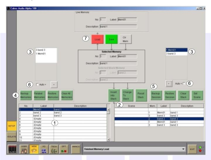
99 memories can be held in the Flash ROM for different console arrangements. In addition to this, the PC back-up can allow an unlimited number of memories, which can be called into the Flash ROM quickly and easily. Memories can be stored to removable media such as floppy disk. This can be useful for when many different operators use the same console (for example an Outside Broadcast vehicle), or when the console is required to broadcast many different weekly productions.
