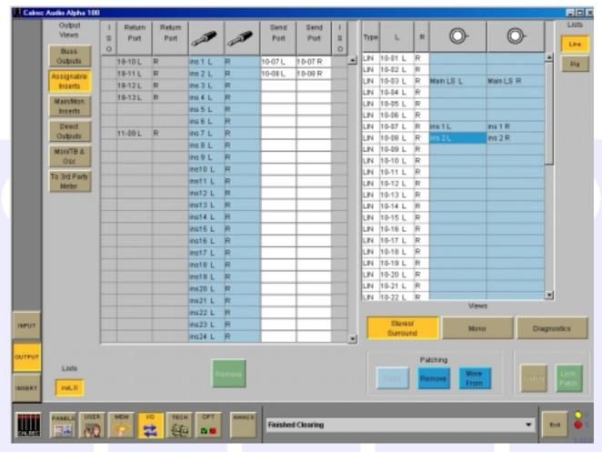
The Assignable Insert Sends are set up on the Output Ports screen, by selecting "Assignable Inserts" from the list of Output Views. The Output Ports for Assignable Insert Sends can be patched, moved and removed here in the same way that buss outputs are patched.
