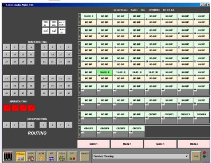
This screen works in parallel with the console Assign Buttons and the Routing panel. It provides alternative controls for the routing, which can be useful should the Routing Panel develop a fault.
