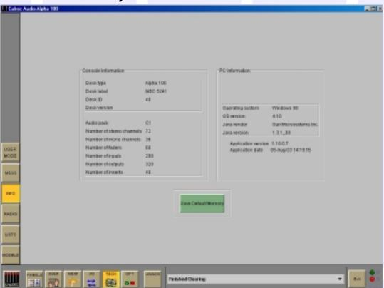
The Default Memory will usually be created upon installation of the Alpha 100 using the Save button on this screen. This default memory could contain the input port set-ups which match the studio wiring, and settings for relays, optos, and running levels. It could have all channel settings OFF or flat, with no routes made, and would be available as a start up memory, from which more specific memories could be created. It is recalled using the Default Set Up button on the Functions panel.
