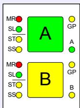
Each fader has an “Assign” button (sometimes called the “Show Me” button) for each audio path. The Assign buttons are labelled A and B for channel or group paths, and M1, M2, M3 or M4 for the main output paths on the main faders. Pressing the Assign button causes the central control panels (the “Assign panels”) to display and control the settings for that fader’s channel, group or main path.
