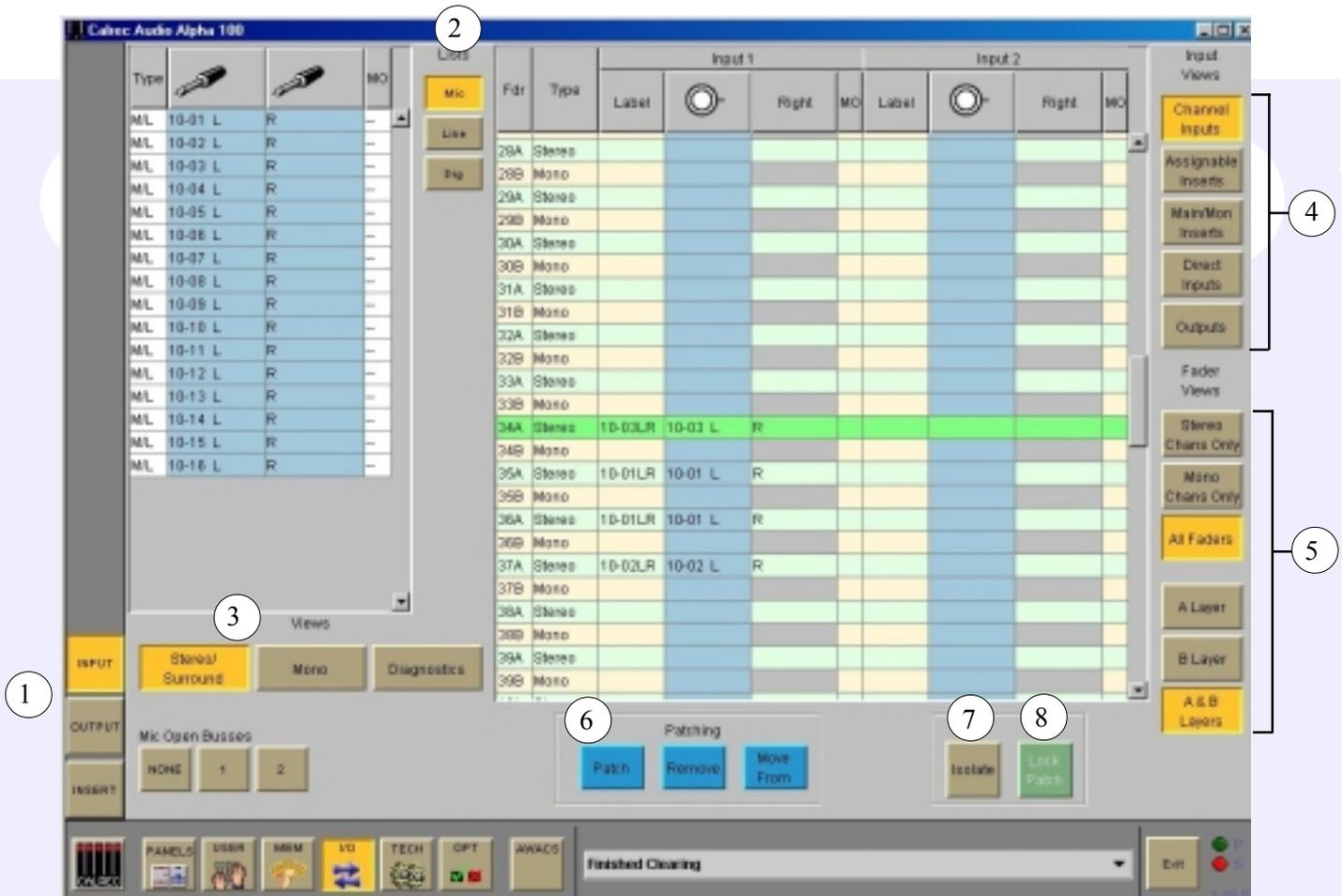
On the control surface, ports are assigned using the I/O Matrix panel, but these screens provide an alternative set of controls. The screens automatically scroll to follow the Assign button (A and B) presses on the faders.
