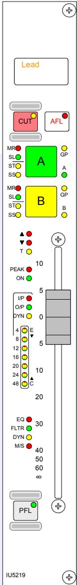
Channel and group paths are controlled by the console’s “Channel” faders. Each fader can control two independent audio signal paths, named A and B. Any fader can control any channel or group path. Main output paths are controlled by their dedicated faders on the Main outputs panel.
