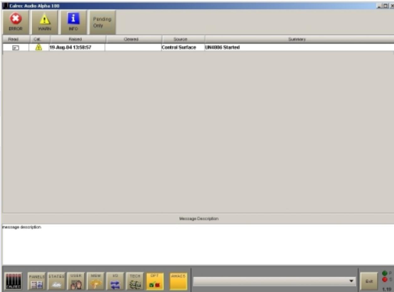
If a problem does develop, messages will be delivered on the Automatic Warning and Correction System (AWACS) screen. The AWACS button at the bottom of the screen will flash to alert the user that a message has been reported. Selection of this button will open the AWACS page, where messages can be viewed. Selecting a message will reveal a more detailed description. Message history is saved to the PC’s hard disk for future analysis.
