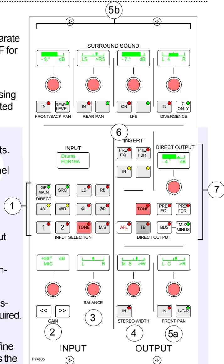
The Front Pan allows the front signal to be panned from left, through centre, to right. On stereo channels and groups, the L-R PAN acts as a balance control.
