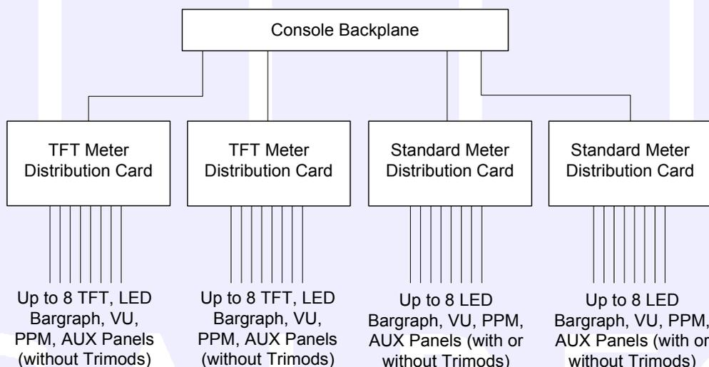
In addition to the TFT meter distribution cards, it is also possible to fit up to 2 standard meter distribution cards for connecting to current meter panels with trimod LCD displays. So, for example, in a system which had 2 TFT meter distribution cards and 2 standard meter distribution cards fitted, it would be possible to incorporate 16 TFT metering panels, and 16 standard meter panels into the system -although it is not likely that this number of standard meters would be required.
