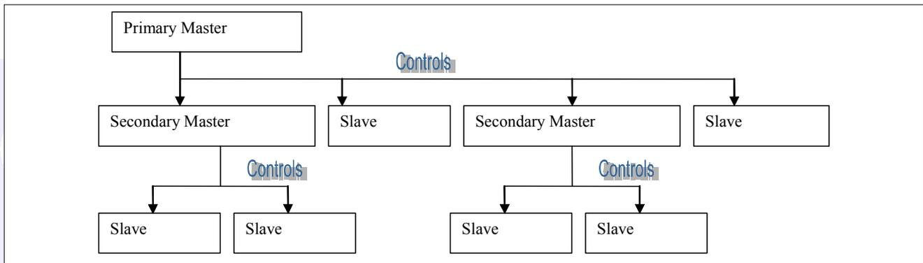
When the level of a primary master is adjusted it will change the audio level of its slaves and the levels of its secondary master's slaves by the same amount. The slave faders will not move, the Null LEDs will illuminate to indicate whether the audio is above or below the position of the fader. The CUT, AFL and PFL settings will also be applied to all the slaves, secondary masters and their slaves.
