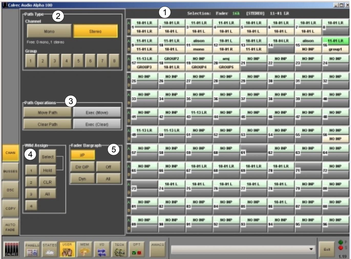
This screen provides alternative controls for channel functions already available on the control surface.
