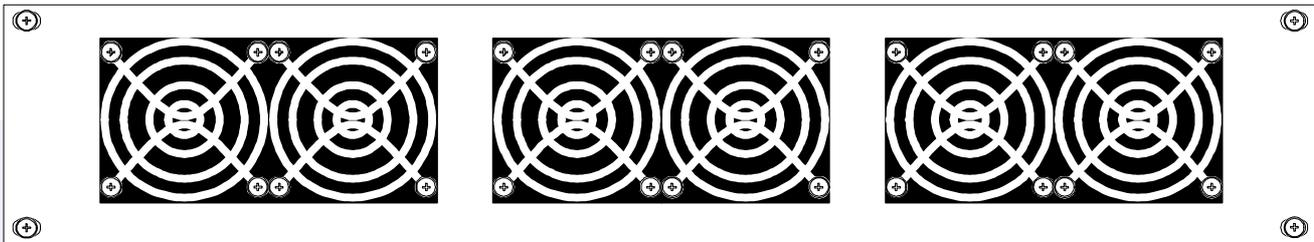
The Bulk PSU Rack is a 2U rack which can hold up to three identical 24V 1kW plug-in PSU's. The rack has separate AC power inputs and DC outputs for each of the three PSU's. Any one PSU can be removed from the rack without disturbing the operation of the others in the rack. The number of PSU's required in the rack is dependant upon the size of the system, the distance between console and rack, and the "hot spare" require-
