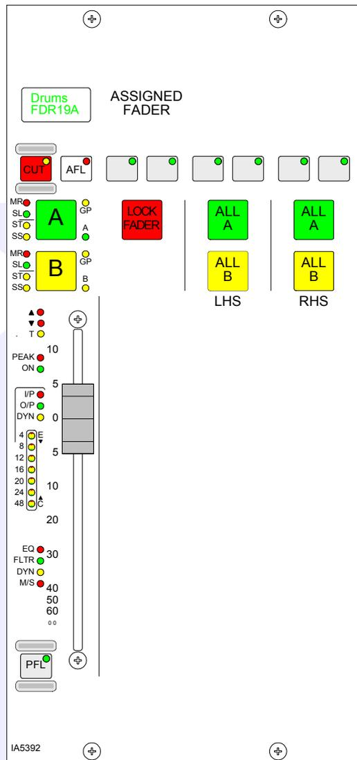
The Assignable Fader is positioned towards the centre of the console, in the optimum listening position, and works in parallel with the currently assigned channel or group fader. Alternatively, LOCK FADER allows it to be fixed to a specific path.
