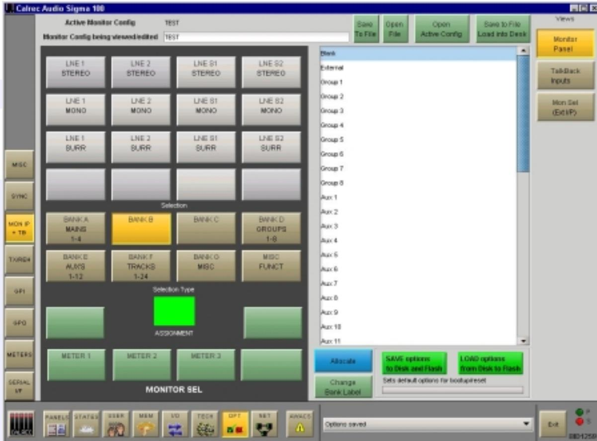
The left side of the screen shows a representation of the monitor selection panel. The right side of the screen lists all the available monitor sources. Monitor sources are allocated to the 16 selection buttons on each bank as follows:
