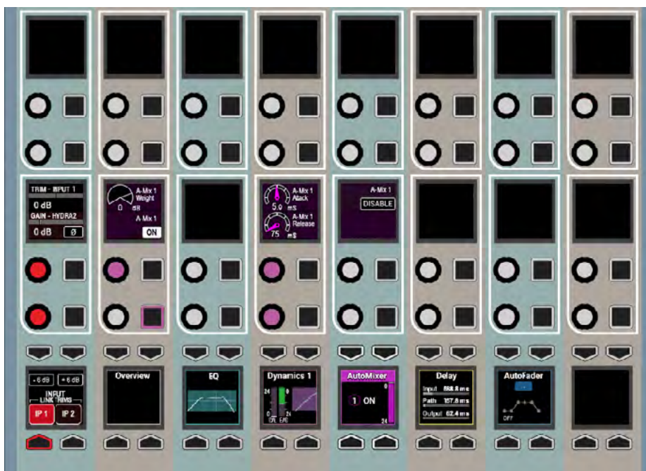
FIG 2 - AUTOMIXER CONTROLS ON THE PROCESSING-DYN2 PANEL LAYOUT
