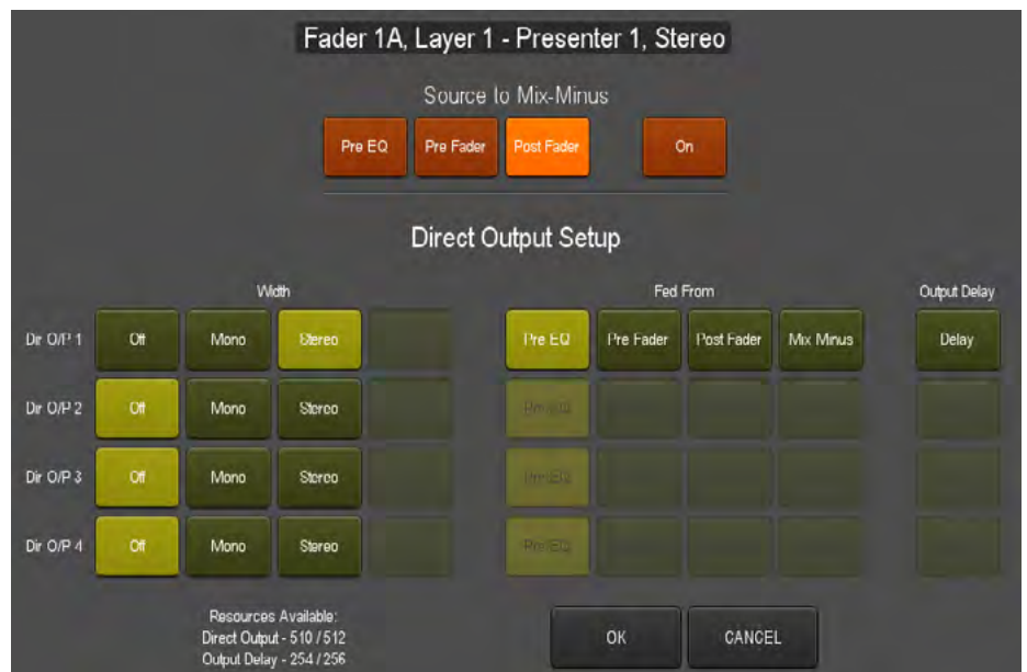
FIG 2 - DIRECT OUTPUT SETUP POP-UP
