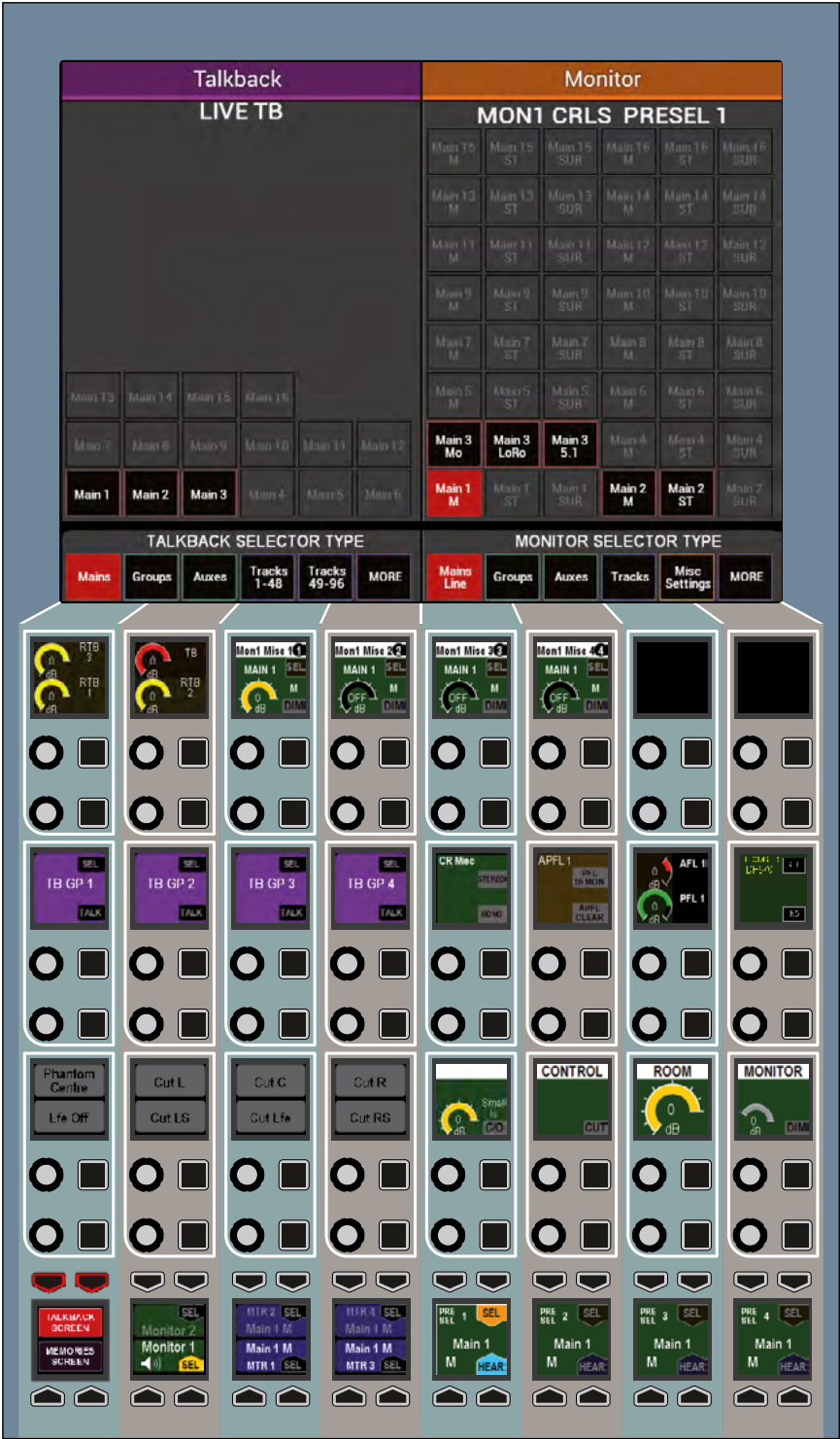
FIG 1 - CONTROL LAYOUT IN MONITOR MODE
