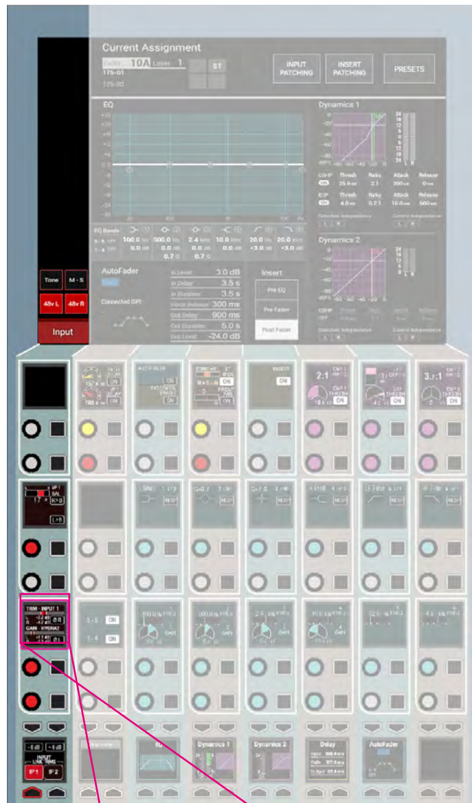
FIG 1 - INPUT CONTROLS COLUMN ON PROCESSING OVERVIEW
