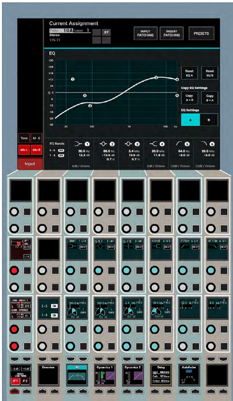
FIG 1 - EQ CONTROLS ON THE PROCESSING-EQUALISER ASSIGN MODE LAYOUT
