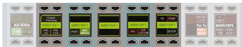
FIG 3 - MONITORING A MIX MINUS SIGNAL
