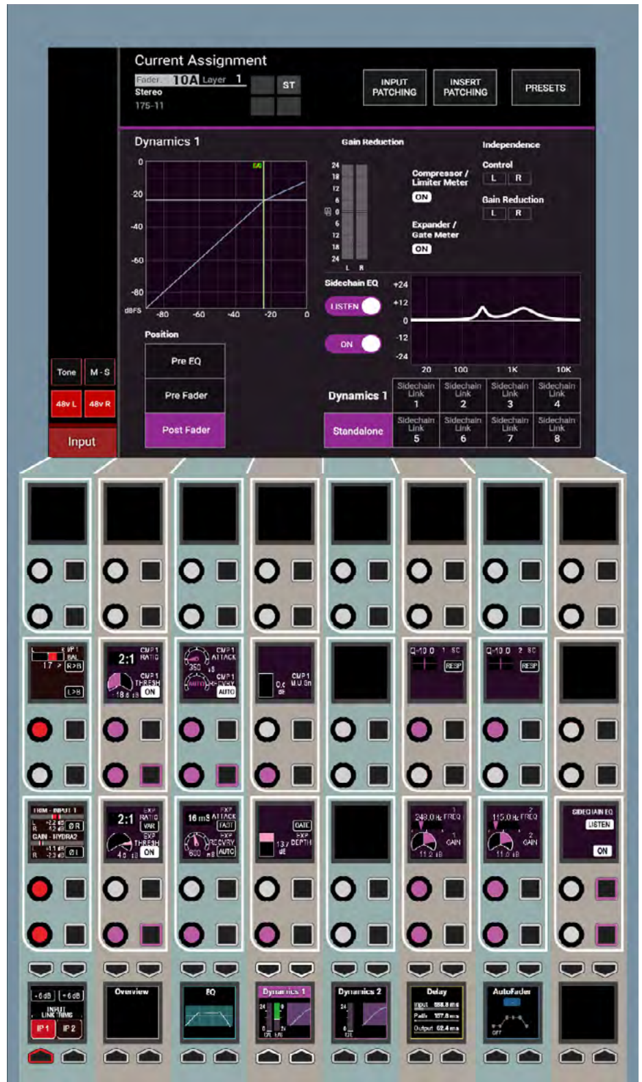
FIG 1 - DYN CONTROLS ON THE PROCESSING-DYN 1 ASSIGN MODE LAYOUT
