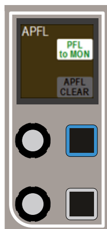
FIG 6 - MONITOR PANEL MODE PFL TO MON
