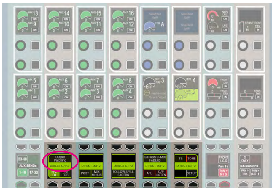
FIG 3 - ADDITIONAL CONTROLS FOR EACH DIRECT OUTPUT
