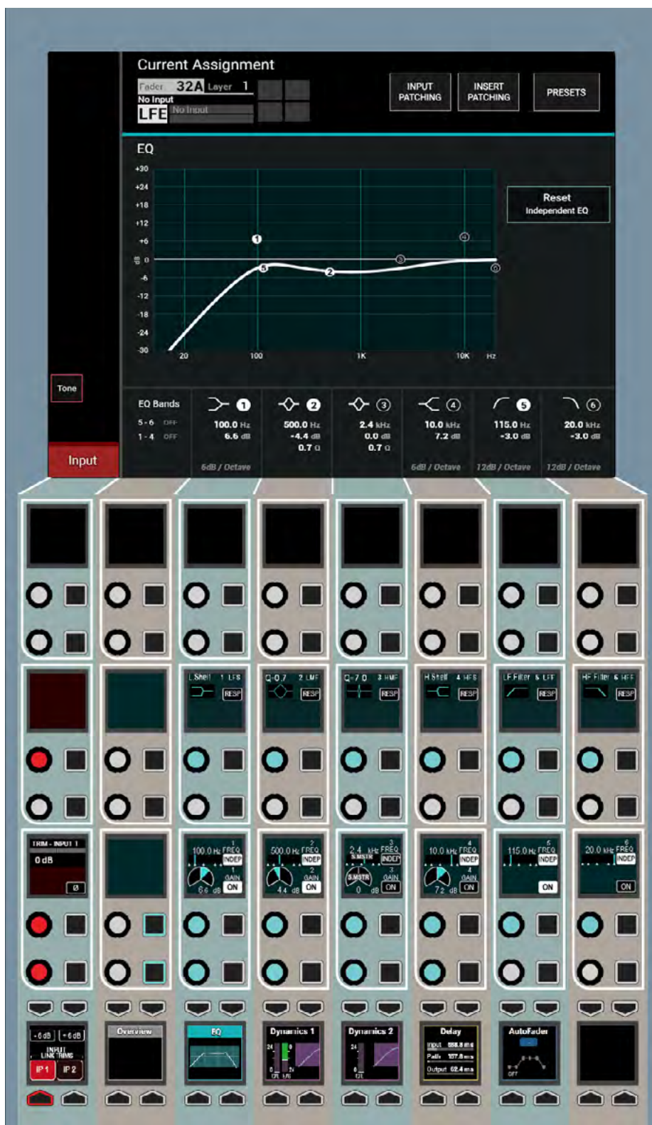
FIG 1 - EQ INDEPENDENCE CONTROLS
