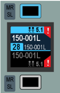
FIG 3. - SOURCE OFFLINE INDICATION
