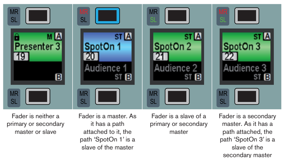
FIGURE 2 - FADER STATUS
