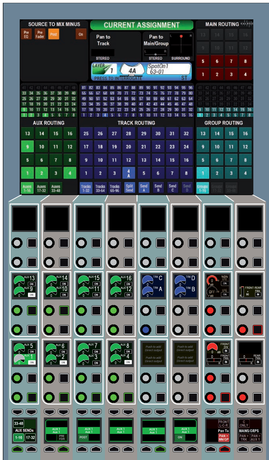
FIGURE 2 - THE SENDS-ROUTES ASSIGN LAYOUT
