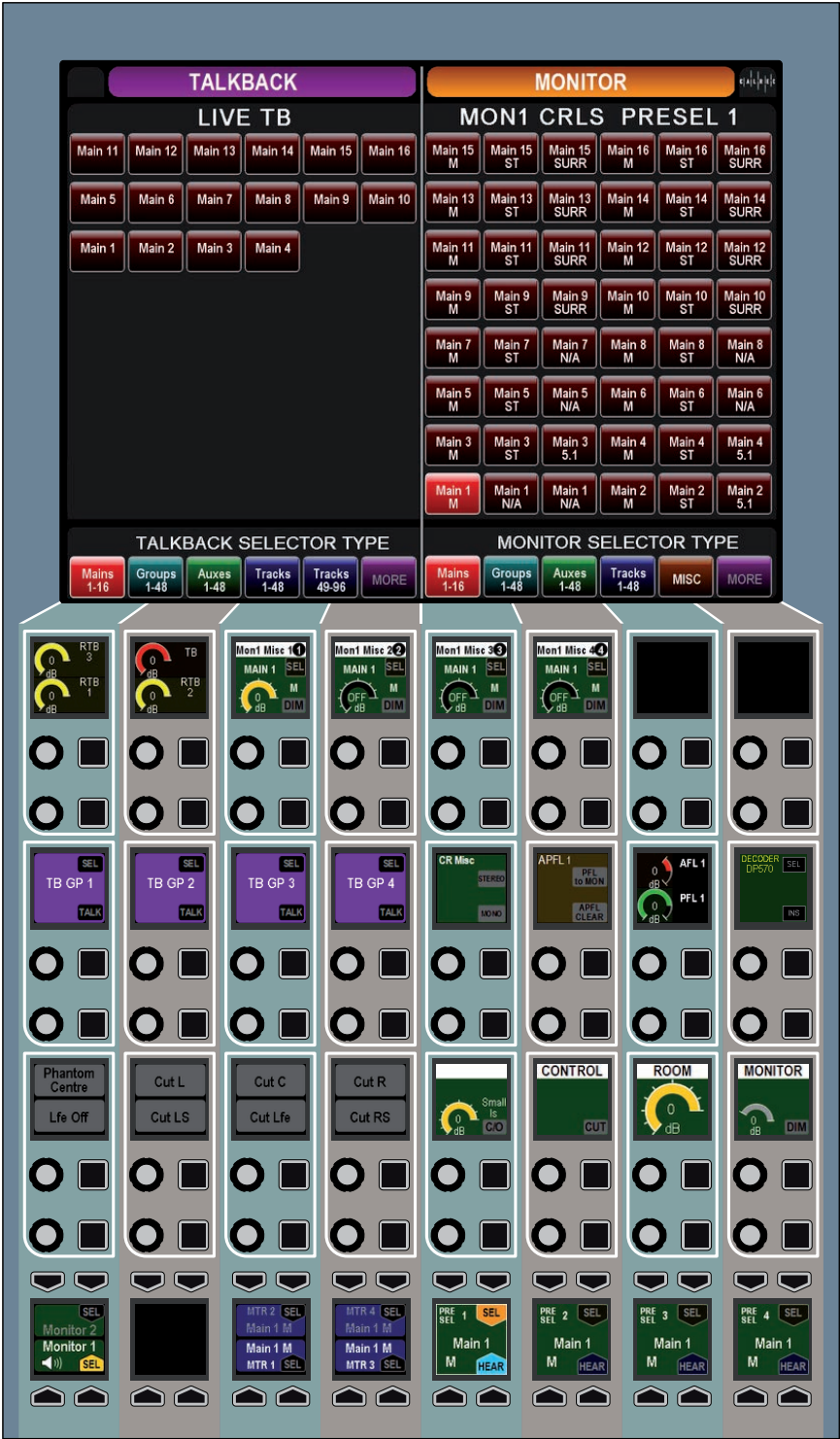
FIGURE 1 - CONTROL LAYOUT IN MONITOR MODE
