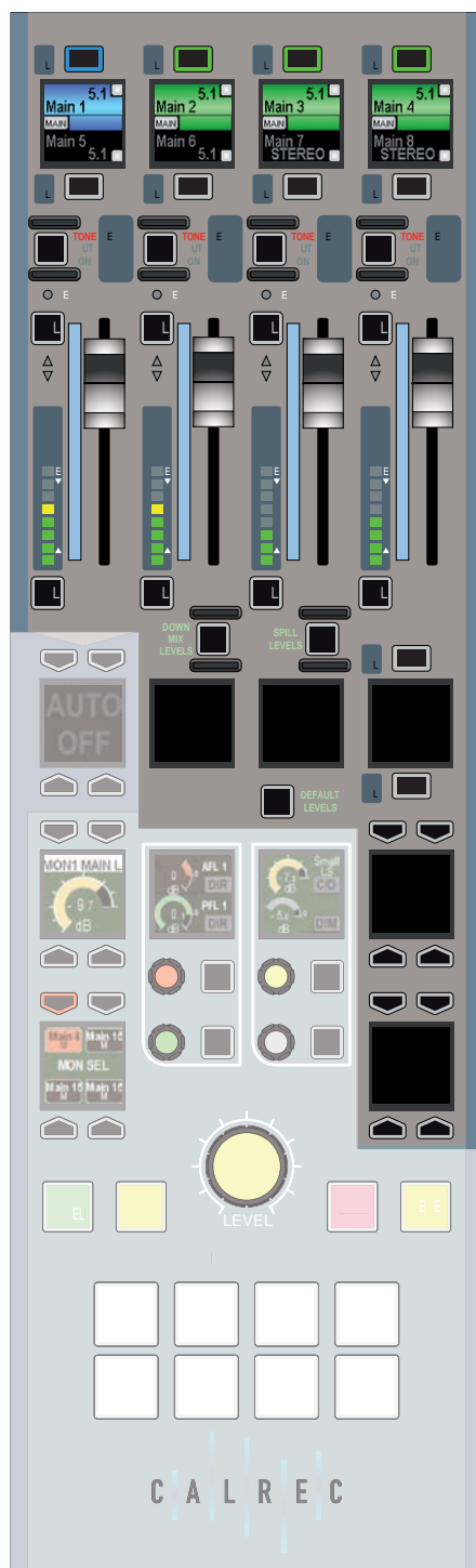
FIGURE 1 - MAIN PATHS ON MONITOR PANEL
