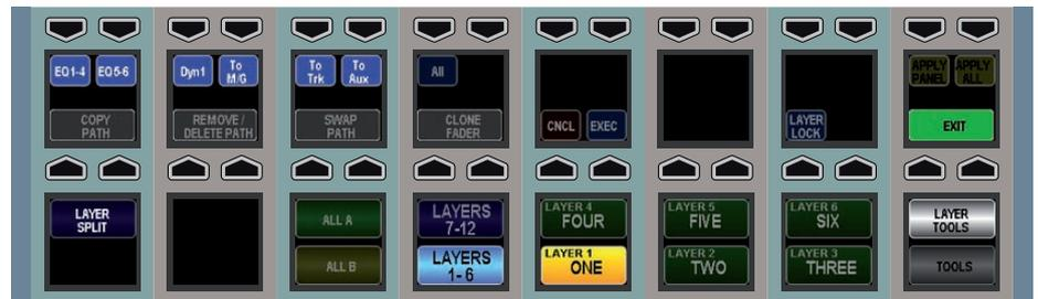
of the selected layer. To lock a path touch the LAYER TOOLS button on the Layers Row. On the updated Functions row above, touch and hold the LAYER LOCK button and then tap the assign buttons of any faders which contain paths that are to be locked to the surface. Holding LAYER LOCK and tapping an assign button toggles the lock on and off.
