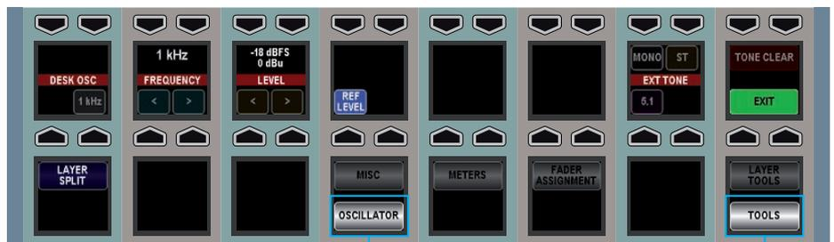
Press the TOOLS button, then the OSCILLATOR button to bring up the oscillator controls
