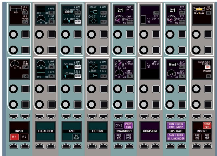
of gain reduction applied to it. This same amount of gain reduction is also applied to all other legs even if they didn't cross the threshold. This keeps the relative balance of the sound field intact.
