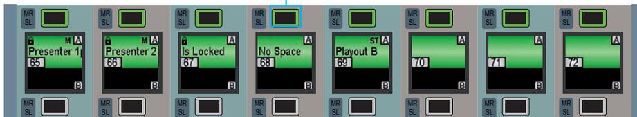
Paths may only be inserted if there are enough empty faders to the left or right of where the path is inserted. If there are locked paths between the empty faders and the path to be inserted they will not allow the insertion to continue. Similarly, paths cannot be moved past the faders at the left and right edges of the surface.
