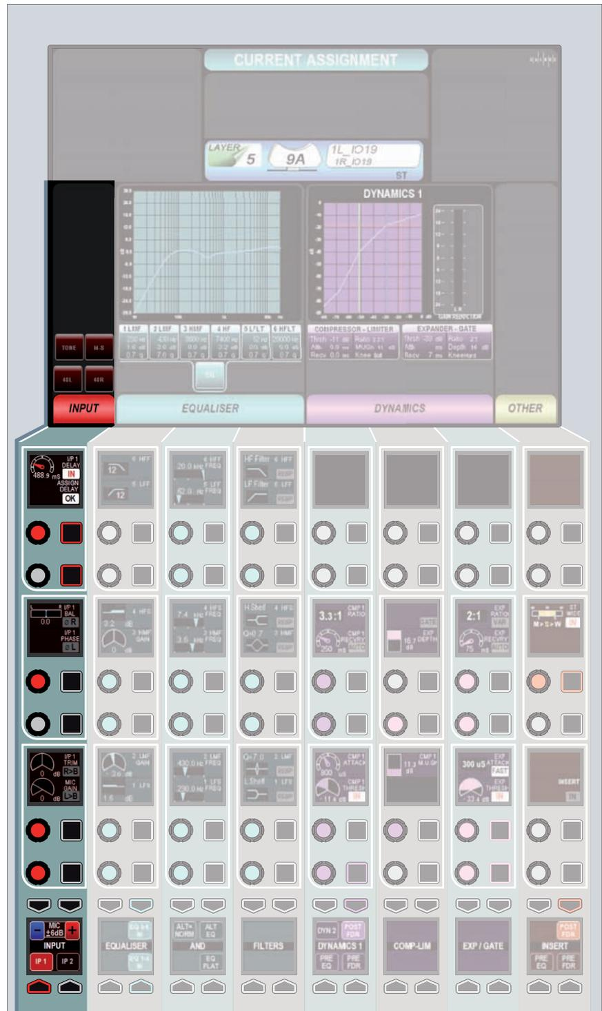
This is the only input gain control available for digital input signals and the only input gain control available for a port owned by another user. As the gain is applied inside the channel path it has no effect on any other operators using the same port.
