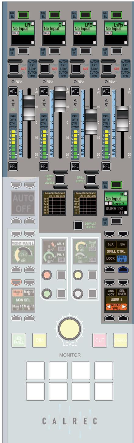
the surface. They have the same assign buttons above and below the fader label OLED, the same AFL, PFL and cut buttons and the same bargraph meters. They can be assigned in the same way as any other fader and by doing so, individual control of the processing of a specific component path is possible.
