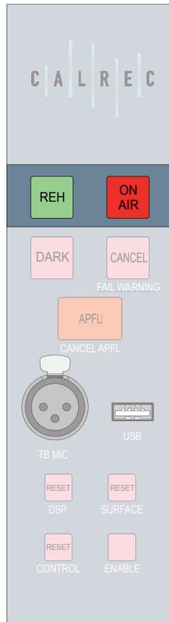
It also allows control over a separate external interface via GPOs than the On Air mode, such as a Rehearse light.
