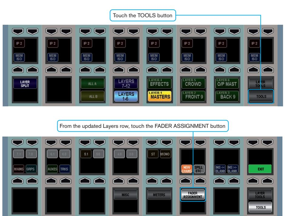
**FIGURE 3 - INSERTING BLANKS**
