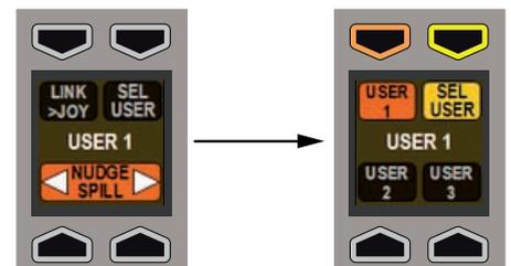
If the path controlled by the spill faders is locked, the path selection OLED on the spill panel will not follow the path assignment on the surface. It will display the locked path as an indicator of which path is being controlled by the spill panel.
