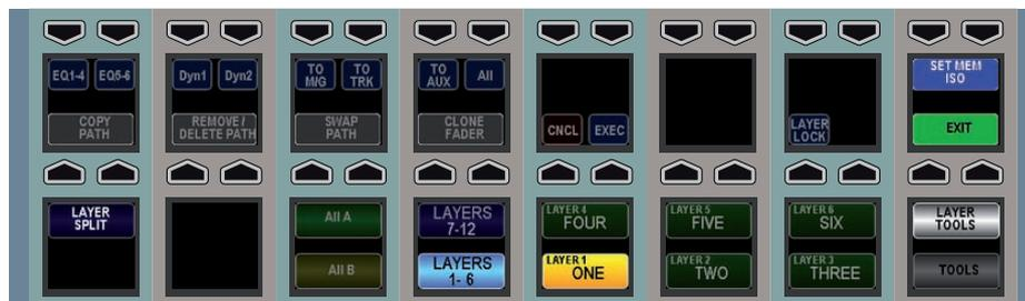
The lower two rows of control cells on the wild assign panel will now display the elements of the path which can be isolated. They relate to the currently assigned path. These elements may vary depending on the type of path assigned, for example input and input port settings are not applicable to groups.
