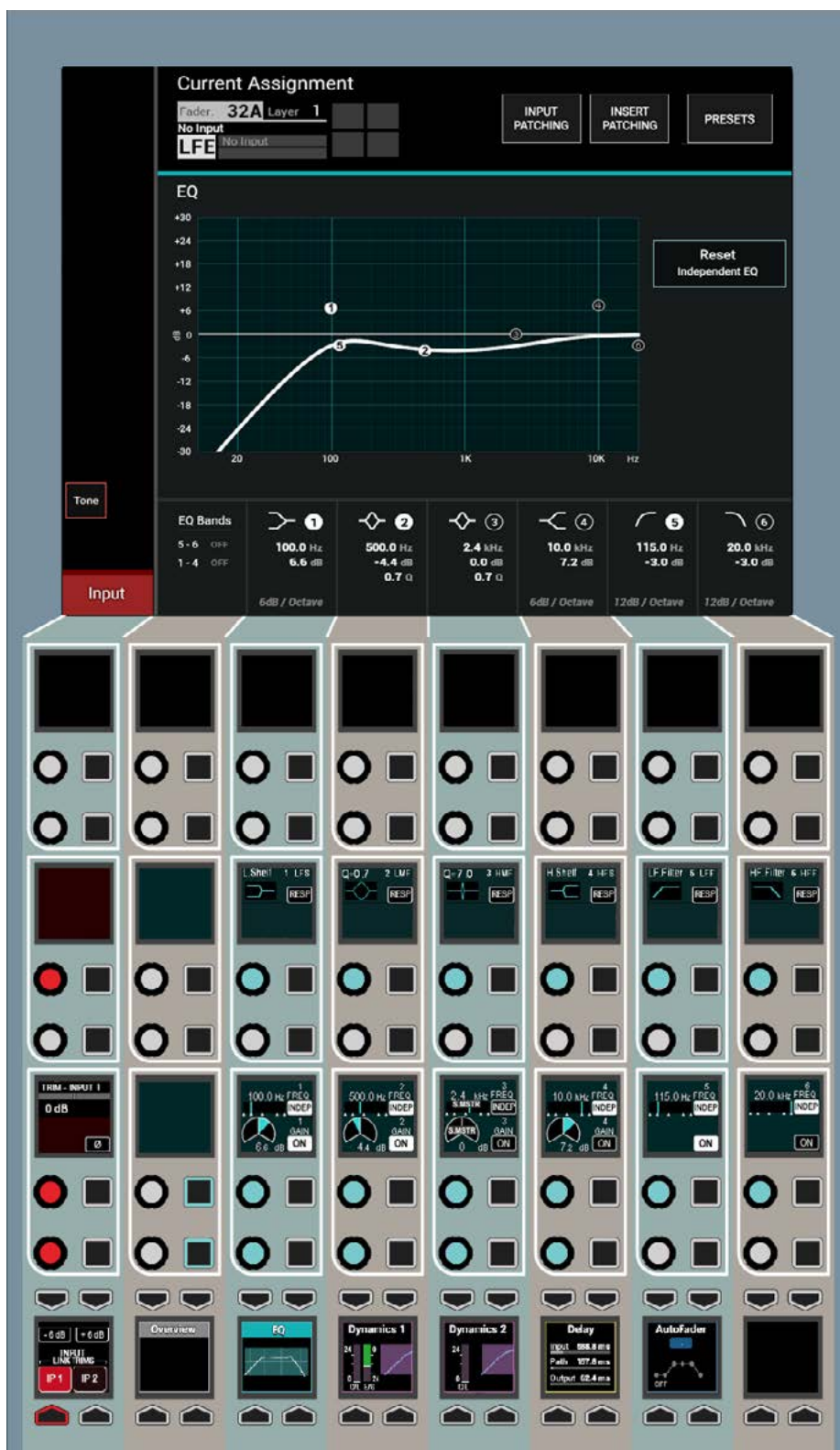
FIG 1 - EQ INDEPENDENCE CONTROLS
