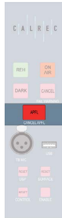
FIG 2 - ACCESS AFL AND OUTPUT LISTEN FOR OUTPUT BUSES
