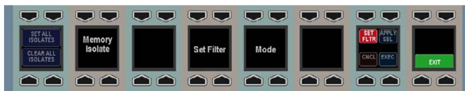
FIG 5 - WILD ASSIGN ROW IN SET FILTER MODE
