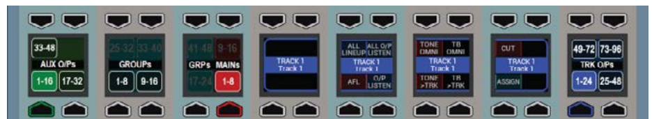
FIG 2 - ACCESS AFL AND OUTPUT LISTEN FOR OUTPUT BUSES
