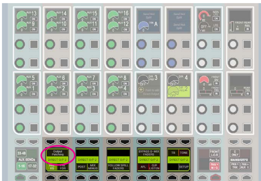
FIG 3 - ADDITIONAL CONTROLS FOR EACH DIRECT OUTPUT
