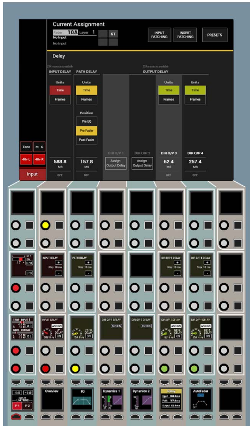
FIG 1 - DELAY CONTROLS ON THE PROCESSING-DELAY ASSIGN MODE LAYOUT
