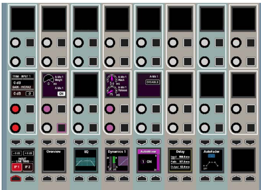
FIG 2 - AUTOMIXER CONTROLS ON THE PROCESSING-DYN2 PANEL LAYOUT
