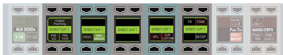
FIG 3 - MONITORING A MIX MINUS SIGNAL
