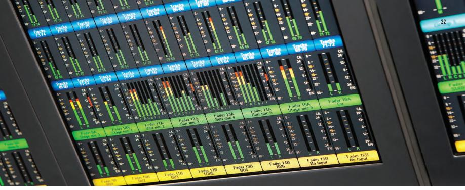
With per-channel bargraph meters next to each fader and multi-channel metering via an array of TFTs, Apollo offers no shortage of ways to monitor signal levels.
