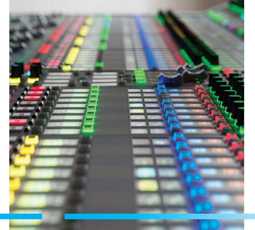
as an eight or 16 fader sub mixer using the same processing hardware and linking to the main console with a simple Cat5e or fiber cable. Layers give an operator the ability to access many more channels on this compact frame.
