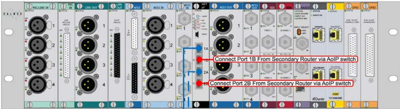
Modular I/O Box with AoIP interface Module
