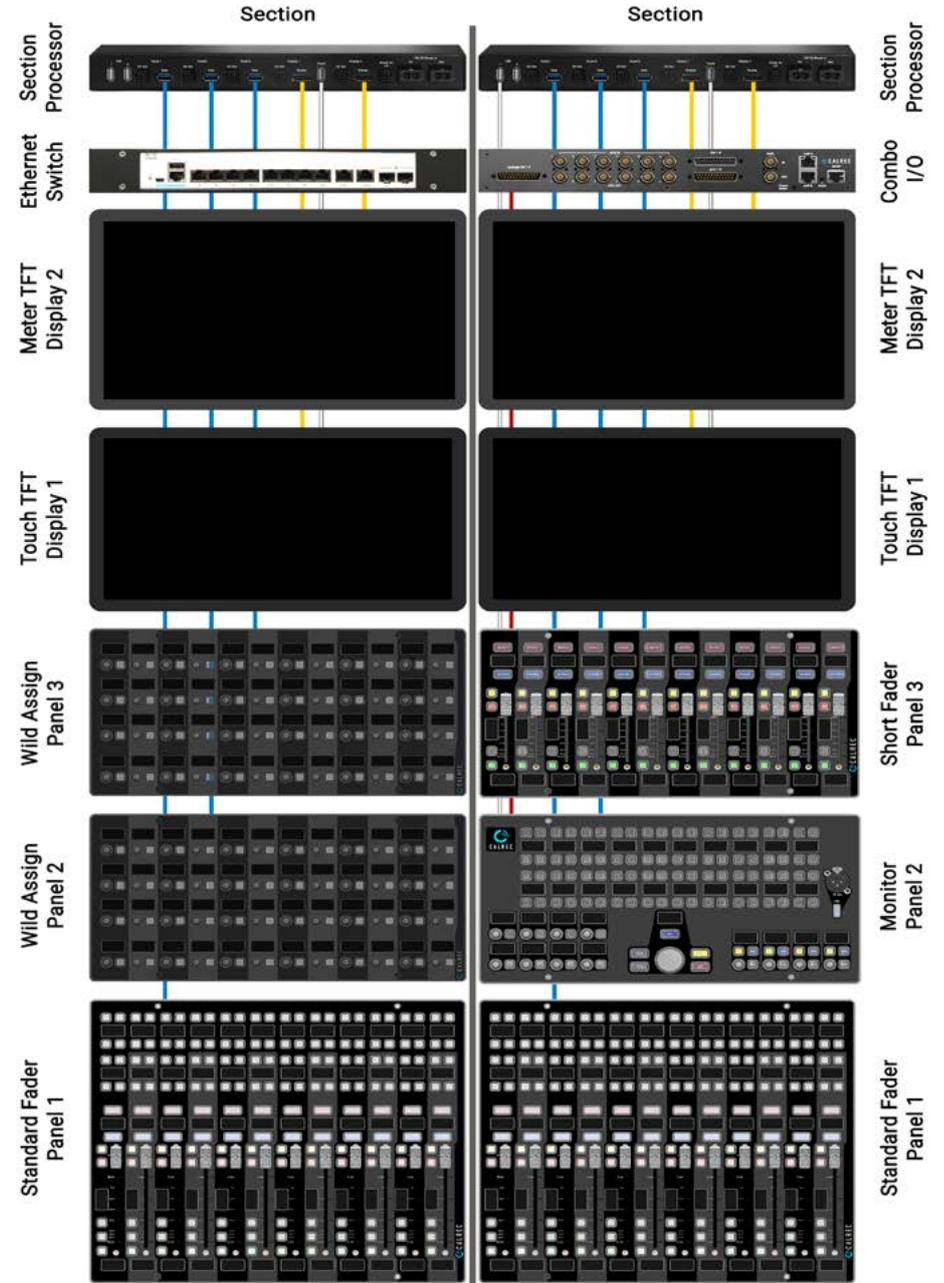
Display 1's DP connector is used for the MU6572 Touch display TFT panel, together with its USB 2.0 touch port
