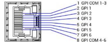
8-pin RJ45 GP input pin-out for GPI 1-6 or 7-12
