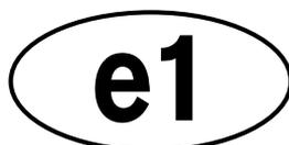
Circuit boards assembled with lead-free solder can be identified (in accordance with IPC/JEDEC standards) by a small oval logo (see Figure 2) on the top-side of the circuit board near the PCB reference number (8xx-xxx). The same logo is used on the connector hoods of soldered cable assemblies.
