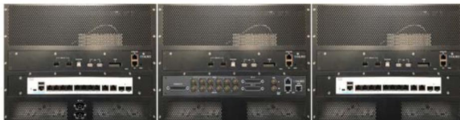
Argo Rear section 1 view showing Section Processor, 10 port Ethernet Switch and 2x IEC AC Mains inlets
