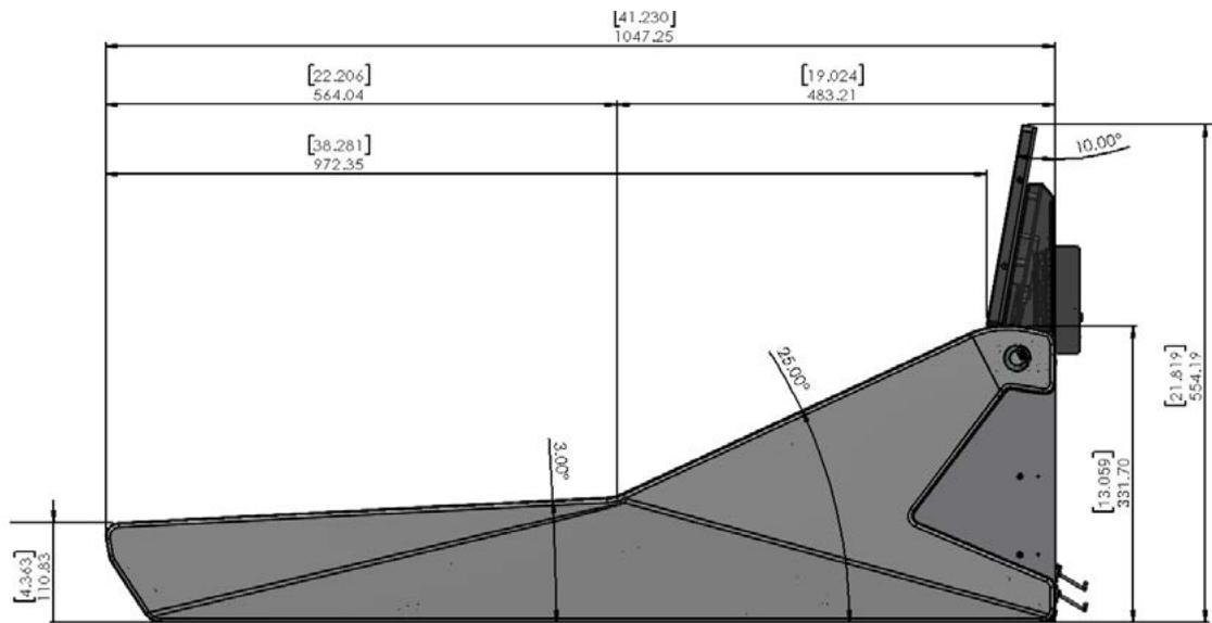
FIG 4 - FLOOR STAND FITTED ADJUSTABLE FEET, END ELEVATION ARGO Q
