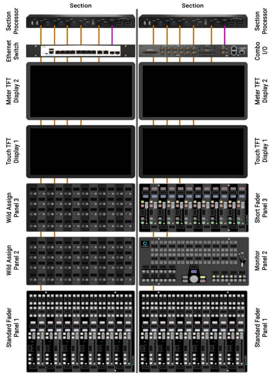
Power for I/O DC Out is used to power a 491-329 Cisco Ethernet switch, fitted into the back of a console section. Alternatively this can be used to power one of the AoIP interface modules also
