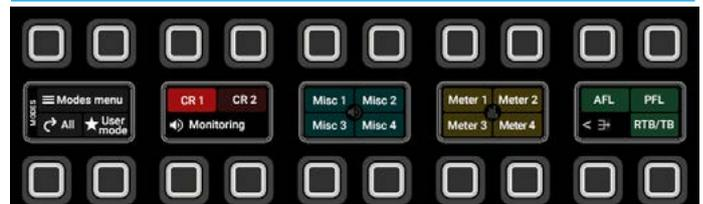
The image below shows the Wild Assign panel in [Processing>Input](#) mode. The layout of the controls approximately mimics the layout of the TFT touchscreen and changes according to the type of path and the mode that has been selected.
