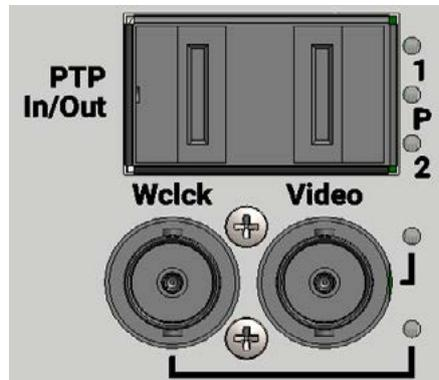
PTP specifies that the network has a Grand Master Clock source, which is generally synchronised to a high precision real-time clock source such as GPS.
