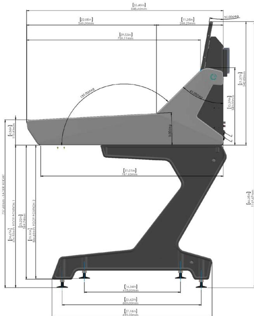
FIG 3 - NO FLOOR STAND FITTED, END ELEVATION ARGO Q
