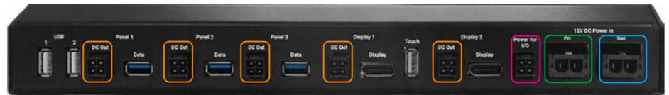
FIG 2 - DC OUT POWER DISTRIBUTION FOR TWO SECTIONS
