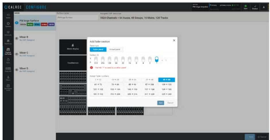
Fig 3 below right shows the console surface layout page in the Configuration Application which uses the Section Processor configuration switches to identify each section column and add the various Fader/Wild/Monitor/Short Fader/Touch TFT and Meter TFT panels associated with it.
