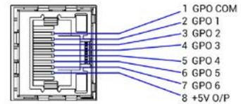
8-pin RJ45 GP output pin-out for GPO 1-6 or 7-12
