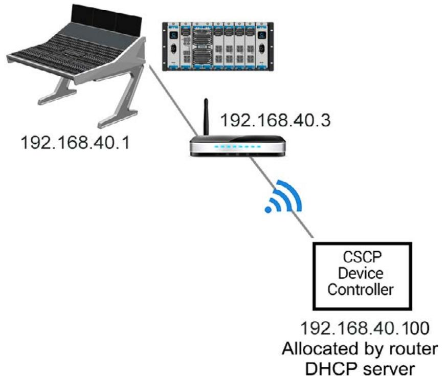
**FIG 4 - WIRELESS ROUTER TO CONTROL PROCESSOR CONNECTION**
