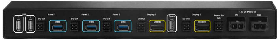
FIG 2 - USB3, DP & USB2 PANEL CONNECTIONS FOR TWO SECTIONS
