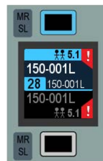
FIG 3. - SOURCE OFFLINE INDICATION
