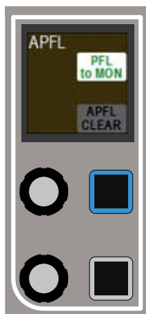
FIG 6 - MONITOR PANEL MODE PFL TO MON
