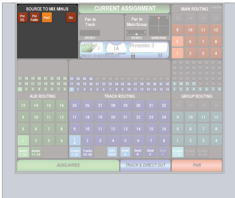
FIGURE 2 - SENDING SIGNALS TO THE MIX MINUS BUSS
