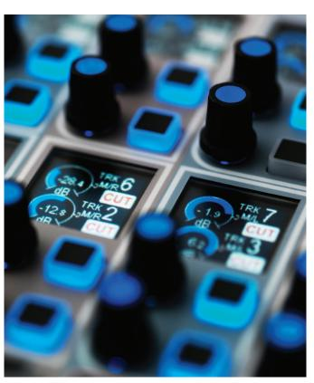
Monitor Mode provides additional functionality to the dedicated monitor panel. This could include talkback groups. It also allows multiple operators access to their own set of monitoring controls.
