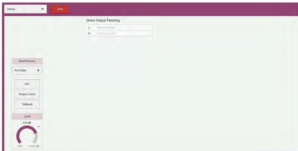
FIGURE 4 - ROUTING TONE TO A DIRECT OUTPUT
