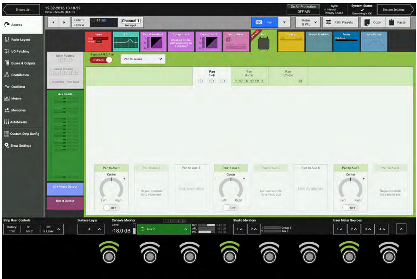
FIGURE 2 - PAN TO AUX CONTROLS
