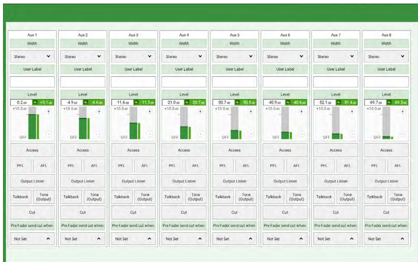
FIGURE 4 - AUX BUS OUTPUT FADERS—SLAVES IN VCA GROUP
