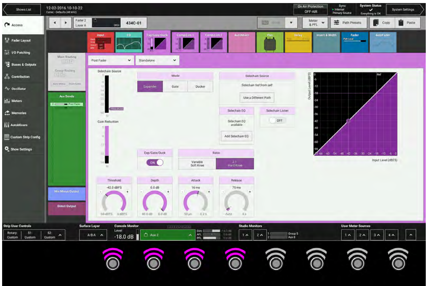
FIGURE 1 - CONTEXT CONTROLS—ACCESS MODE—EXPANDER/GATE/DUCKER*
