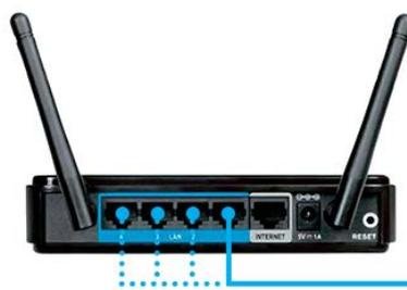
One connection from any LAN / ethernet port to the primary control processor - MAC 3, 4 or 5.
