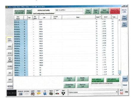
With all port lists defined and ports assigned to lists, save the port file and send the changes to the console. You may overwrite the existing Lists file or save a new Ports List file.
