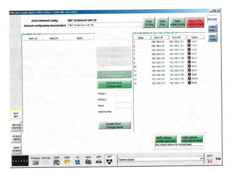
In order to use the new network configuration, which includes your new I/O box, you must first load the new network configuration into the console.
