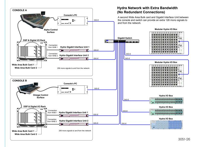
Each WAB and Gigabit interface provides 128 mono audio paths to and from the network. Increasing the number of WAB/Gigabit interfaces will increase the bandwidth your system can support.
