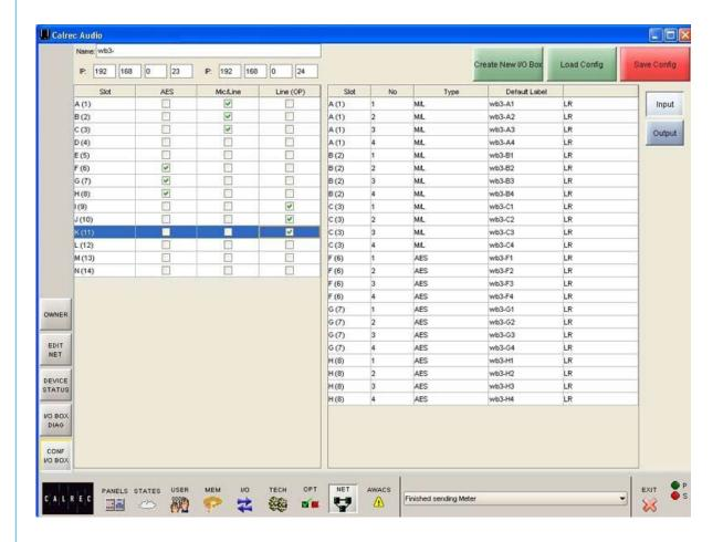
This screen allows the user to manually setup the type of input and output modules occupying each slot in a modular Hydra I/O box.
