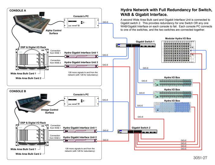
The system can offer redundancy, such that it is protected in case of failure of any connector, cable, or even a Gigabit switch.
