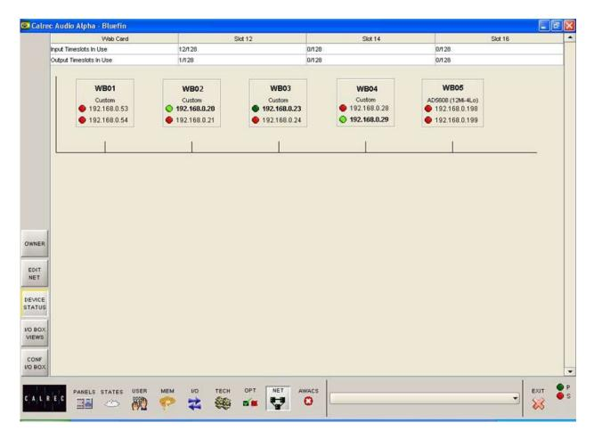
The Device Status screen provides an overview of the status of all devices configured on the network.
