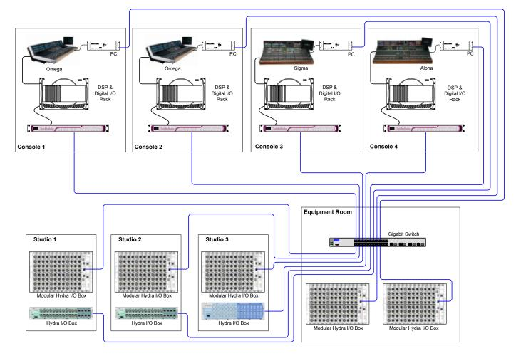
The above diagram shows 4 control rooms, each with a Calrec digital console. The Gigabit interface unit for each console transmits and receives audio data to and from the Hydra I/O boxes, via a Gigabit switch located in the Equipment Room.
