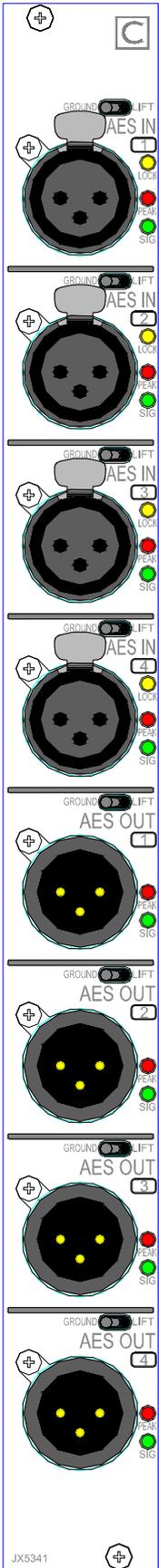
This module provides 4 AES inputs and 4 AES output circuits.
