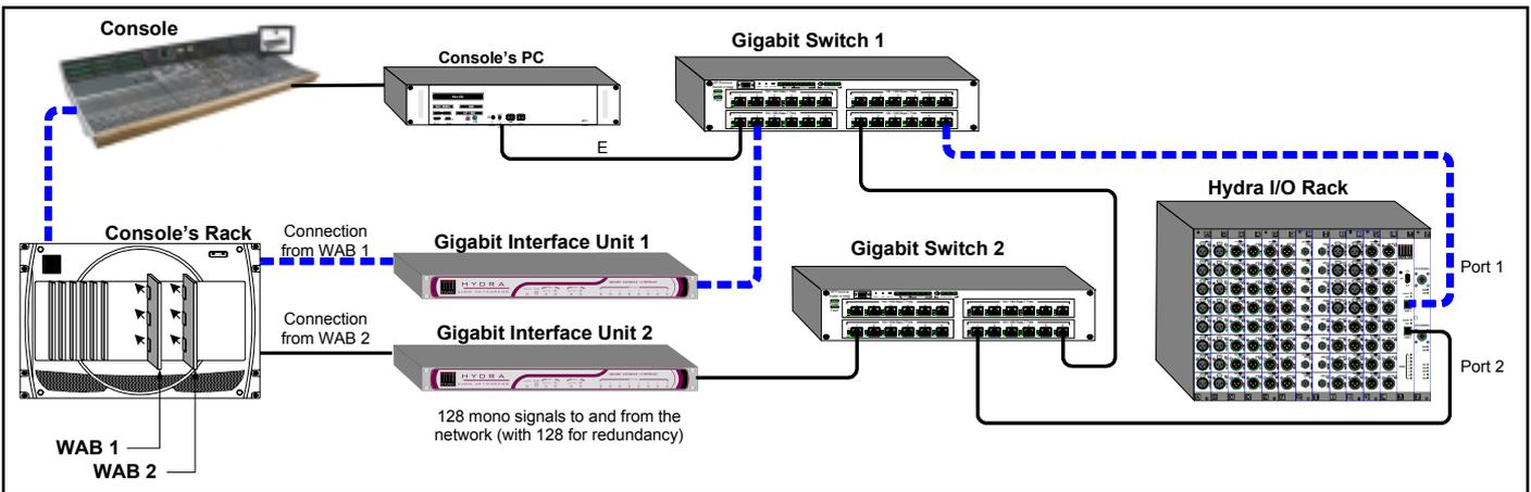
**Example 1 - Loss of Connection between Gigabit Interface 1 and Gigabit Switch 1**
