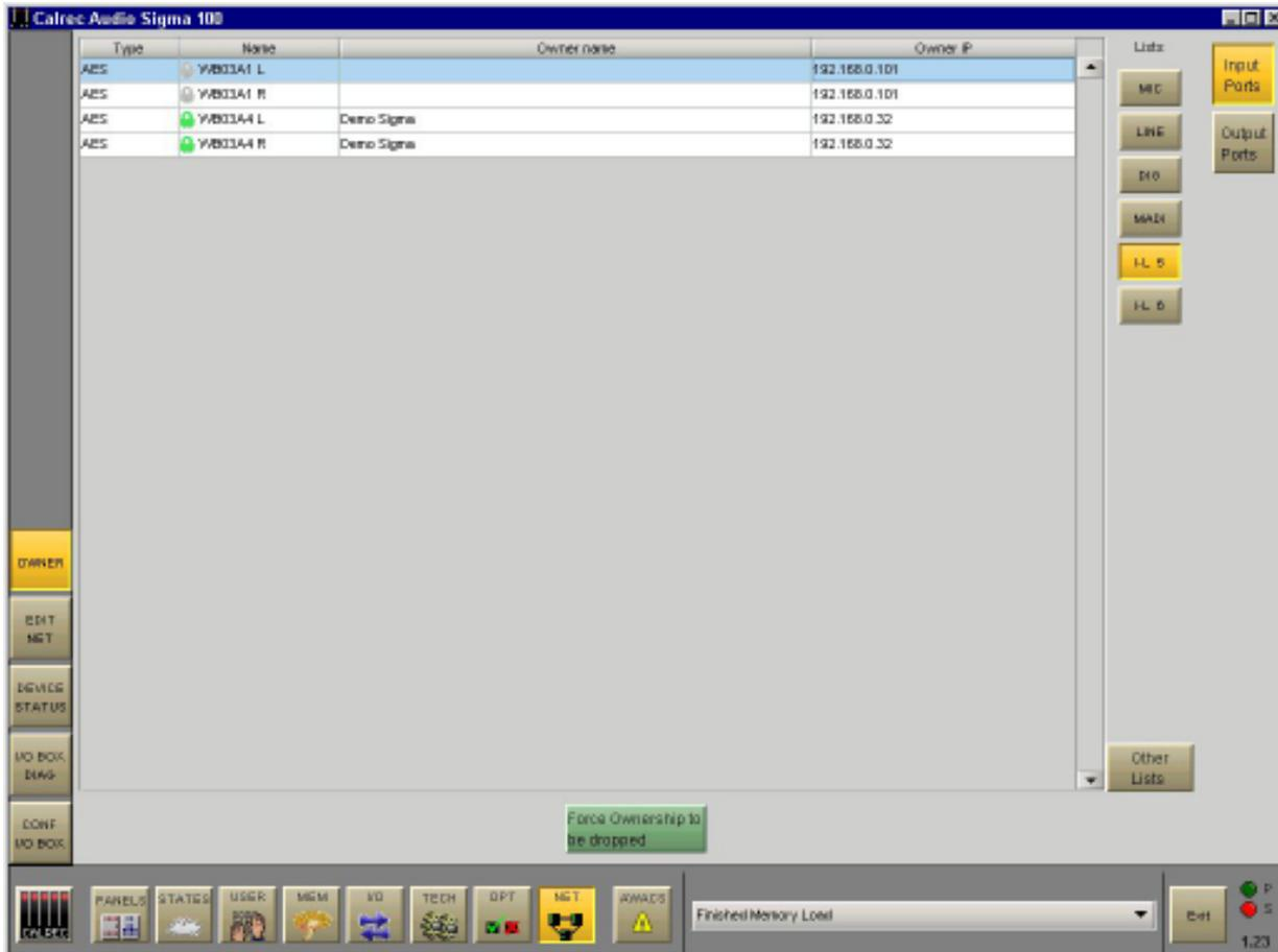
When a Hydra port is patched, ownership of it assigned to the console. The console that connects to the source first will be given control (ownership) over that source. Other consoles that subsequently connect the same source will not be able to control it.
