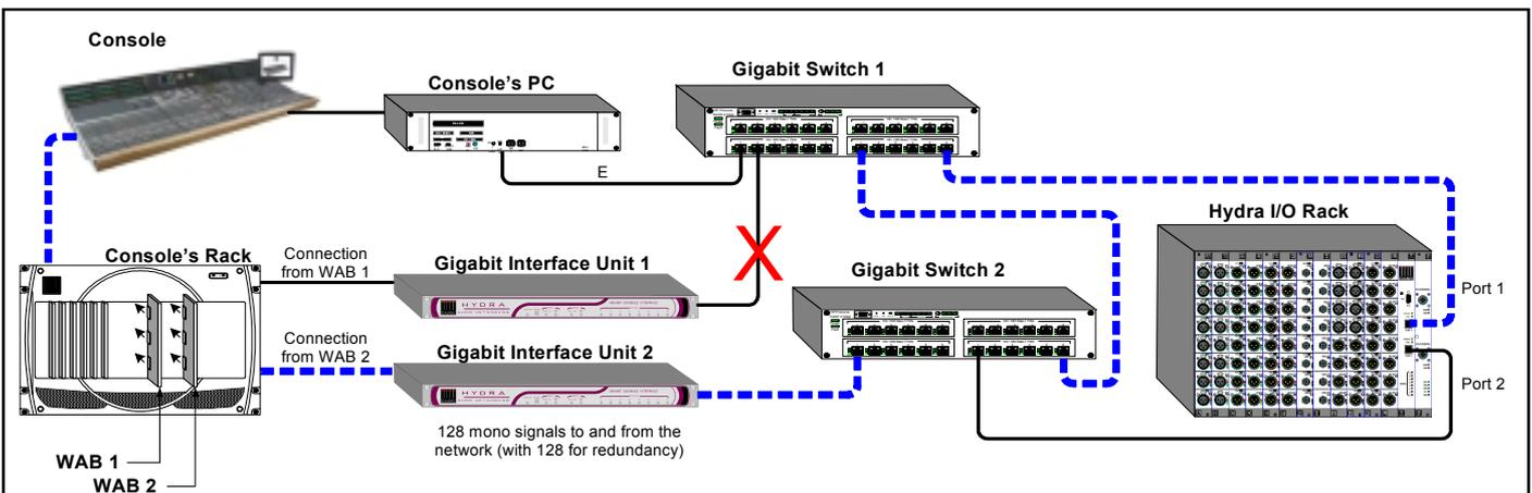
**Example 2 - Loss of Connection to the Hydra I/O Rack Port**
