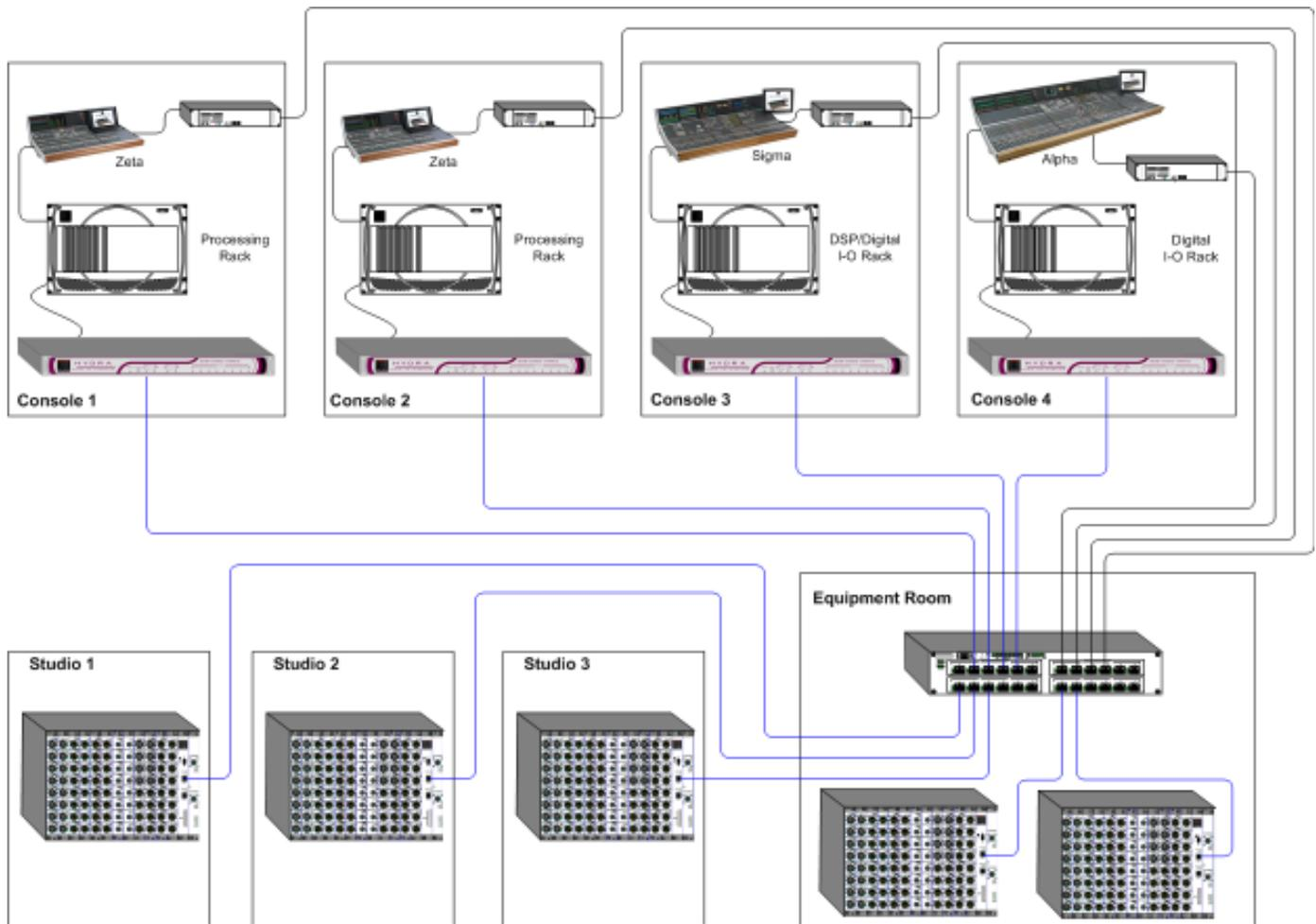
The above diagram shows 4 control rooms, each with a Calrec digital console. The Gigabit interface unit for each console transmits and receives audio data to and from the Hydra I/O Racks, via a Gigabit switch located in the Equipment Room. The console racks and Gigabit interface unit could also be in the Equipment Room if this was more suitable.
