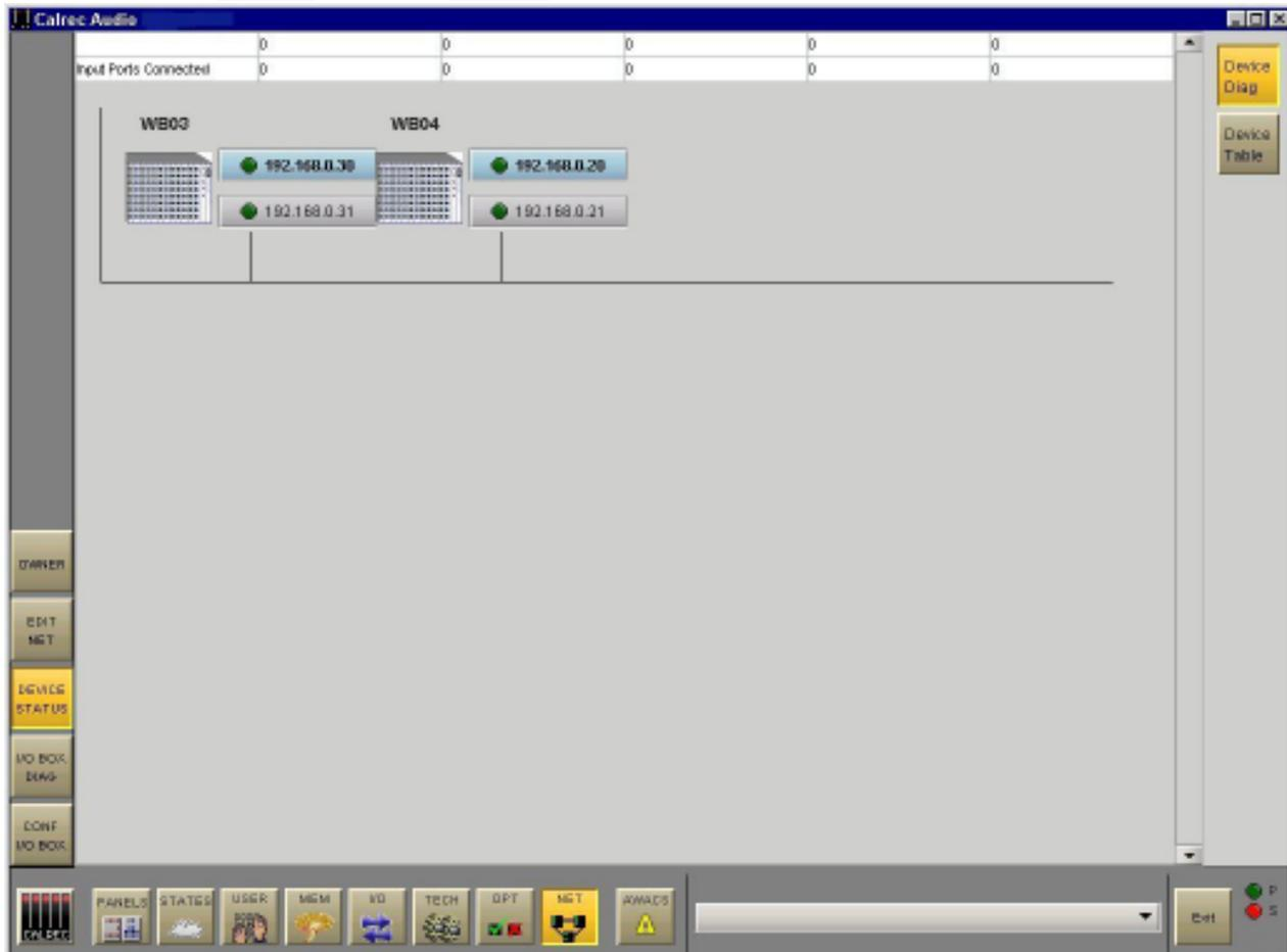
The Device Status screen provides a graphical overview of the status of all devices configured on the network. Each port has a green indicator, which will “heartbeat” (flash bright green) to indicate that the unit is running and can be reached. If the device is not “heartbeating” then it cannot be reached and its graphic will be greyed out.
