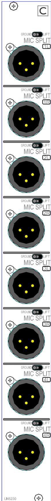
This module provides 8 split outputs which are at the same level as the mic/line input being split. The panel must be situated adjacent to the right hand side of the mic/line input panel that it is splitting. If extra splits are required of the mic/line input more splitter modules can be placed to the right of the first splitter, up to a maximum of 11 splitter units.
