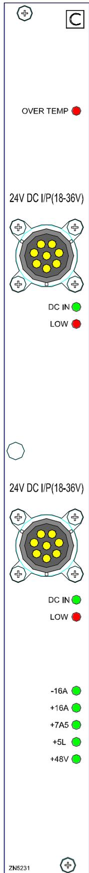
This module is the primary DC power supply for the Hydra I/O Rack. It has two input connectors, which offer partial redundancy. However for full redundancy and greater security, a second DC power supply unit would be fitted into the rack adjacent to the primary DC power supply unit and an input connection wired to each module.
