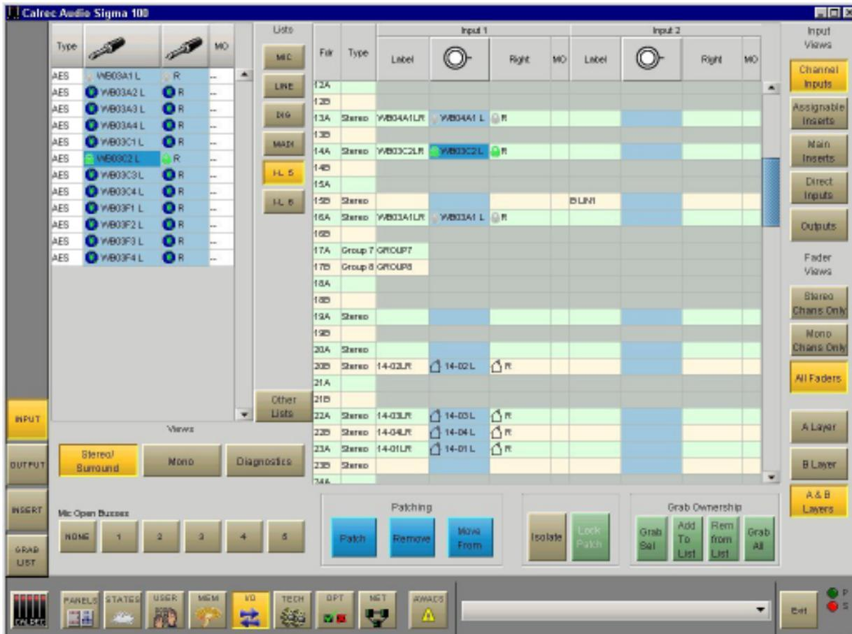
Once set up, Hydra sources are selectable on the I/O screens just like local sources, and can then be patched to faders on the console in the same way. A Hydra I/O list can be selected from the list selector buttons, just like local lists. "Other Lists" is used to access the FE only lists. When selected, the Hydra sources will be displayed on the left side of the screen. These sources can then be patched to faders on the console on the right side of the screen.
