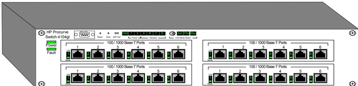
Although the console and racks boot from power on in less than 20 seconds, the switch may take longer, Therefore, networked I/O may take slightly longer to become available on power up, or after a switch reset. It is recommended that the switch is powered using an un-interruptible power supply.
