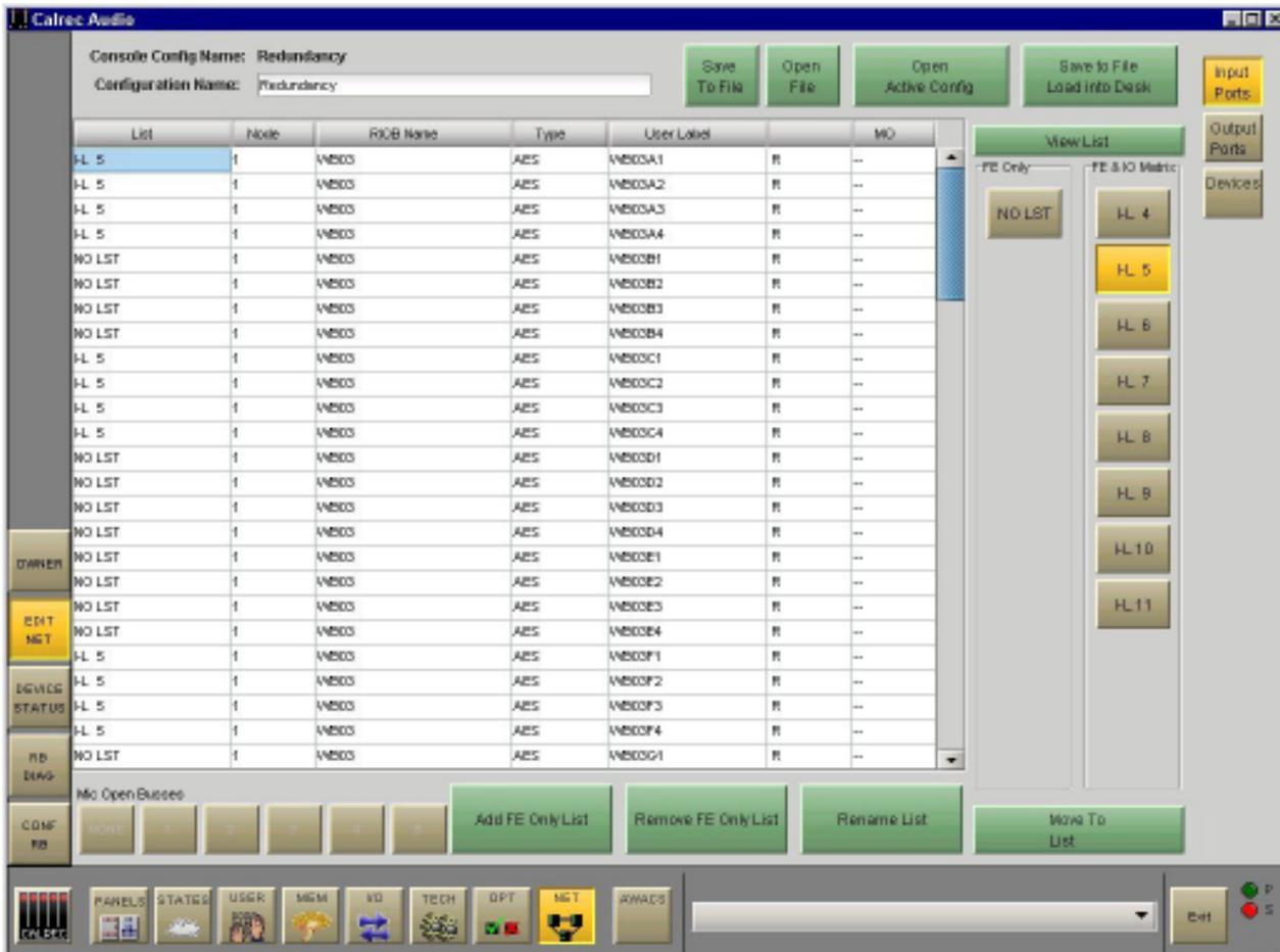
This screen allows the user to allocate the sources from the the Hydra I/O Racks into lists to allow similar I/O to be grouped together for selection. This also makes them easier to access either on the front end (FE) application or on the I/O matrix port assignment controls on the control surface (if available).
