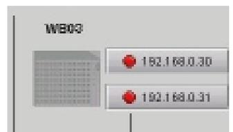
If the device does not appear to be heartbeating, but it is not greyed out, then the console can access the device, but the PC cannot. This situation could arise in redundant systems, where the PC is connected to just one of two switches, and the connection between the switches has failed. The PC will only be able to “see” the devices connected to the same switch as itself. As the console will be connected to both switches, normal operation can continue.
