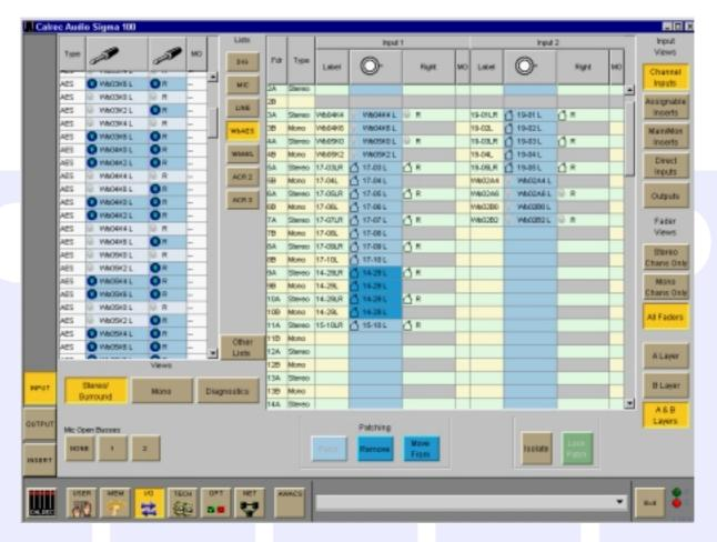
Once set up, remote sources are selectable on the I/O screens just like local sources, and can then be patched to faders on the console in the same way. A Remote I/O unit or console can be selected from the list selector buttons, just like local lists. When selected, the remote sources will be displayed on the left side of the screen. These sources can then be patched to faders on the console on the right side of the screen.
