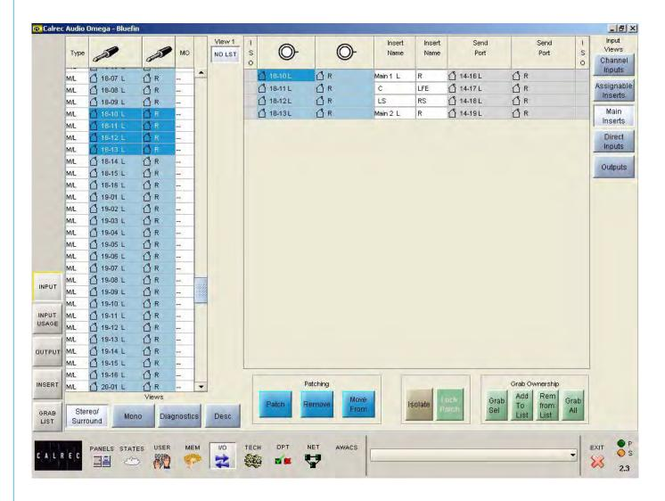
The main insert returns are set up on the I/O - INPUT screen, by selecting "Main Inserts" from the list of Input Views. The input sources for main insert returns can be patched here in the same way that channel inputs are patched.
