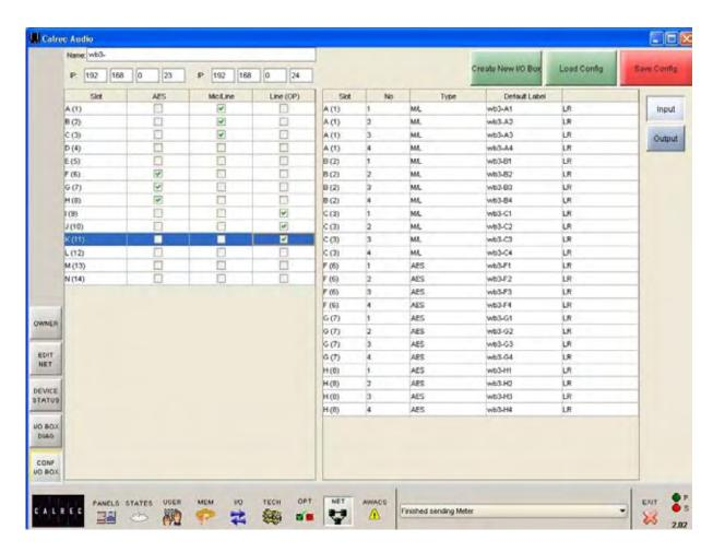
This screen allows the user to manually setup the type of input and output modules occupying each slot in a Hydra I/O Rack. Please note that this configurability is not available for small format I/O boxes.
