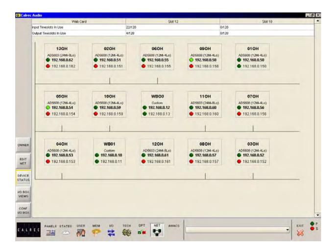
The Device Status screen provides a graphical overview of the status of all devices configured on the network.
