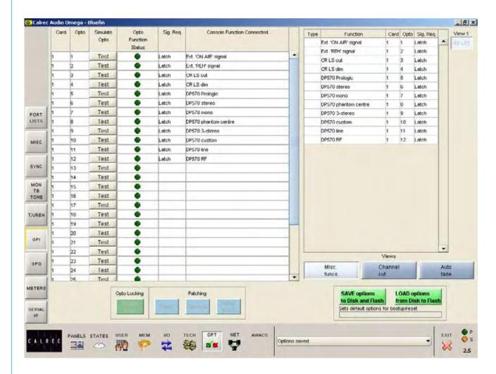
Connections for 32 opto-isolated inputs are provided on the rear of the console. In addition to this, there are 8 double pole change-over GPIO relays on the rear of the Bulk Power Supply and Distribution Unit. The GPI screen allows the general purpose inputs to be set up.
