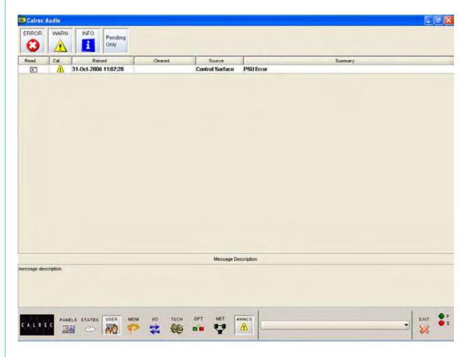
If a problem does develop, messages are delivered on the Automatic Warning and Correction System (AWACS) screen.
