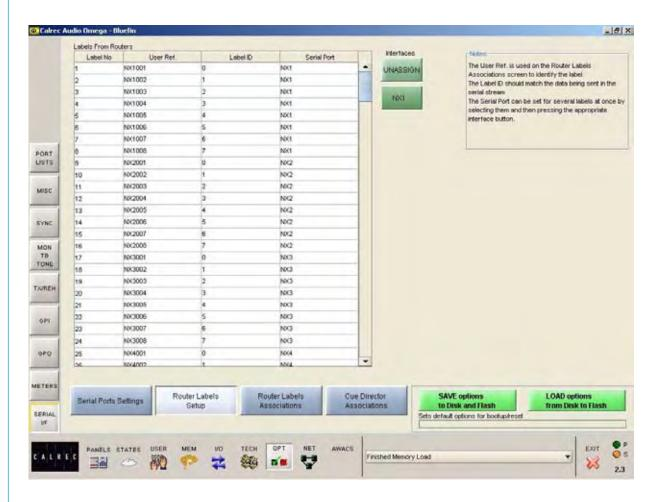
Some Routers incorporate a label interface which is used for the transmission of source (input) and destination (output) descriptions between itself and other equipment.
