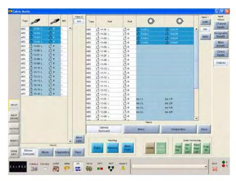
Input ports can be patched directly to output ports on the I/O - INPUT screen, by selecting "Outputs" from the list of Input Views.
