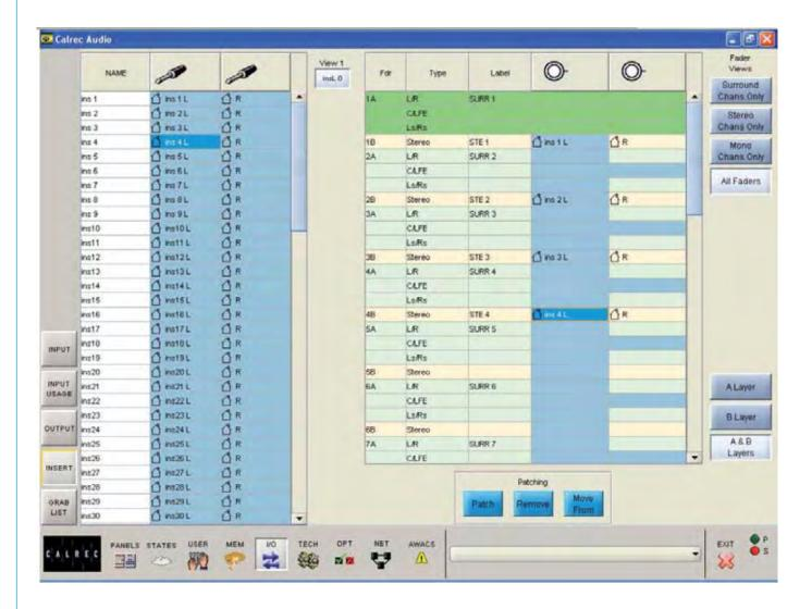
Once the assignable insert sends and returns have been set up on the I/O - Input and I/O - Output screens, they can be patched here to channels and groups, in the same way that channel inputs are patched.
