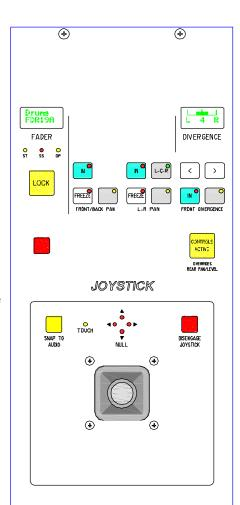
restore any previous Rear Level or Rear Pan controls, but leaves the Rear Level switched out, and the Rear Pan at the same setting and IN/OUT status as the Front Pan.
