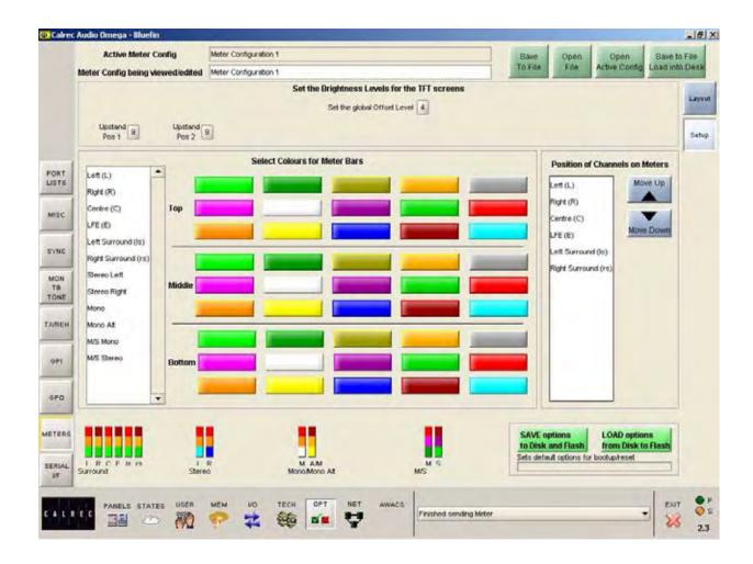
The Options - Meters - Setup screen allows the user to change global metering settings.
