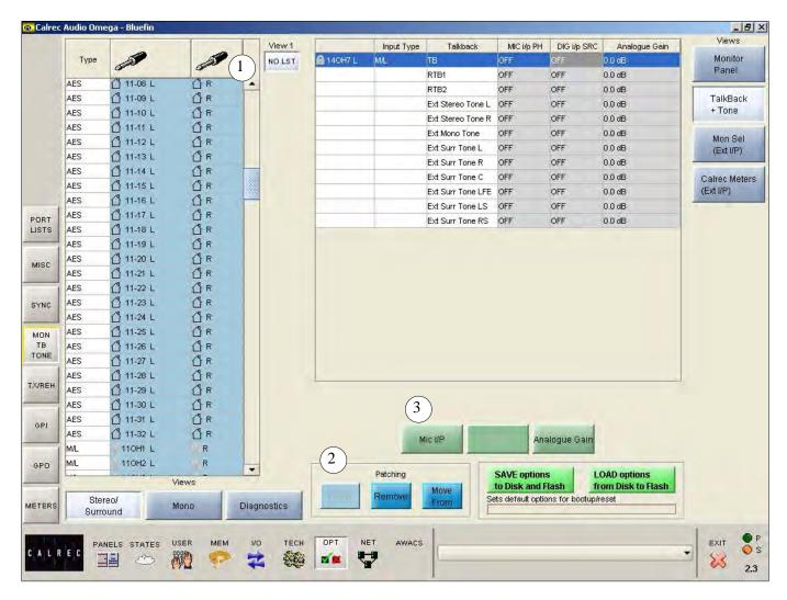
The input sources for Talkback and Reverse Talkback are patched on this screen. The ports for the mono, stereo or 5.1 surround external tone inputs for use with the oscillator can also be patched here.
