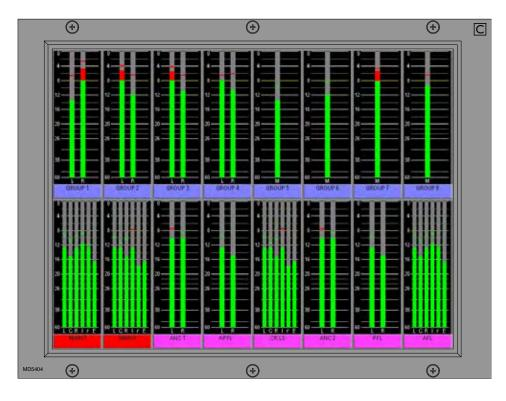
When a screen is configured with 8 columns, these columns will line up with any faders positioned in that section of the console. This is useful when metering channel inputs or groups.
