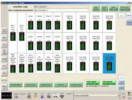
END can be used to allocate subsequent sources in the list to all the meter positions to the right of the selected meter position in the row, until the row is full, or you run out of sources in the list. This is similar to APPLY TO ROW in the pop up dialogue box, COPY TO END allows you to do this after the first meter has had a source allocated.
