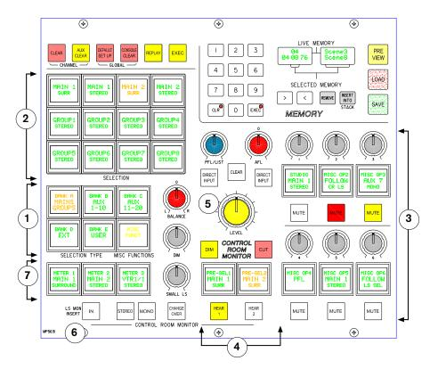
functions bank allows options for the mute button, CUT, DIM and mono/stereo monitoring options to be applied.
