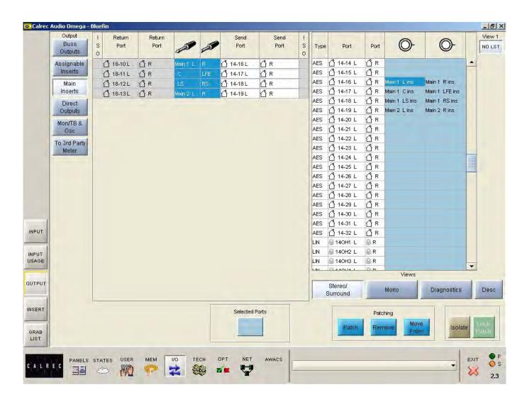
The main insert sends are set up on the I/O - Output screen, by selecting "Main Inserts" from the list of output views. The output ports for main insert sends can be patched, moved and removed here in the same way as buss outputs are patched.
