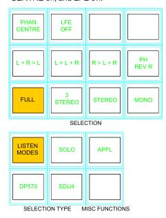
4 stereo option buttons: L+R to L, L to L+R, R to L+R and PH REV R. These will work in any mode, but are really designed for use in stereo mode or when monitoring stereo sources.
