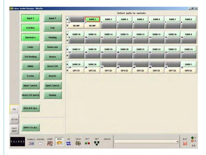
The right side of the screen shows all fader paths. Paths can be selected from here or by pressing the fader assign button.
