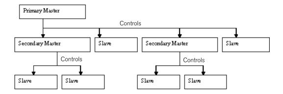
VCA groups allow the audio level, CUT, AFL and PFL functions of several slave faders to be controlled from one master fader.
