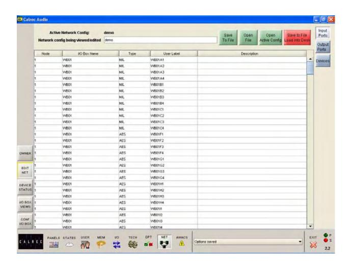
This screen allows the user to view the hydra sources, their location and type. A similar screen is available to view the output ports.
