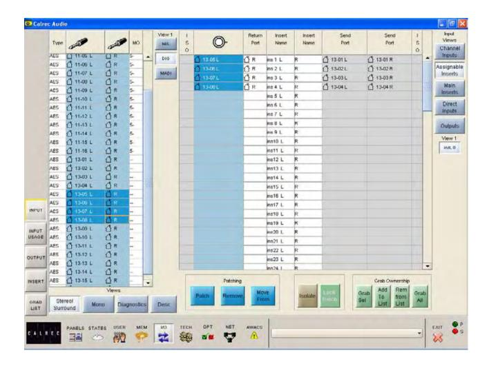
There can be up to 96 pairs of assignable inserts for use in channel or group paths. Input ports for the assignable insert returns are set up on the I/O - Input screen, by selecting "Assignable Inserts" from the list of Input Views.
