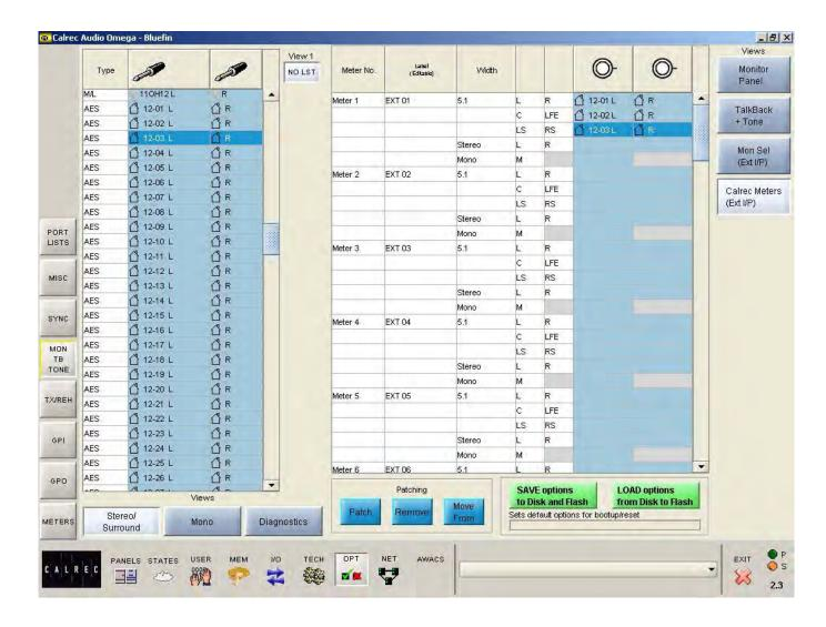
The input sources for external meters can be patched here in the same way that channel inputs are patched. There can be up to 32 external meter inputs, which are mono, stereo or 5.1 surround.
