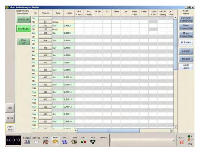
The partial memory save option allows components of console settings to be saved in the same way as full console memories. Once partial memory save option is active, the save buttons on the screen and control surface are used to save partial memories in the same way as full console memories.
