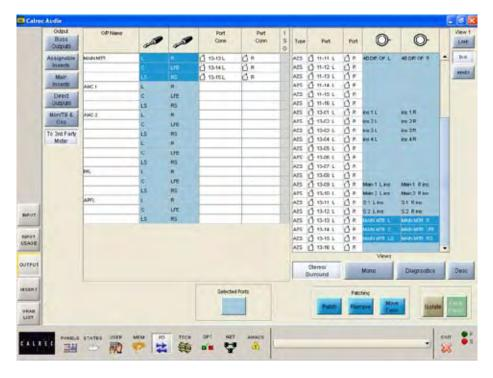
The output ports for external meters, such as a DK phase scope, can be patched on the I/O - OUTPUT screen, by selecting "To 3rd Party Meter" from the list of Output Views. Most of the meters on the console are driven internally and do not require output ports.
