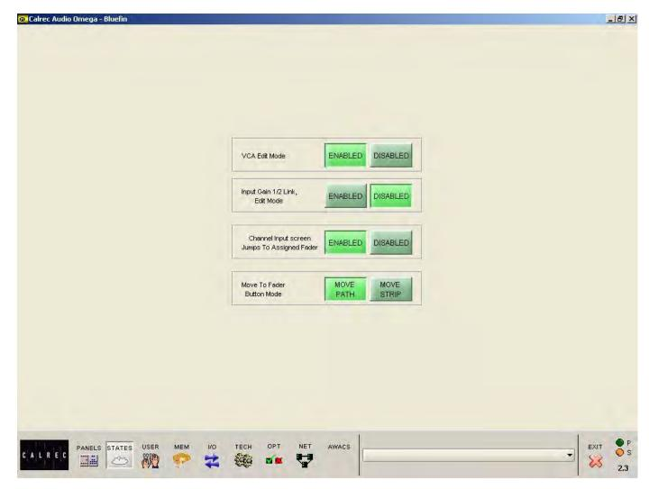
The States Screen allows different console behaviours to be enabled and disabled.
