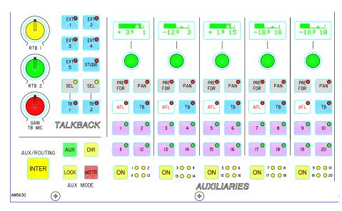
When DIRECT or MASTER are selected, the displays above each rotary control show a bargraph of the gain, and what is being controlled (e.g O/P or DIR). This remains until they are adjusted, when the dB value of the gain is then displayed. A short time after the adjustment has been made, the display will show the bar and label again.
