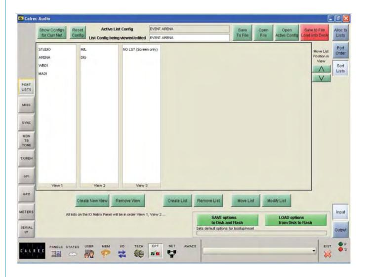
This screen allows a number of list views to be created. List views allow the user to change the order the lists appear on the port selection controls and I/O patching screens, and control the accessibility of the lists.
