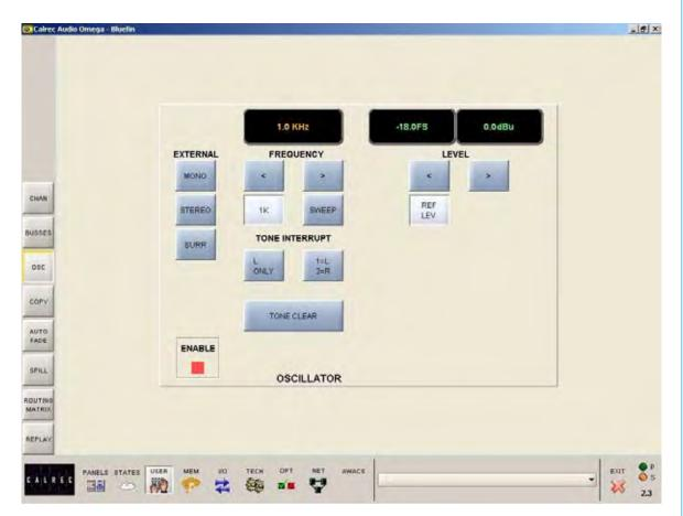
This screen provides controls for the oscillator, which is used to generate test tones for alignment and testing.
