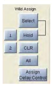
All the Assign panel rotary controls incorporate a switch which is operated by pushing the control. These switches are used to assign the assign panel function to a Wild control as follows:
