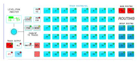
can be added or removed from the bus under interrogation, by selecting or deselecting their fader assign buttons.
