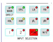
SRC switches the sample rate converter on AES inputs.
