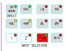
Go to the **Port Select** area of the control surface and select Input 1 or 2 in order to assign a port to it. Do this by turning the selector control knob to scroll through the available ports.
