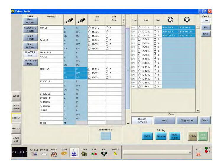
The output ports for the monitoring, talkback and oscillator outputs can be patched on the I/O - OUTPUT screen, by selecting "Mon/TB & Osc" from the list of Output Views.
