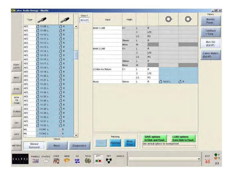
The input sources for external monitor inputs can be patched here in the same way that channel inputs are patched.
