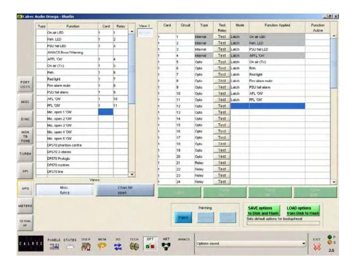
Connections for 16 opto outputs and 40 Darlington outputs are provided on the rear of the console. In addition to this, there are 8 double pole change-over GPIO relays on the rear of the Bulk Power Supply and Distribution Unit. The GPO screen allows the general purpose outputs to be set up.
