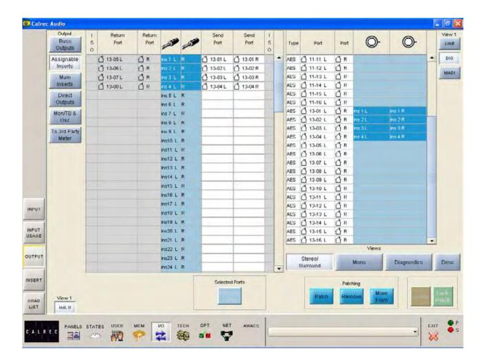
There can be up to 96 pairs of assignable inserts for use in channel or group paths. Output ports for the assignable insert sends are set up on the I/O - Output screen, by selecting "Assignable Inserts" from the list of Output Views.
