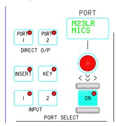
Once you have arrived at the port you want, press the ON button to connect it. (this is like inserting the patch cord).
