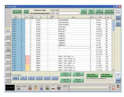
means that the list will not be available for selection on the control surface port selection controls. This makes control surface port selection easier, as it ensures only the relevant lists are displayed. All lists are always available on the I/O patching screens.
