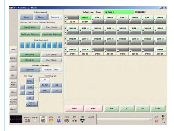
This screen provides controls for channel functions, some of which are available on the control surface. The right side of the screen shows the fader paths A and B.
