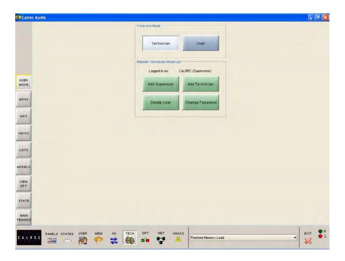
The console can be in one of three modes, "User", "Technician" and "Supervisor". Operation of certain screen functions is only available in "Technician" or "Supervisor" mode. These modes are password protected to add an extra layer of security. The TECH-USER MODE screen is used to log in and out of different modes, and manage usernames and passwords for the different types of user.
