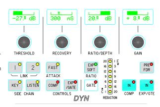
for when the same dynamics settings need to be applied to more than one channel. With the channel selected, press Link 1 or 2 to assign the channel to the bus.
